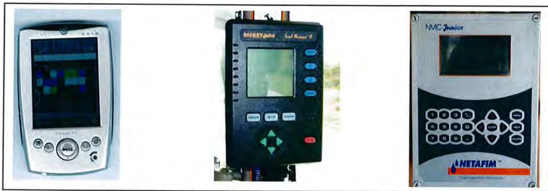
Figure 3. Examples from left to right of a hand-held Pocket PC with Arcpad GIS software (ESRI), variable rate controller for a fertilizer spreader, and an automatic irrigation system controller.
