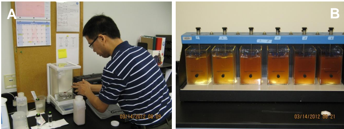
Figure 2. (A) Weighing of ViroPhos™ doses at the start of the jar test; (B) Laboratory mixer used to conduct the jar test with duplicate jars for the (L-R) 0.5, 1.0 and 2.0 ViroPhos™ treatments.
