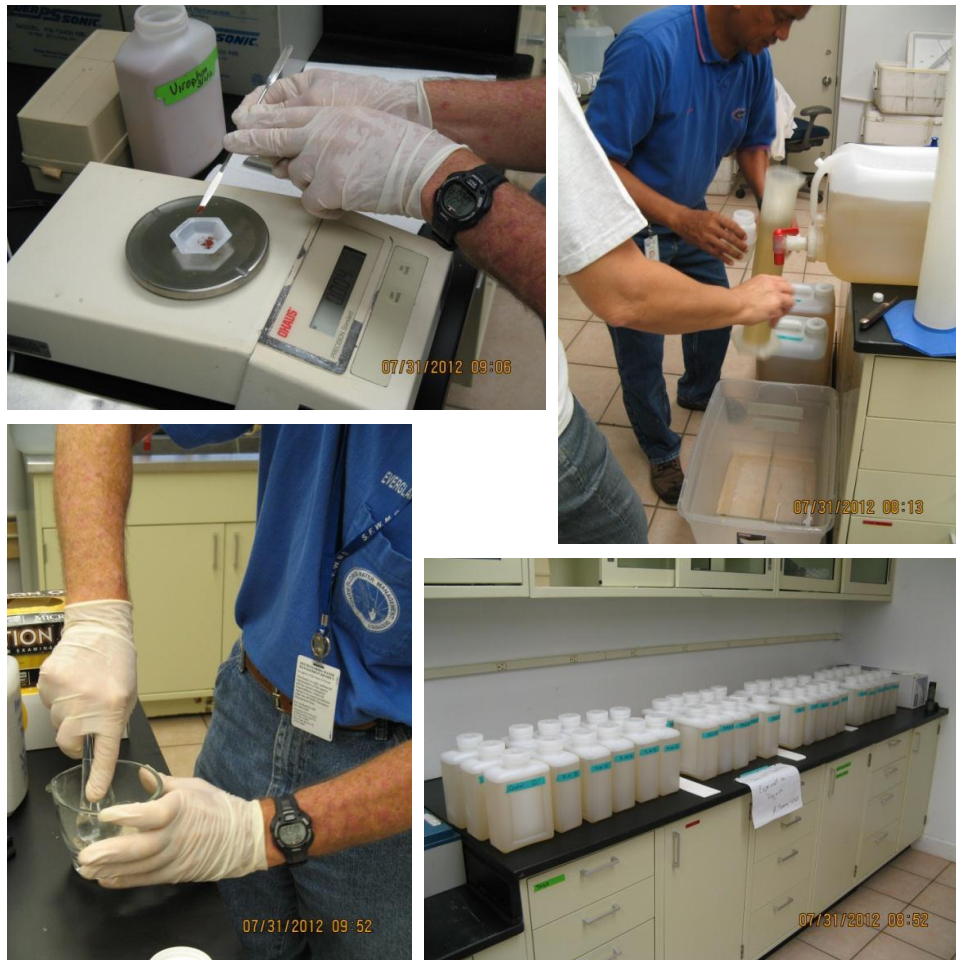
Figure 2. Conducting the NATA Product Jar Test (clockwise from upper left): weighing out a product dose; filling jars with C-51 canal water; arrangement of 2-L Nalgene sample bottles at the start of the test; and grinding Phoslock® with a mortar and pestle.
