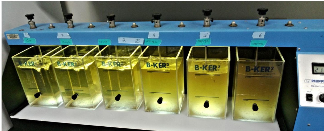
Figure 2. Phipps and Bird PB-700 ™ Standard JarTester apparatus used to conduct the Nclear ® jar test.
