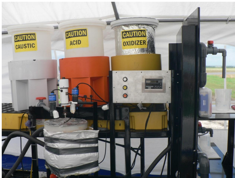
Figure 2. Ferrator® reactor used to synthesize ferrate on site.
