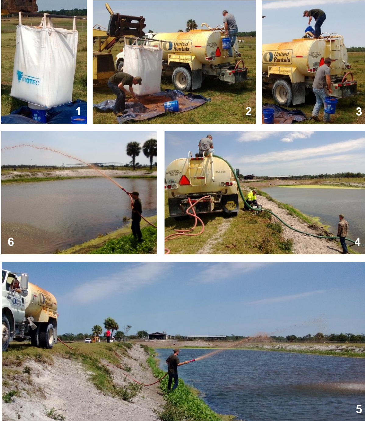
Figure 3. Application of ViroPhos™ at the Turnpike Dairy test pond on March 26-28, 2013. Clockwise from upper left: (1) ViroPhos™ was delivered to the site in supersacs that each held one metric ton of product; (2 & 3) ViroPhos™ was released from a chute at the bottom of the supersac, transferred to 5-gal buckets and loaded into a water tanker truck; (4) the tanker truck was filled with water pumped from the test pond; and (5 & 6) ViroPhos™ was pumped from the tanker truck and sprayed as a slurry onto the surface of the test pond.
