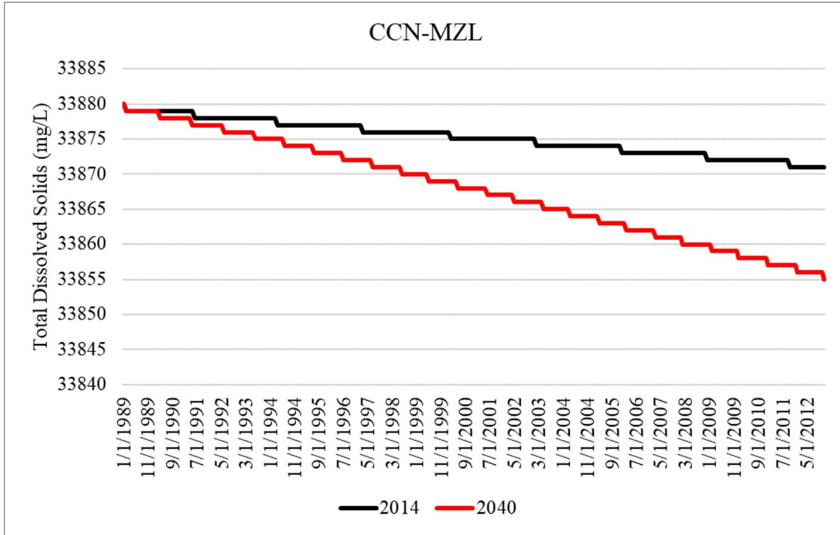
Figure B-25. Simulated total dissolved solids concentrations within the Avon Park permeable zone for the 2014 and 2040 model runs at CCN-MZL in Collier County.
