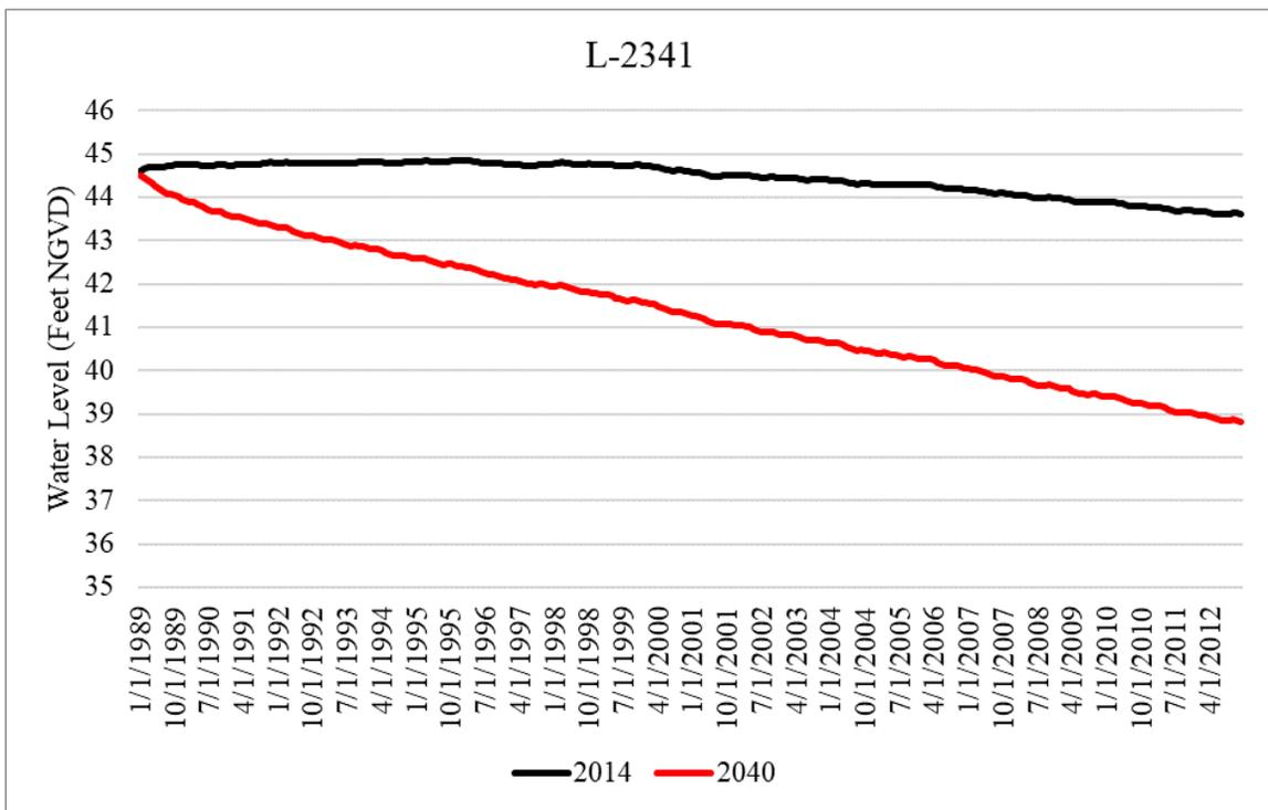
Figure A-8. Simulated water levels within the Upper Floridan aquifer for the 2014 and 2040 model runs at L-2341 in Lee County.
