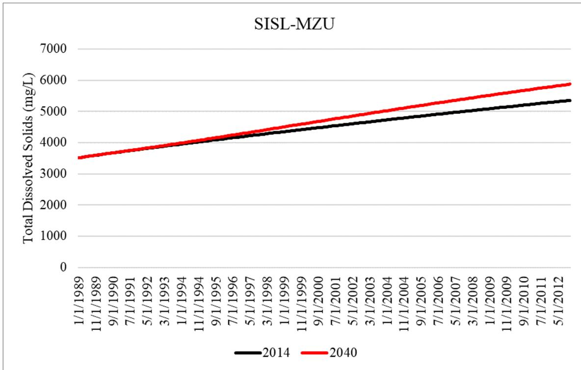
Figure B-16. Simulated total dissolved solids concentrations within the Upper Floridan aquifer for the 2014 and 2040 model runs at SISL-MZU in Lee County.
