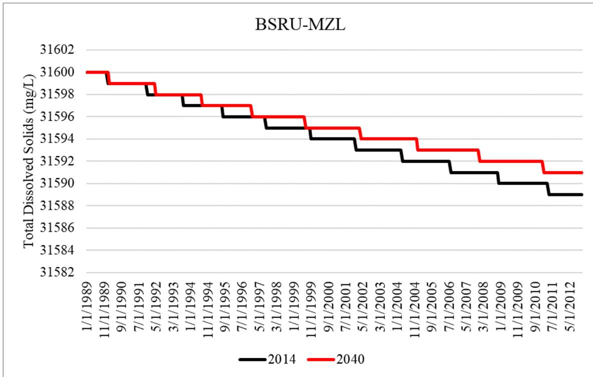
Figure B-4. Simulated total dissolved solids concentrations within the Avon Park permeable zone for the 2014 and 2040 model runs at BSRU-MZL in Lee County.
