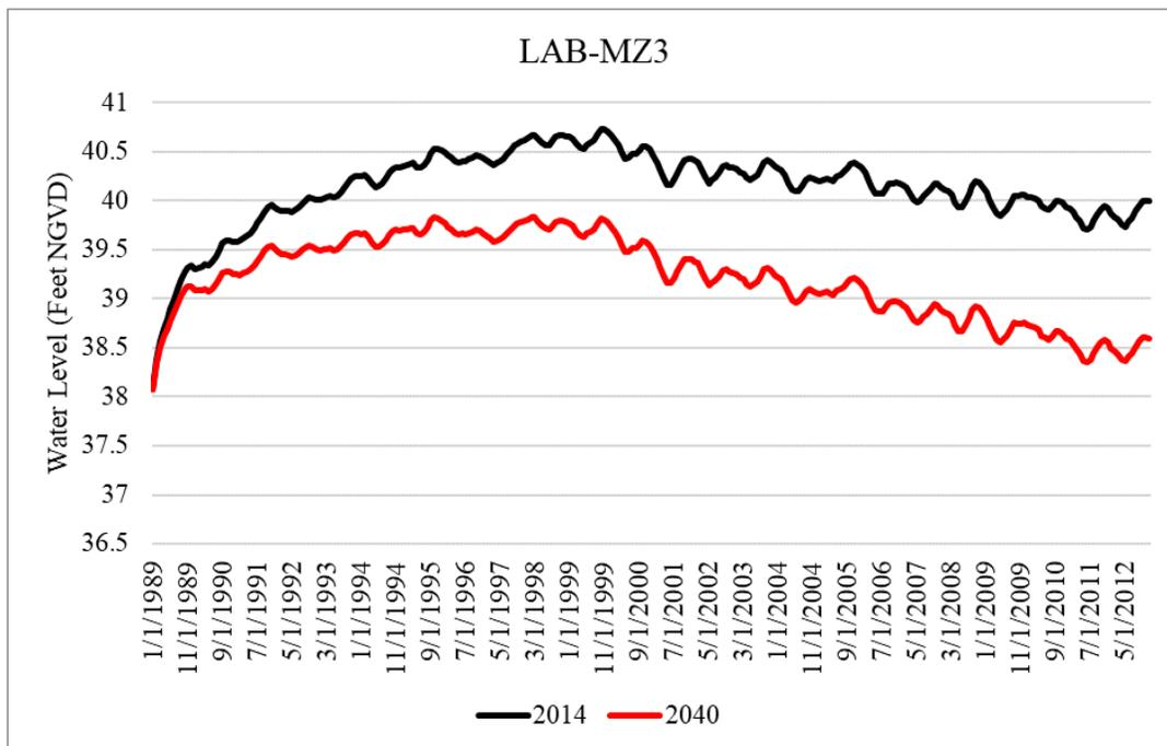
Figure A-12. Simulated water levels within the Avon Park permeable zone for the 2014 and 2040 model runs at LAB-MZ3 in Hendry County.
