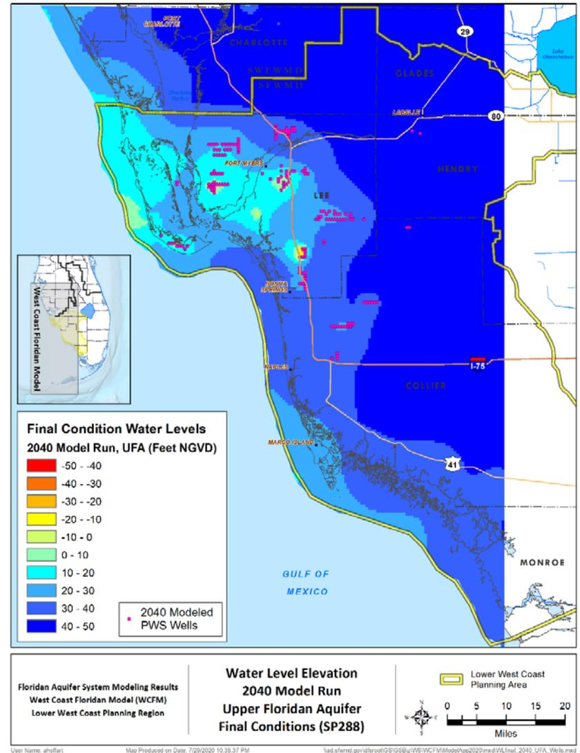
Figure 13. Upper Floridan aquifer water levels for the final condition of the 2040 model run.
