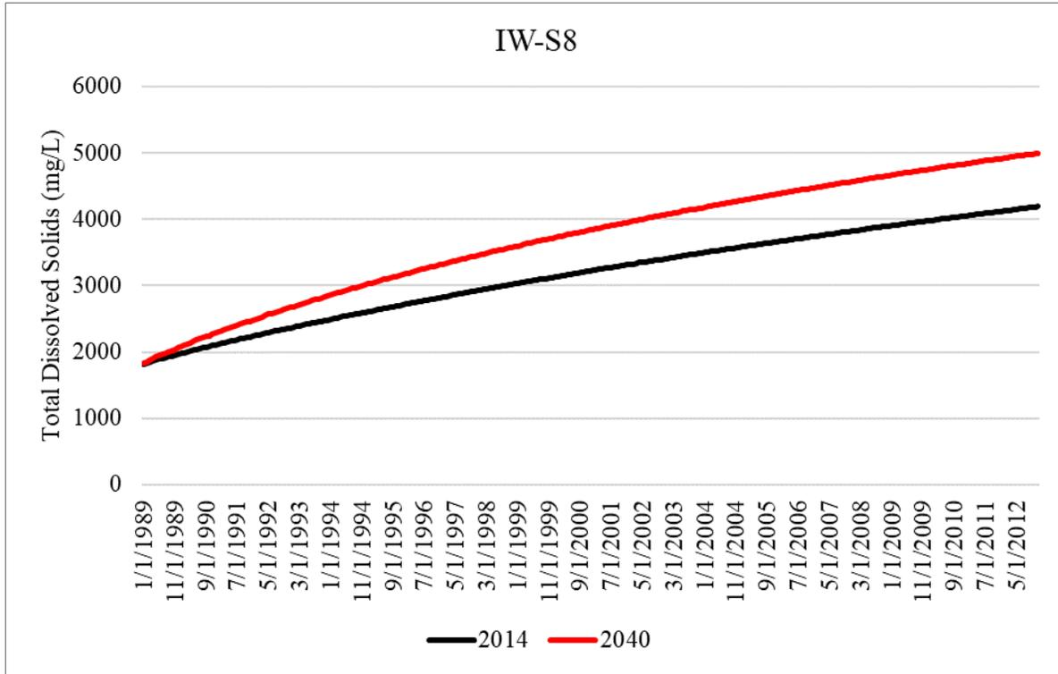
Figure B-15. Simulated total dissolved solids concentrations within the Upper Floridan aquifer for the 2014 and 2040 model runs at IW-S8 in Lee County.
