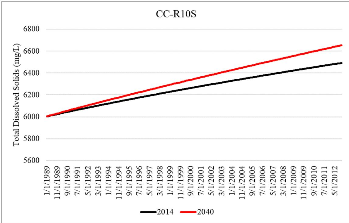
Figure B-27. Simulated total dissolved solids concentrations within the Upper Floridan aquifer for the 2014 and 2040 model runs at CC-R10S in Collier County.
