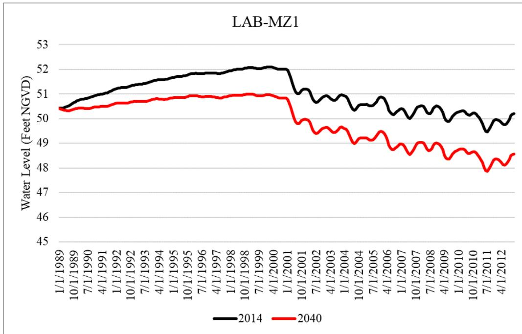
Figure A-11. Simulated water levels within the Upper Floridan aquifer for the 2014 and 2040 model runs at LAB-MZ1 in Hendry County.
