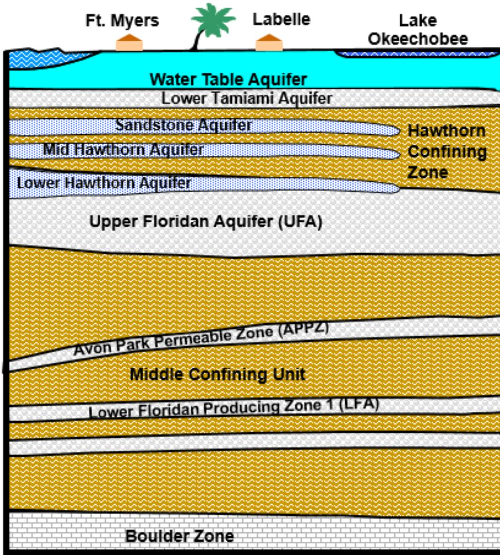
Figure 3. Geologic cross-section through the model domain.
