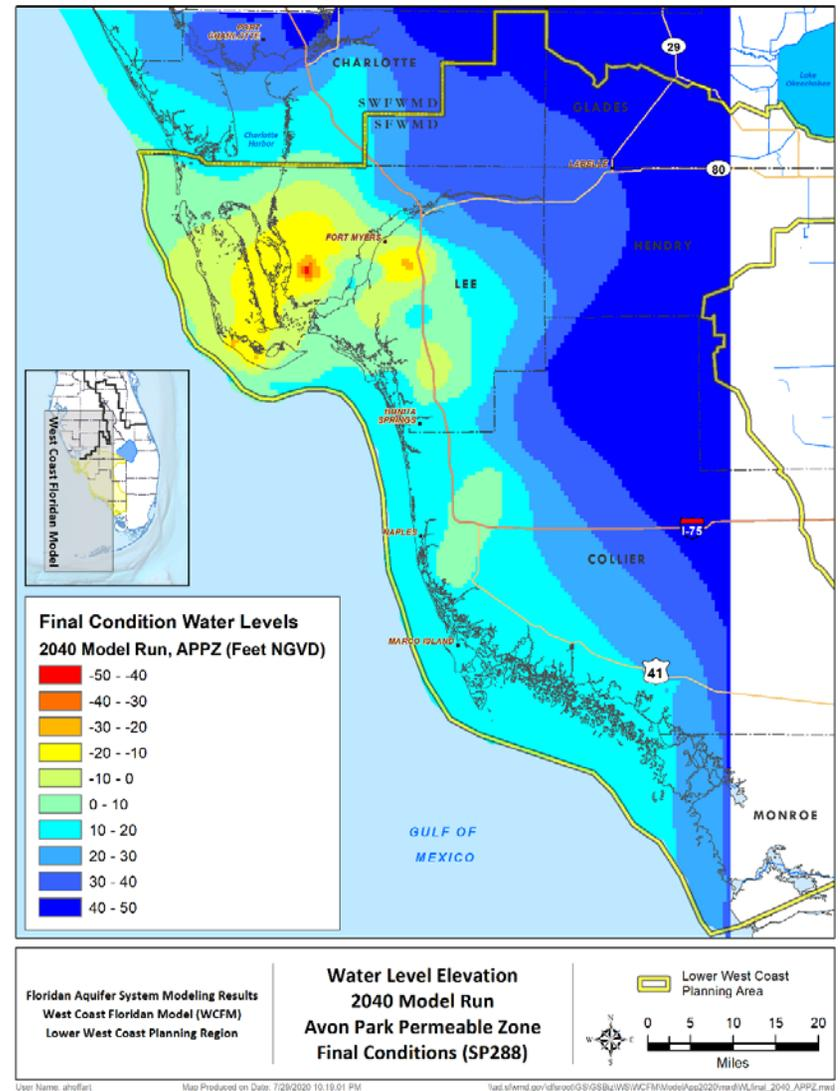
Figure 16. Avon Park permeable zone water levels for the final condition of the 2040 model run.
