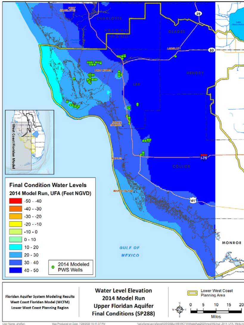
Figure 12. Upper Floridan aquifer water levels for the final condition of the 2014 model run.
