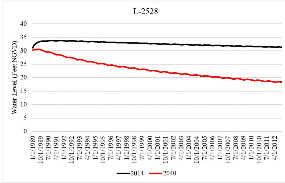
Figure A-1. Simulated water levels within the Upper Floridan aquifer for the 2014 and 2040 model runs at L-2528 in Lee County.
