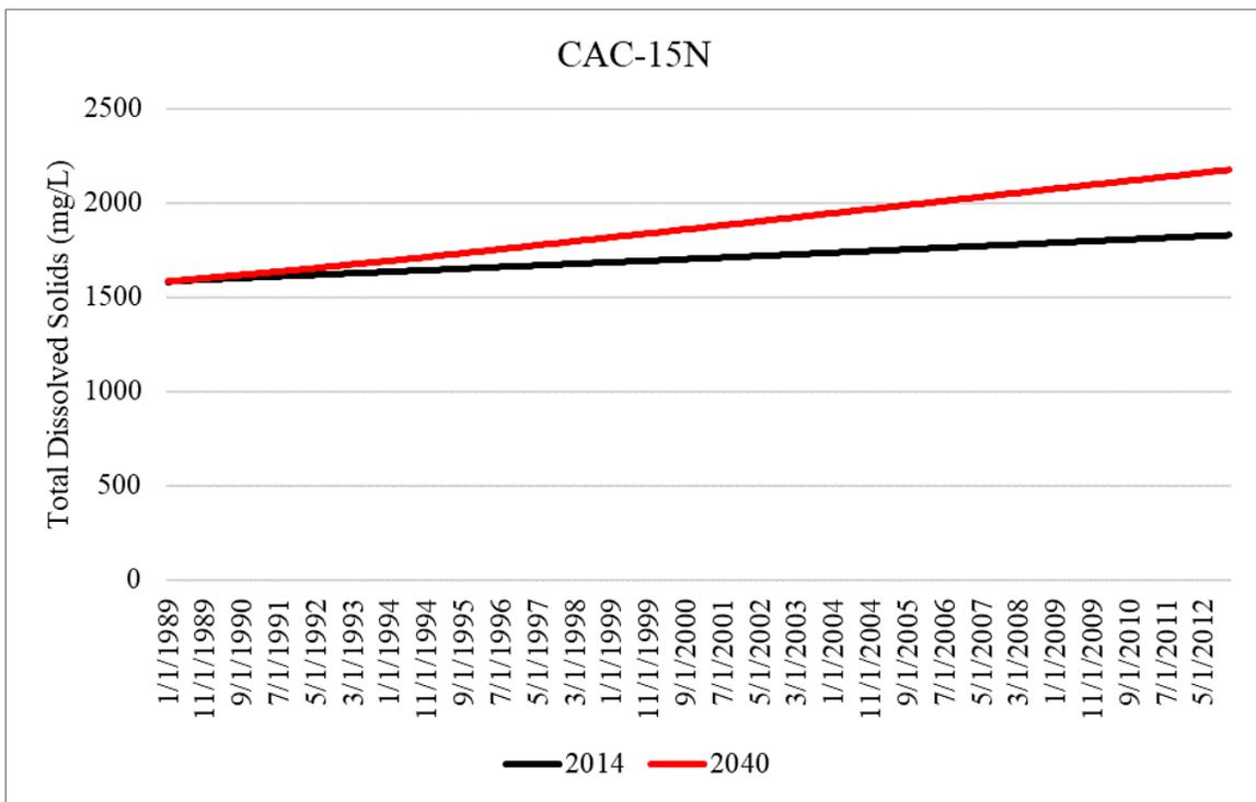
Figure B-6. Simulated total dissolved solids concentrations within the Upper Floridan aquifer for the 2014 and 2040 model runs at CAC-15N in Lee County.
