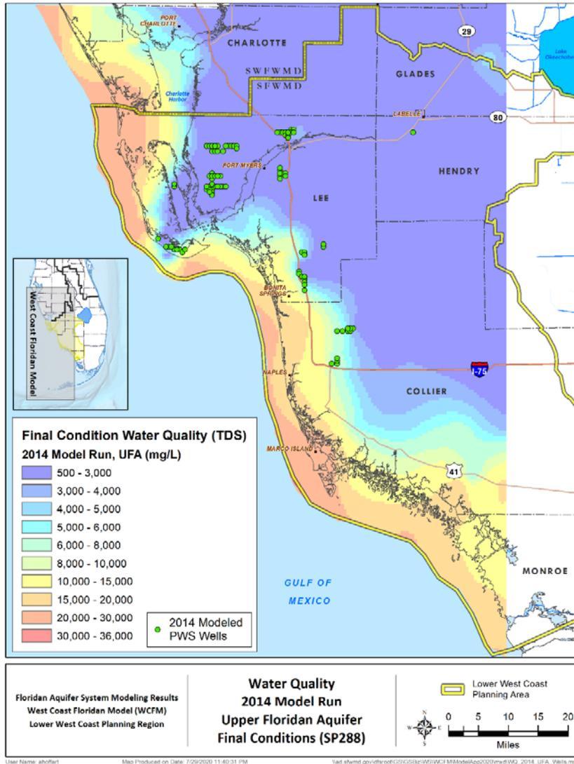
Figure 18. Upper Floridan aquifer water quality (total dissolved solids concentrations) for the final condition of the 2014 model run.
