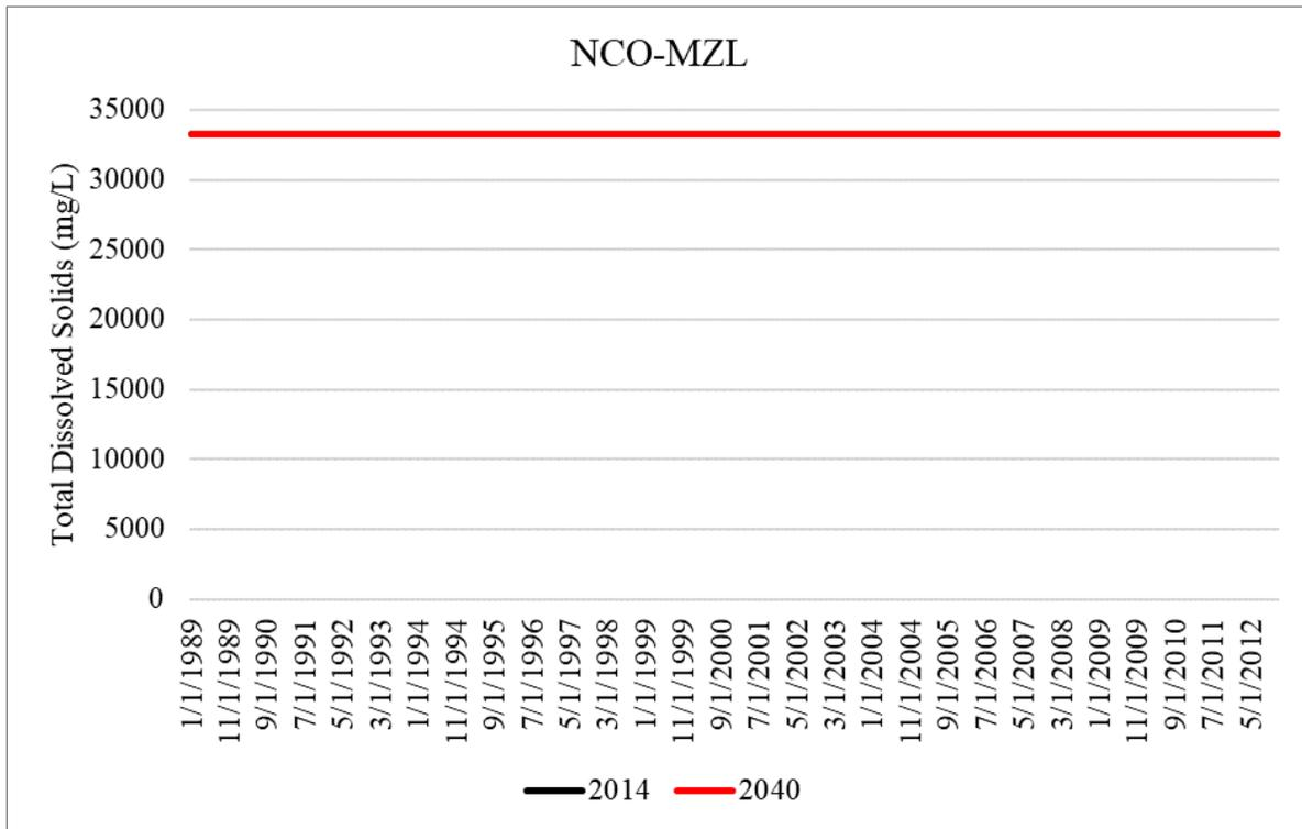
Figure B-26. Simulated total dissolved solids concentrations within the Avon Park permeable zone for the 2014 and 2040 model runs at NCO-MZL in Collier County.
