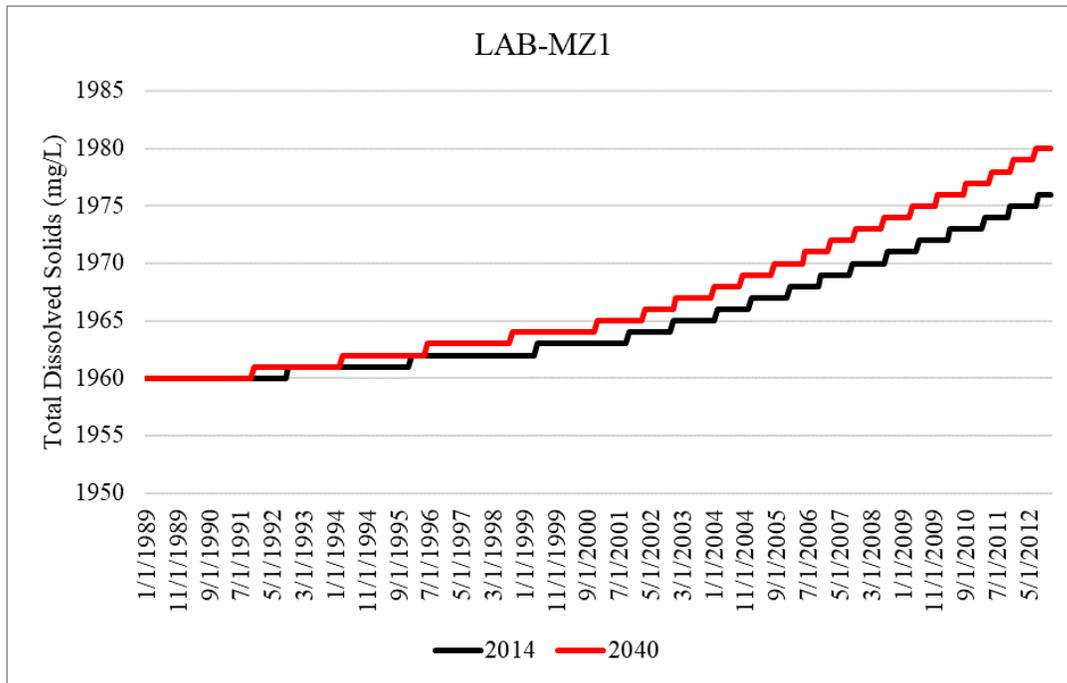
Figure B-33. Simulated total dissolved solids concentrations within the Upper Floridan aquifer for the 2014 and 2040 model runs at LAB-MZ1 in Hendry County.
