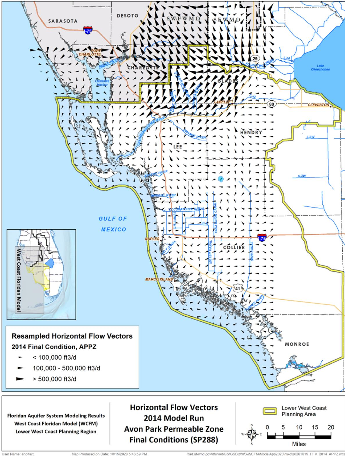
Figure 26. Resampled horizontal flow vectors for the final condition of the 2014 model simulation in the Avon Park permeable zone.
