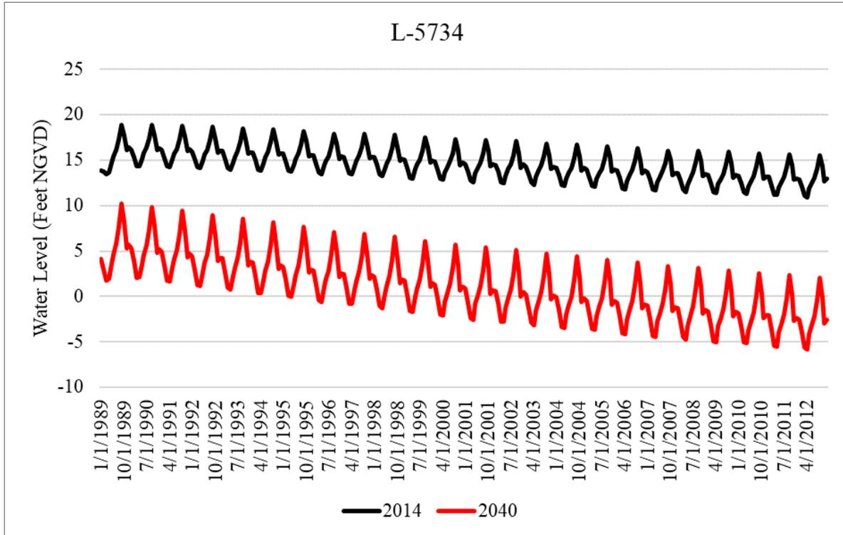
Figure A-5. Simulated water levels within the Upper Floridan aquifer for the 2014 and 2040 model runs at L-5734 in Lee County.
