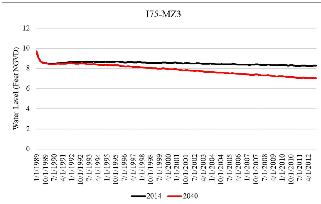
Figure A-10. Simulated water levels within the Lower Floridan aquifer – first permeable zone for the 2014 and 2040 model runs at I75-MZ3 in Collier County.
