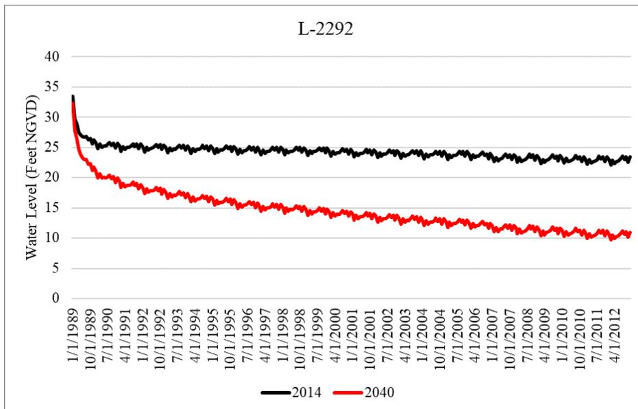
Figure A-2. Simulated water levels within the Upper Floridan aquifer for the 2014 and 2040 model runs at L-2292 in Lee County.
