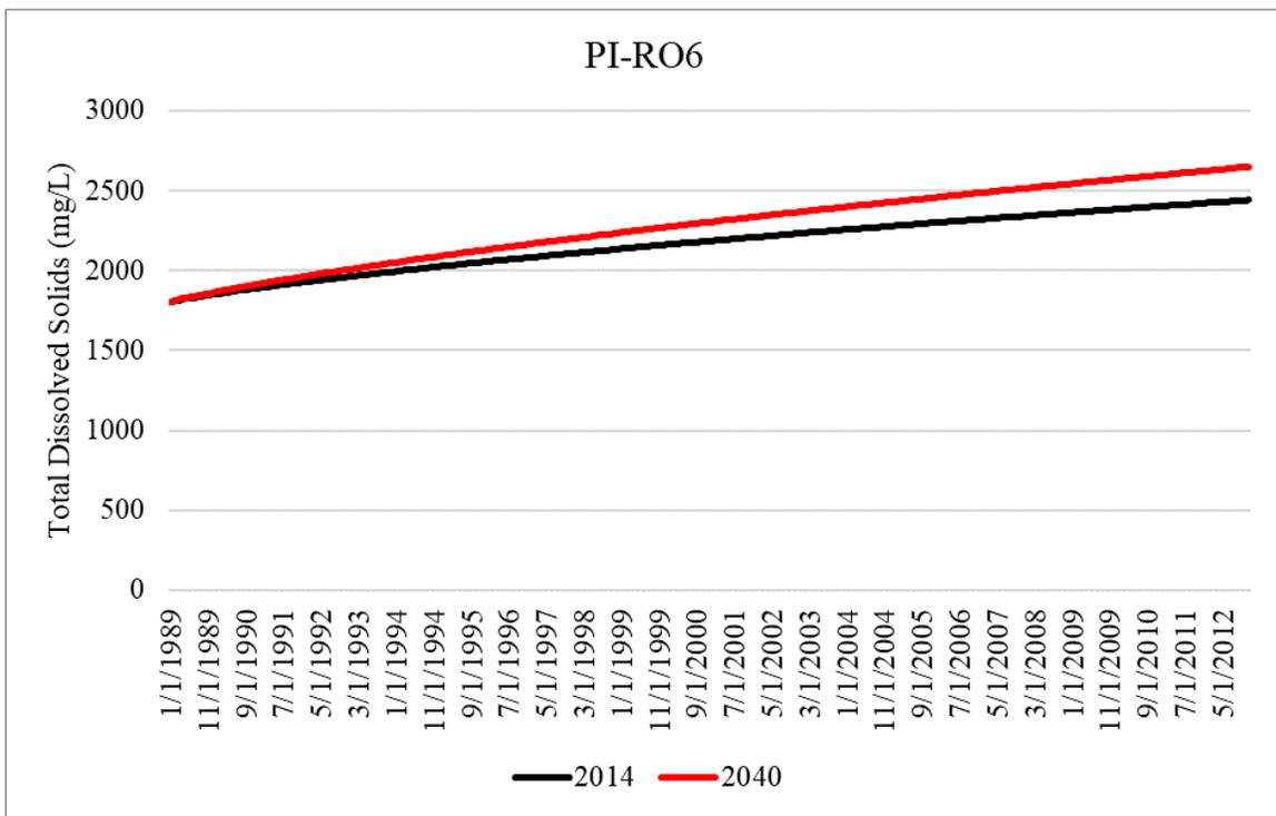
Figure B-12. Simulated total dissolved solids concentrations within the Upper Floridan aquifer for the 2014 and 2040 model runs at PI-RO6 in Lee County.
