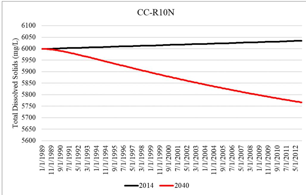
Figure B-21. Simulated total dissolved solids concentrations within the Upper Floridan aquifer for the 2014 and 2040 model runs at CC-R10N in Collier County.
