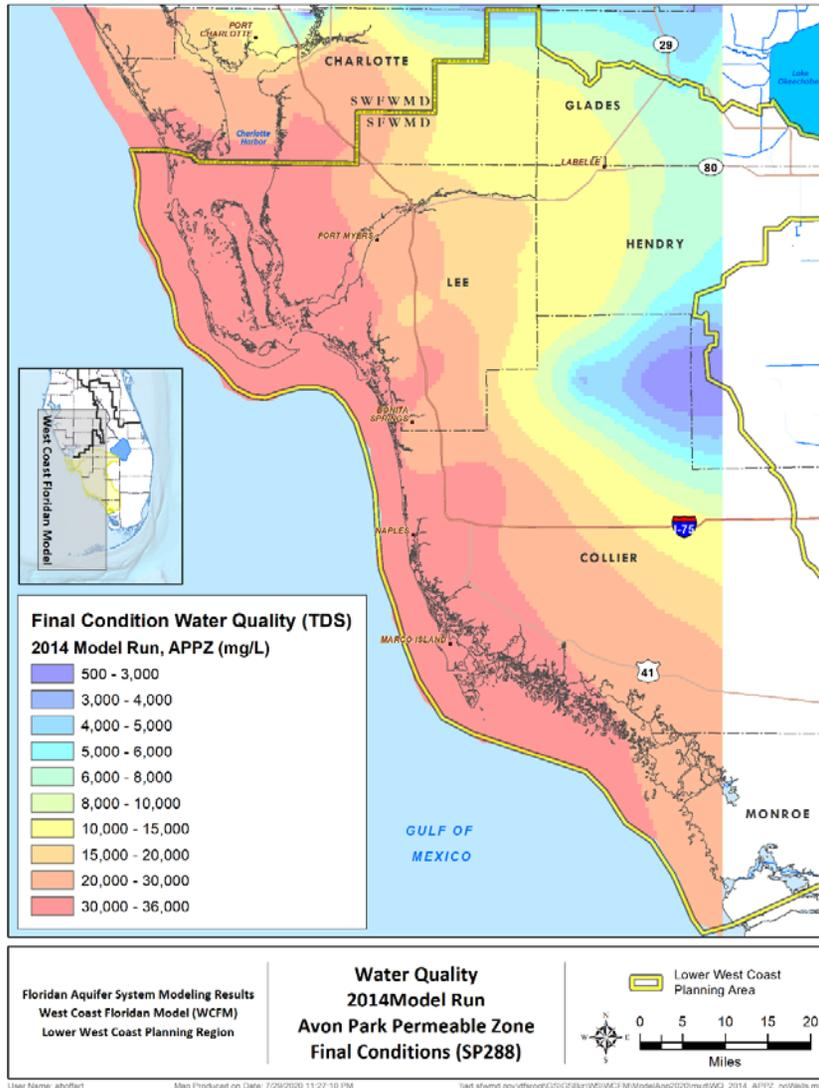
Figure 21. Avon Park permeable zone water quality (total dissolved solids concentrations) for the final condition of the 2014 model run.
