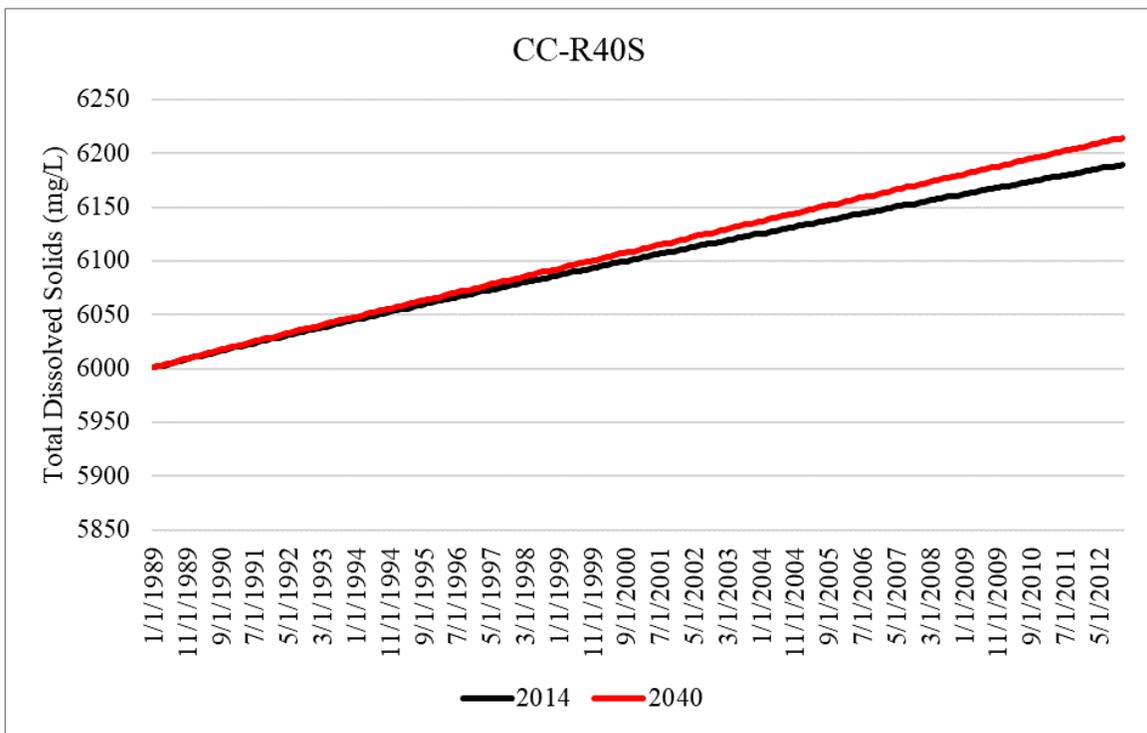
Figure B-28. Simulated total dissolved solids concentrations within the Upper Floridan aquifer for the 2014 and 2040 model runs at CC-R40S in Collier County.
