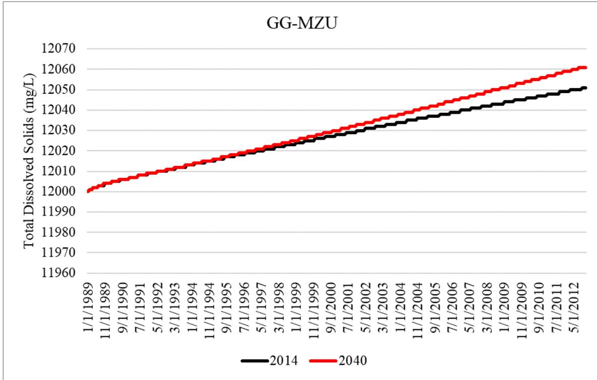
Figure B-29. Simulated total dissolved solids concentrations within the Upper Floridan aquifer for the 2014 and 2040 model runs at GG-MZU in Collier County.
