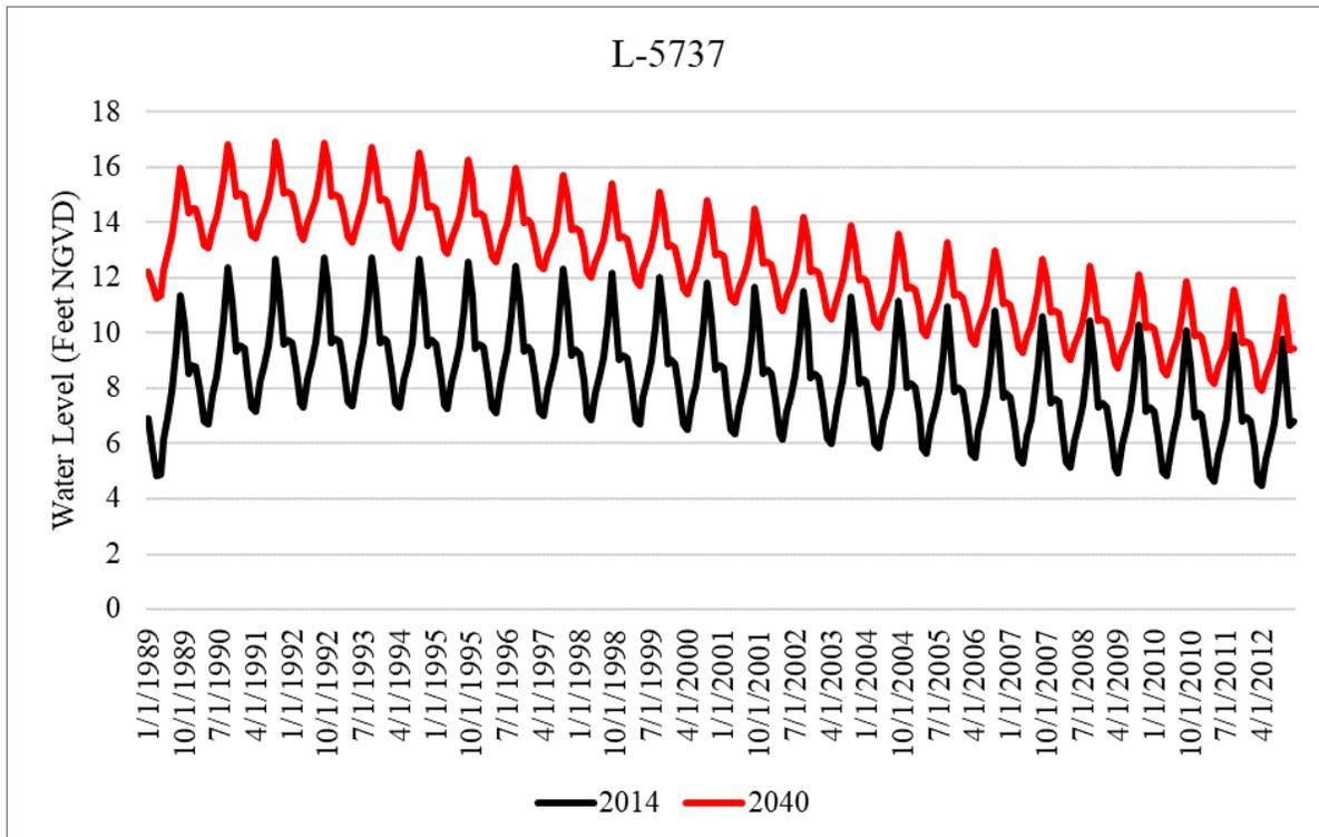
Figure A-6. Simulated water levels within the Upper Floridan aquifer for the 2014 and 2040 model runs at L-5737 in Lee County.
