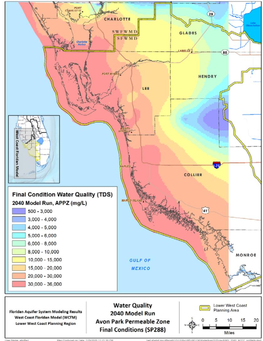
Figure 22. Avon Park permeable zone water quality (total dissolved solids concentrations) for the final condition of the 2040 model run.
