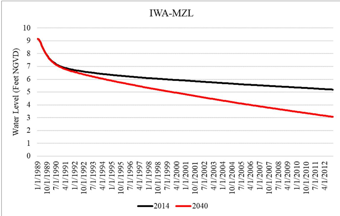
Figure A-7. Simulated water levels within the Lower Floridan aquifer – first permeable zone for the 2014 and 2040 model runs at IWA-MZL in Lee County.
