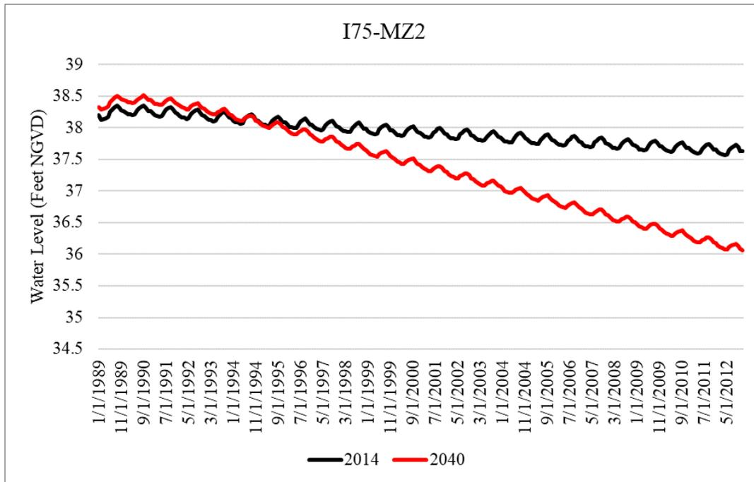
Figure A-9. Simulated water levels within the Upper Floridan aquifer for the 2014 and 2040 model runs at I75-MZ2 in Collier County.
