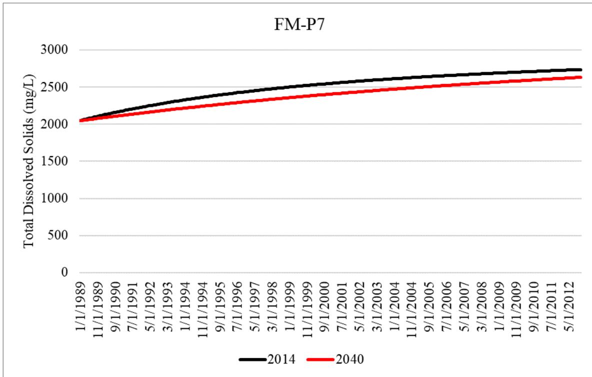
Figure B-10. Simulated total dissolved solids concentrations within the Upper Floridan aquifer for the 2014 and 2040 model runs at FM-P7 in Lee County.
