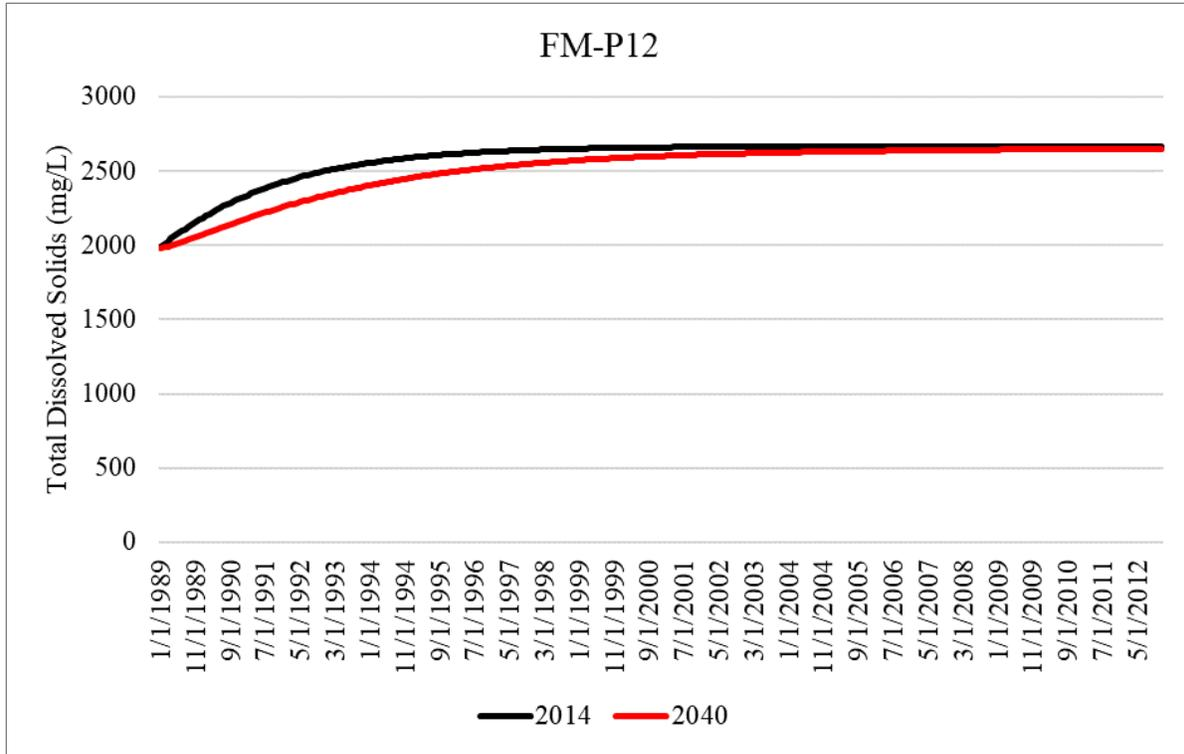
Figure B-9. Simulated total dissolved solids concentrations within the Upper Floridan aquifer for the 2014 and 2040 model runs at FM-P12 in Lee County.
