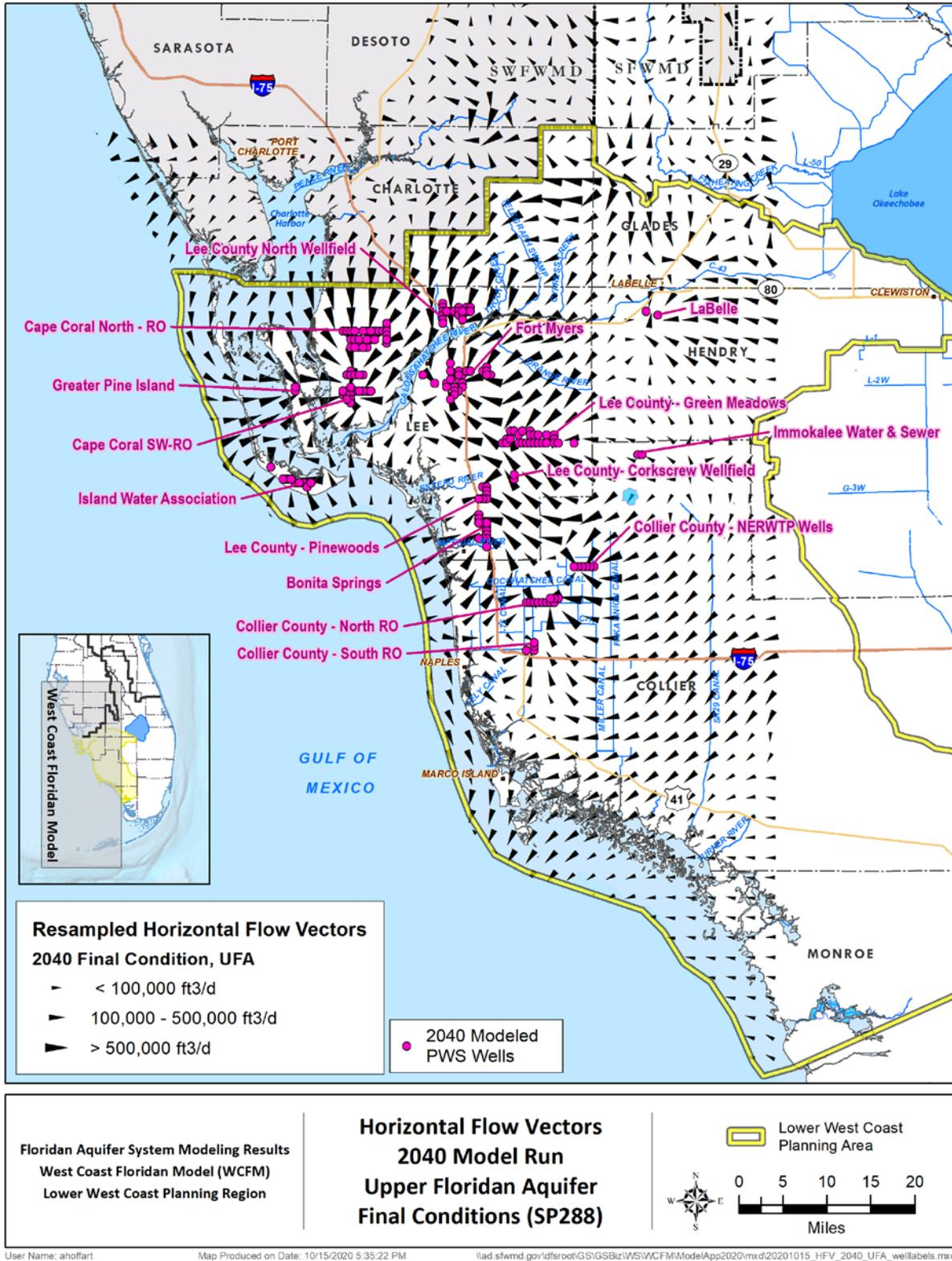
Figure 25. Resampled horizontal flow vectors for the final condition of the 2040 model simulation in the Upper Floridan aquifer.
