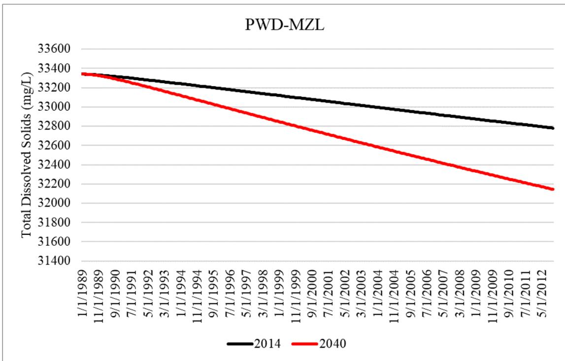
Figure B-20. Simulated total dissolved solids concentrations within the Avon Park permeable zone for the 2014 and 2040 model runs at PWD-MZL in Lee County.
