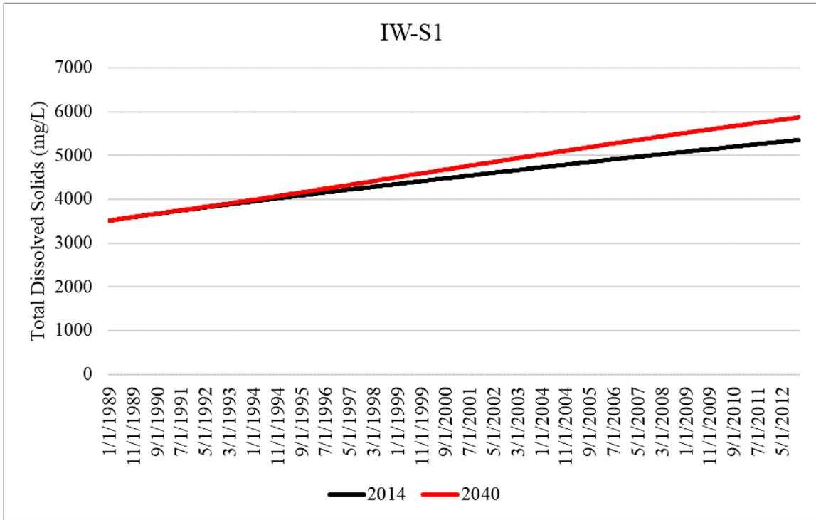
Figure B-13. Simulated total dissolved solids concentrations within the Upper Floridan aquifer for the 2014 and 2040 model runs at IW-S1 in Lee County.
