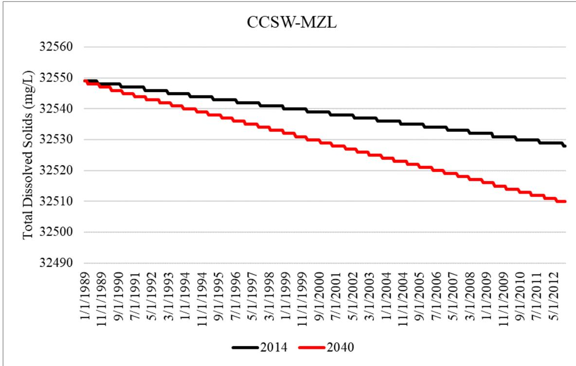
Figure B-31. Simulated total dissolved solids concentrations within the Avon Park permeable zone for the 2014 and 2040 model runs at CCSW-MZL in Collier County.
