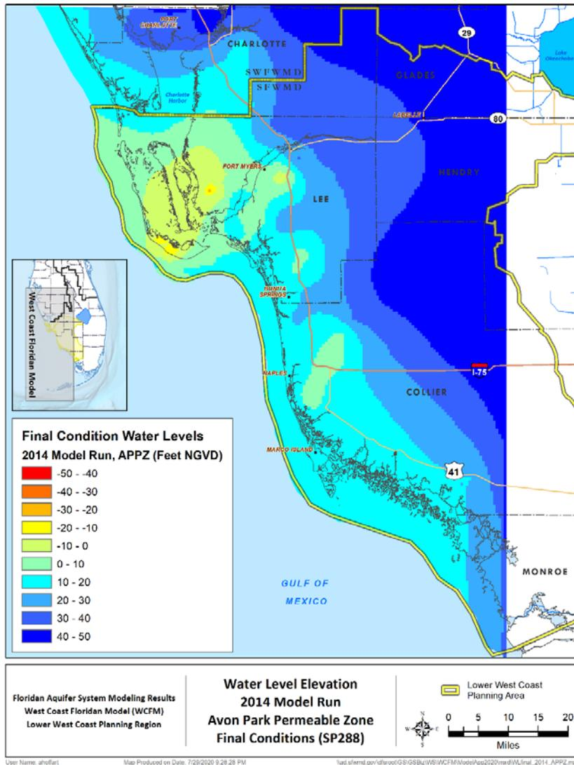
Figure 15. Avon Park permeable zone water levels for the final condition of the 2014 model run.
