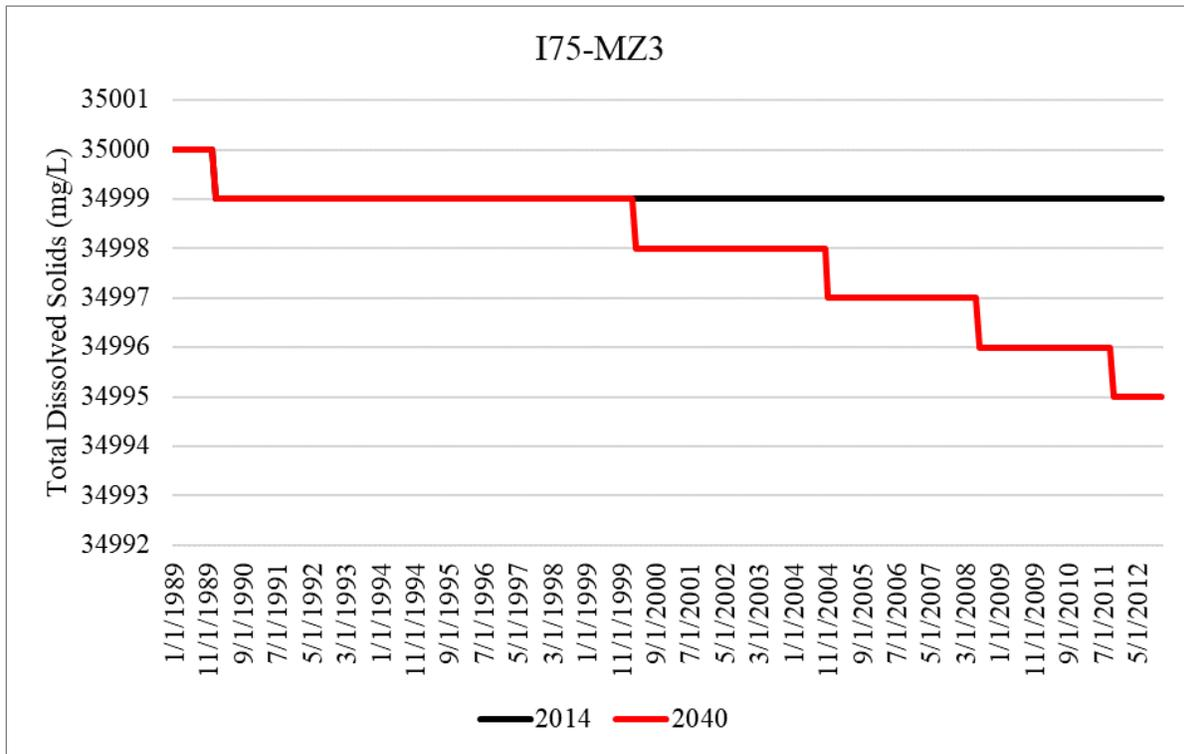
Figure B-32. Simulated total dissolved solids concentrations within the Lower Floridan aquifer – first permeable zone for the 2014 and 2040 model runs at I75-MZ3 in Collier County.
