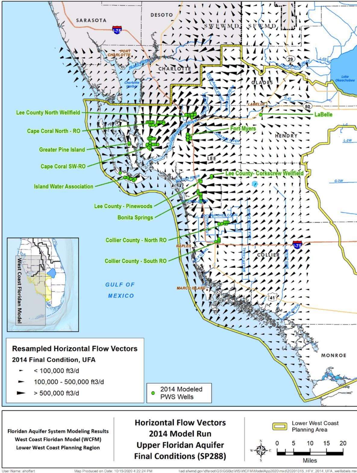
Figure 24. Resampled horizontal flow vectors for the final condition of the 2014 model simulation in the Upper Floridan aquifer.
