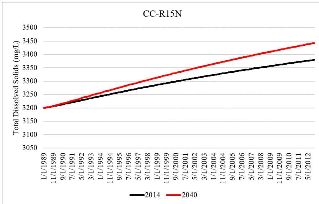
Figure B-22. Simulated total dissolved solids concentrations within the Upper Floridan aquifer for the 2014 and 2040 model runs at CC-R15N in Collier County.
