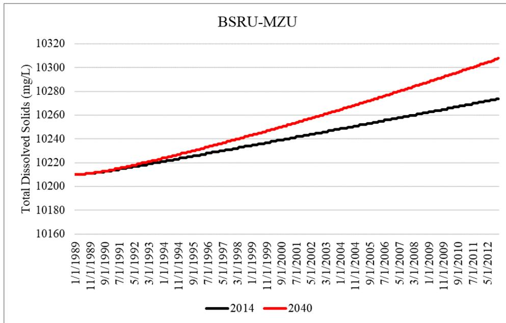
Figure B-2. Simulated total dissolved solids concentrations within the Upper Floridan aquifer for the 2014 and 2040 model runs at BSRU-MZU in Lee County.
