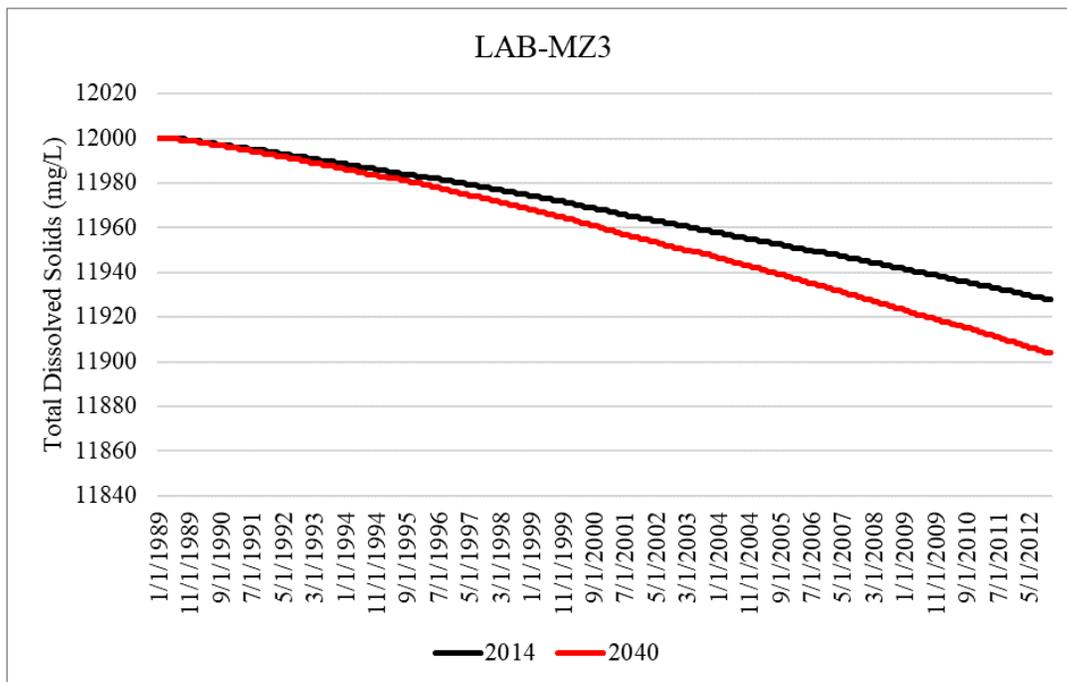
Figure B-34. Simulated total dissolved solids concentrations within the Avon Park permeable zone for the 2014 and 2040 model runs at LAB-MZ3 in Hendry County.
