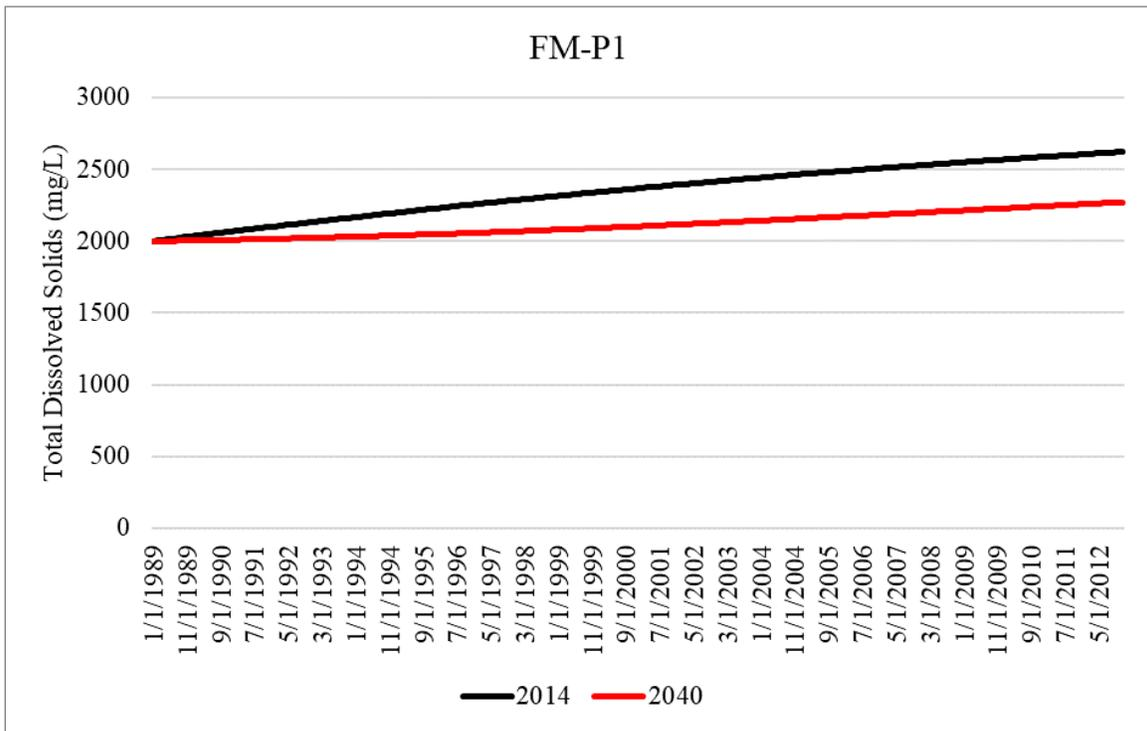
Figure B-8. Simulated total dissolved solids concentrations within the Upper Floridan aquifer for the 2014 and 2040 model runs at FM-P1 in Lee County.
