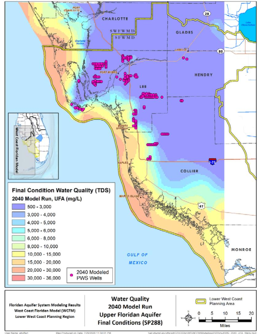
Figure 19. Upper Floridan aquifer water quality (total dissolved solids concentrations) for the final condition of the 2040 model run.
