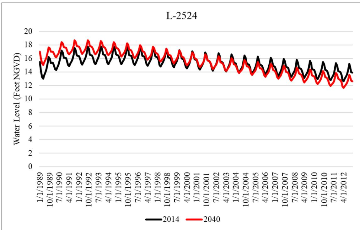
Figure A-4. Simulated water levels within the Upper Floridan aquifer for the 2014 and 2040 model runs at L-2524 in Lee County.
