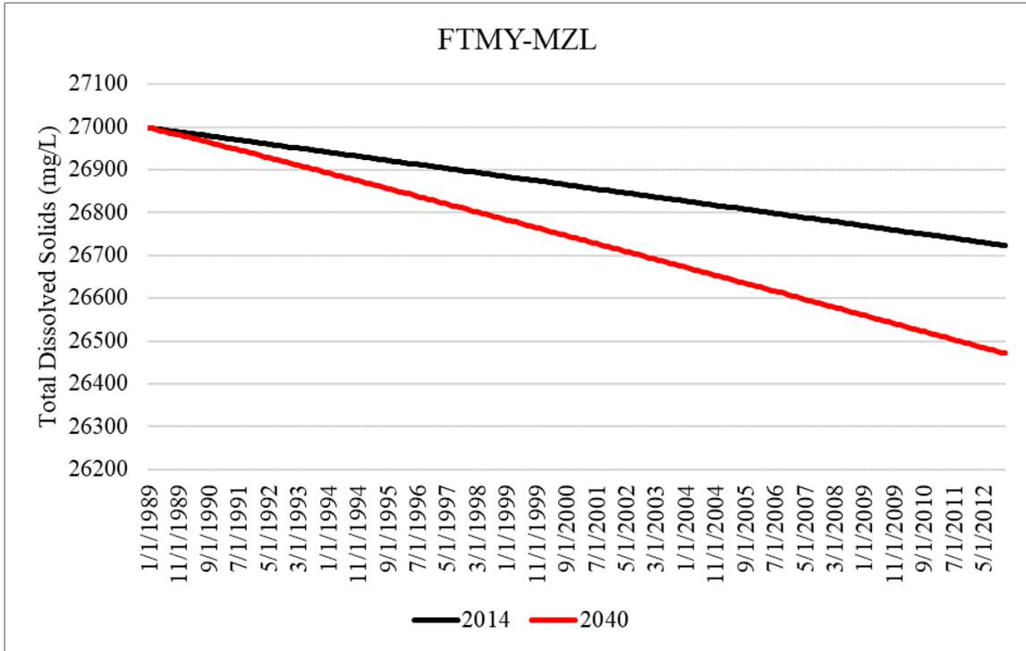
Figure B-11. Simulated total dissolved solids concentrations within the Avon Park permeable zone for the 2014 and 2040 model runs at FTMY-MZL in Lee County.
