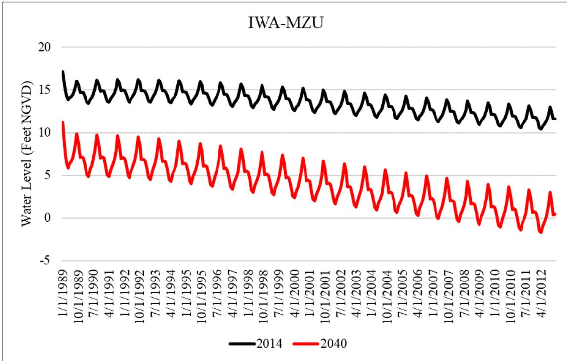
Figure A-3. Simulated water levels within the Upper Floridan aquifer for the 2014 and 2040 model runs at IWA-MZU in Lee County.
