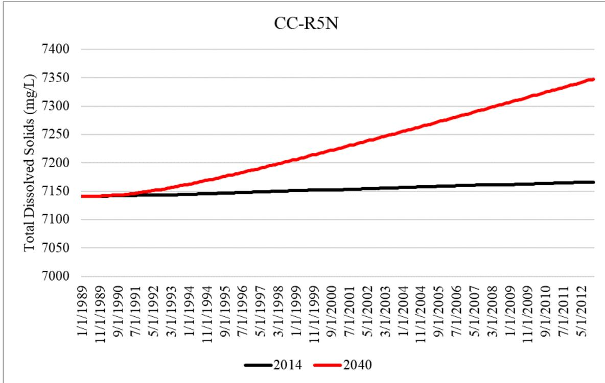
Figure B-23. Simulated total dissolved solids concentrations within the Upper Floridan aquifer for the 2014 and 2040 model runs at CC-R5N in Collier County.
