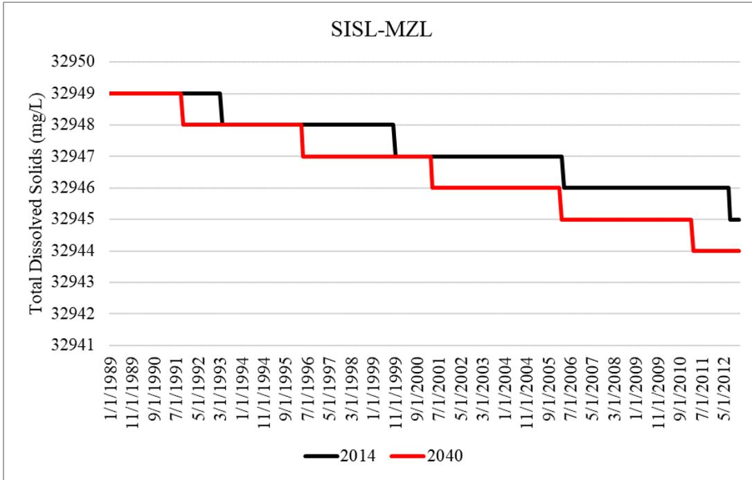
Figure B-17. Simulated total dissolved solids concentrations within the Avon Park permeable zone for the 2014 and 2040 model runs at SISL-MZL in Lee County.
