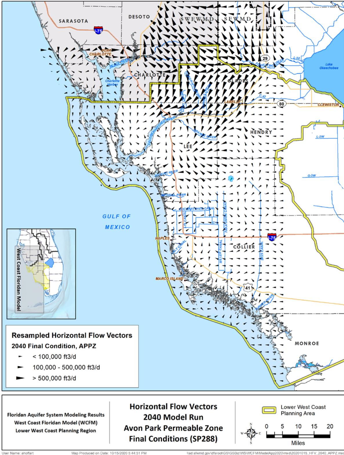
Figure 27. Resampled horizontal flow vectors for the final condition of the 2040 model simulation in the Avon Park permeable zone.
