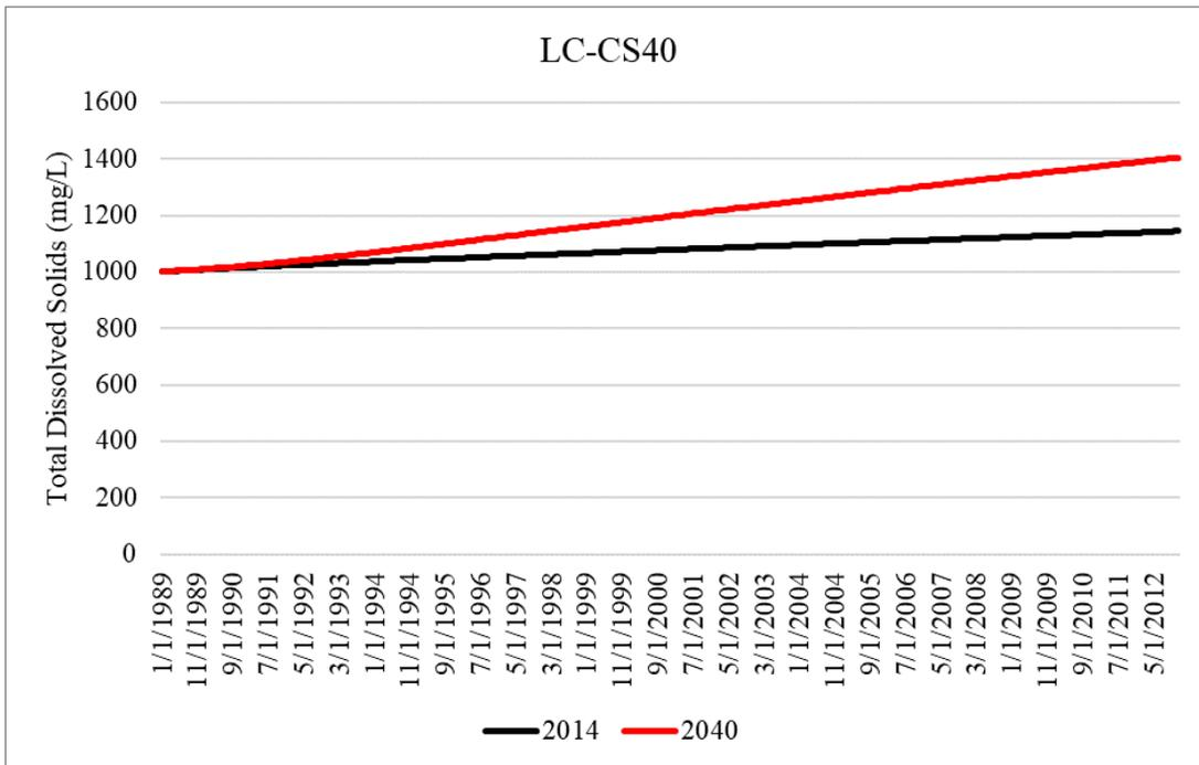
Figure B-18. Simulated total dissolved solids concentrations within the Upper Floridan aquifer for the 2014 and 2040 model runs at LC-CS40 in Lee County.
