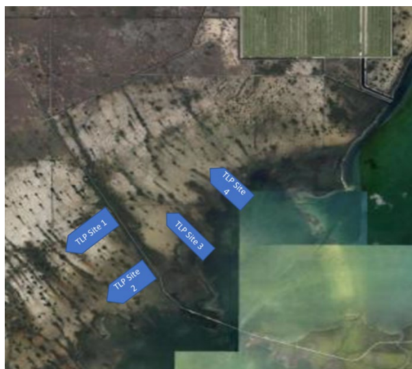
Figure 28. Each transect would be L=1000 ft; W=500 ft; Depth= 4 inches and require some 8000 cubic yards of TLP
