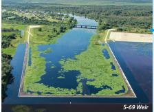
• **Weirs:** Structures across a canal or stream that block the flow of water until the water flows over the structure.
