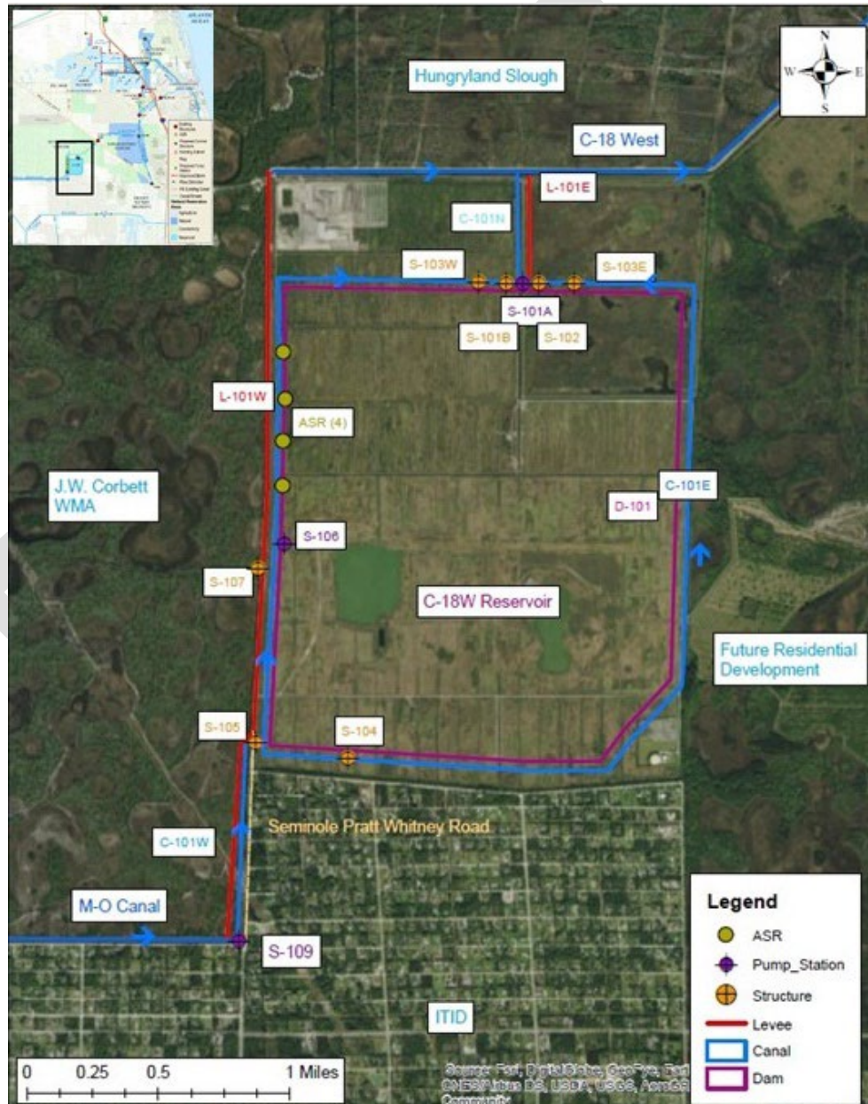
Figure 1-5. Flow-way 2 structures and flows (From: USACE 2020).
