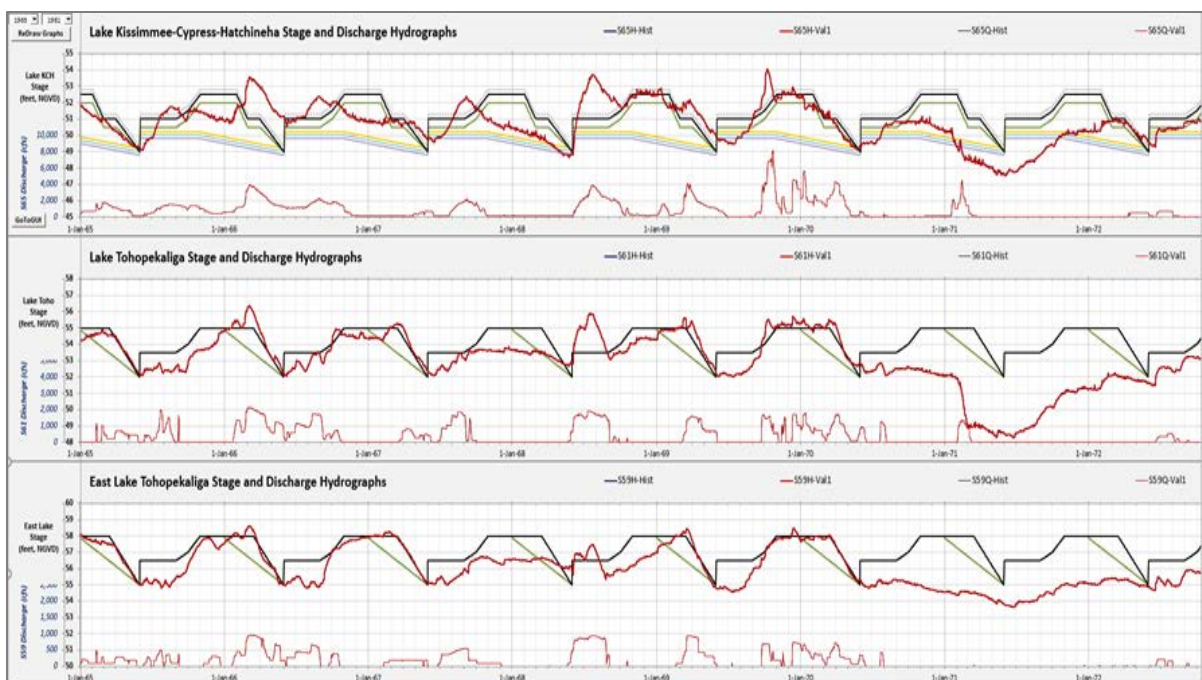
Figure 6-1. Simulated validation (red) and historical (black) hydrographs for 1965 to 1972.
