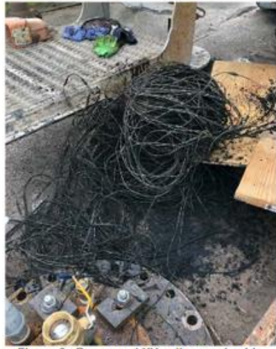
Figure 6. Recovered XY caliper tool cable.
