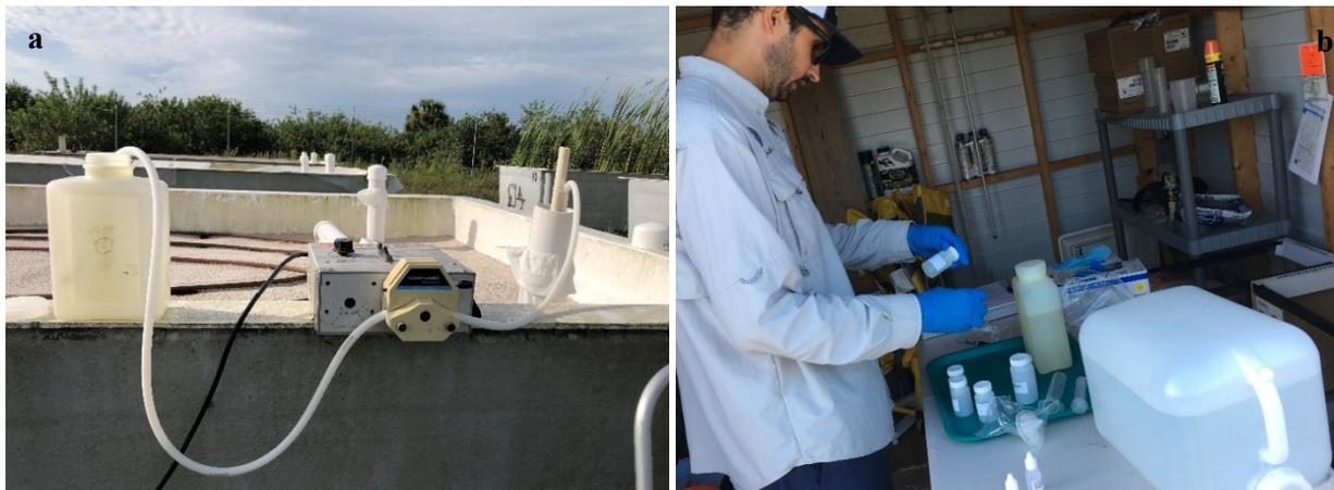
**Figure 6.** a) Water sample collection with peristaltic pump, b) Sample processing.
