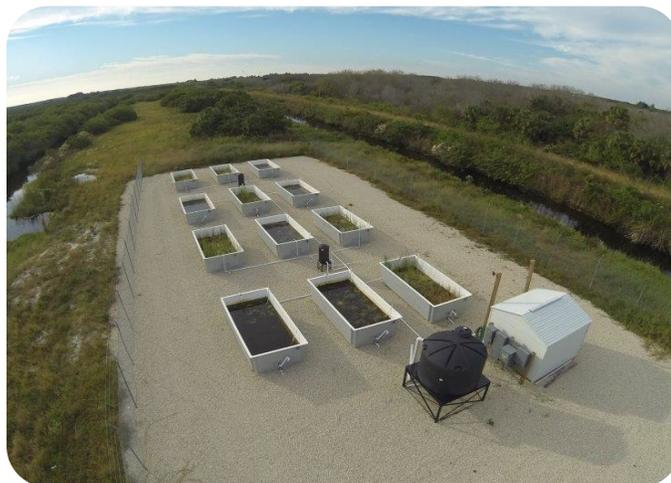
**Figure 2.** Aerial overview of mesocosm tanks, head tank and sub-head tanks.
