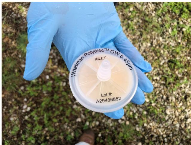
**Figure 16.** Filter after processing a water sample from a Bold&Gold® CTS mesocosm
