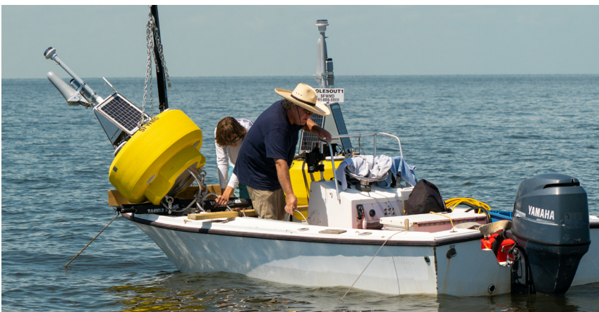
SFWMD Staff Deploying Nexsens CB 450 Data Buoys on Lake Okeechobee to Help Monitor Water Quality Across the Lake. (Photo by SFWMD)
