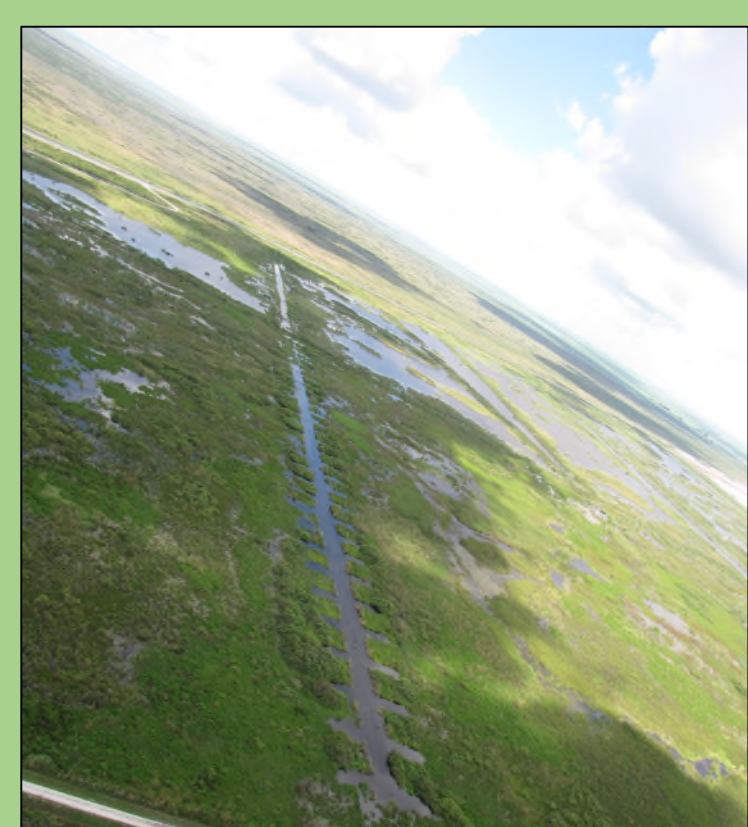
STA-1E Western view of the degraded east-west levee in Cell 6
