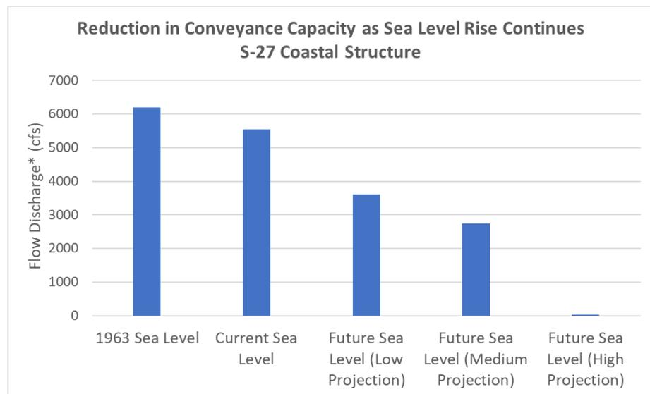
Figure 30. Reduction in conveyance capacity at S-27 as SLR continues.
