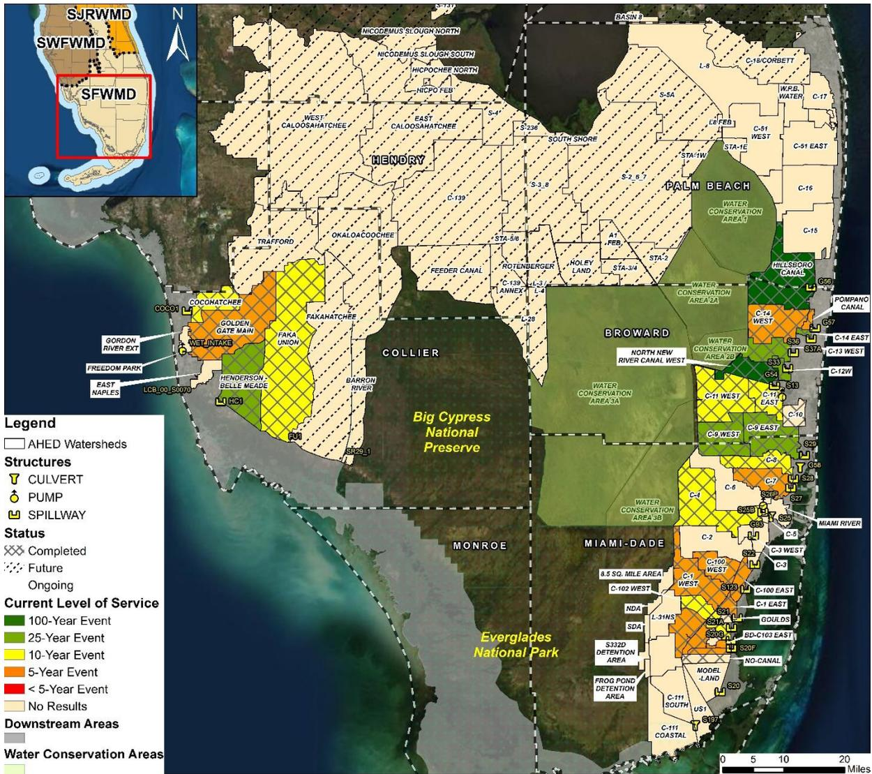
Figure 3. Current Flood Protection Level of Service generally provided by existing infrastructure in critical basins, predominantly located in Broward and Miami-Dade Counties. The Level of Service is represented by the respective rainfall frequency event that results in flooding within areas of each basin, simulated as part of completed FPLoS Phase I – Flood Vulnerability Assessments.
