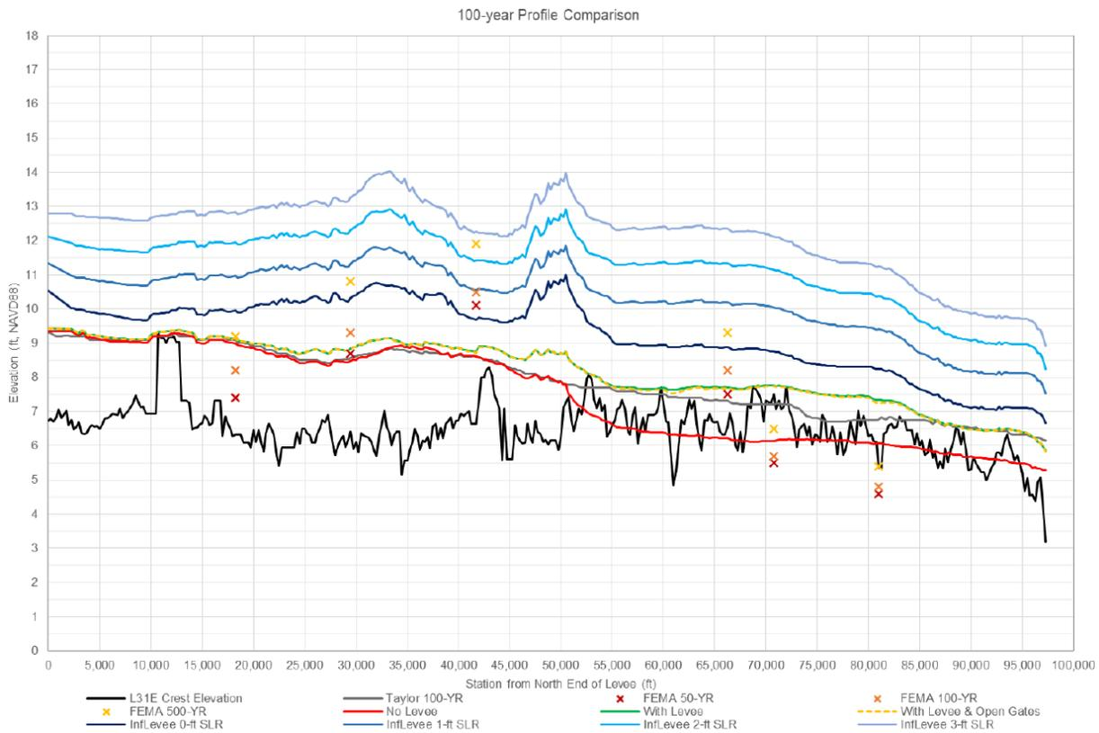
Figure 36. 100-Year Profile for Levee Crest Elevation Consideration.
