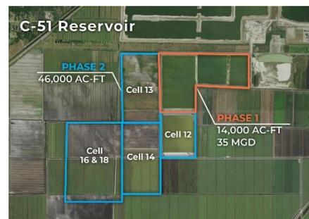
Figure 11. Plan view area of C-51 Reservoir project.
