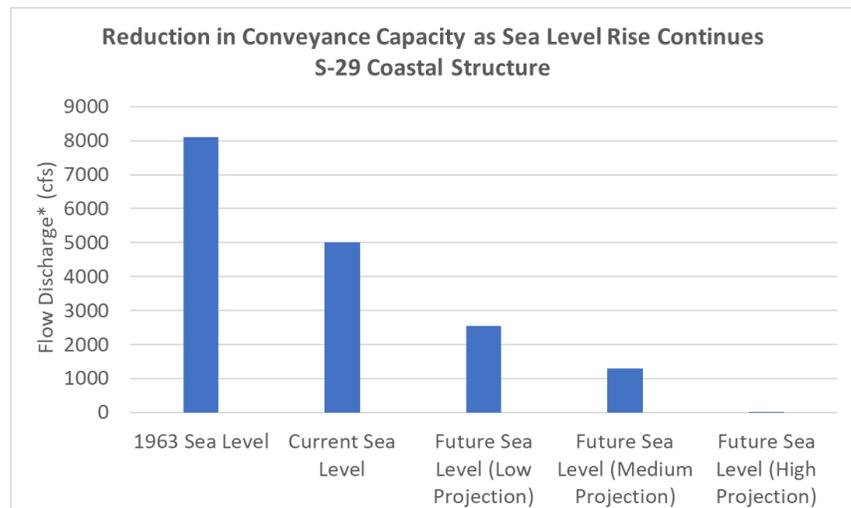
Figure 32. Reduction in conveyance capacity at S-29 as SLR continues
