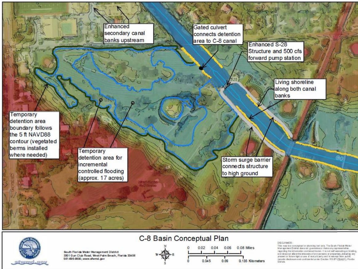
Figure 34. Conceptual plan for the C-8 Basin.
