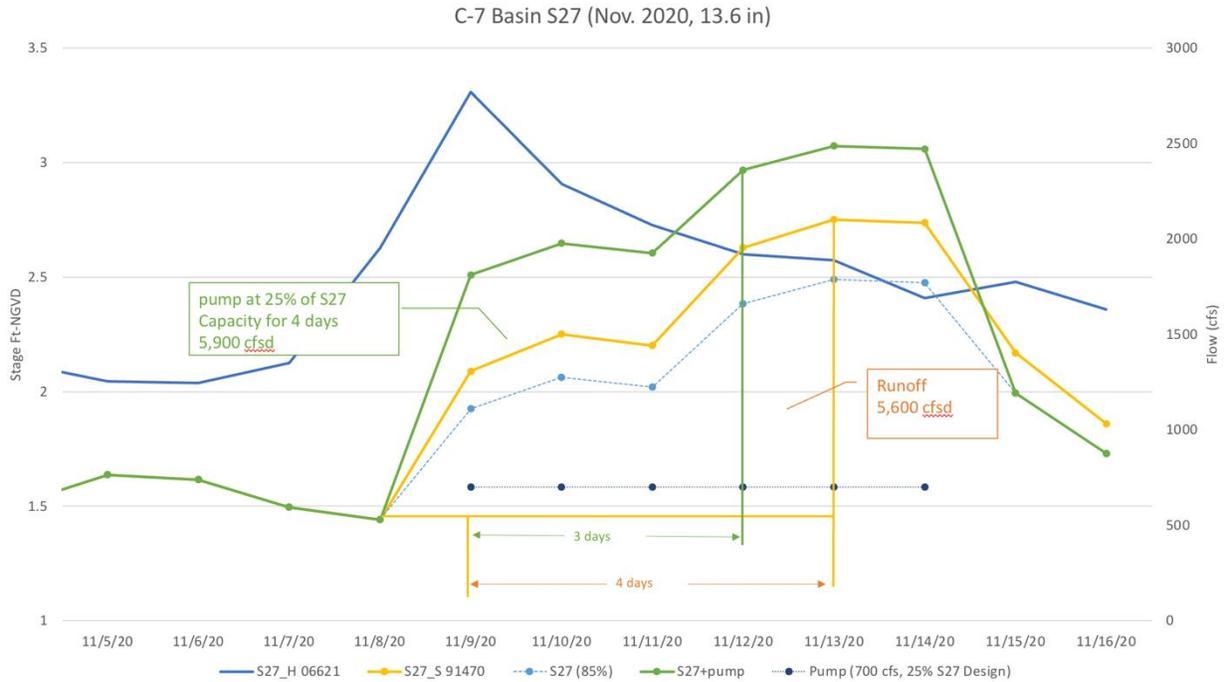
Figure 10. Potential amount of time needed to remove the cumulative flows at S-27 (5600 cfsd total runoff to bring the stages back to normal operating ranges during Tropical Storm Eta in November 2020) for the scenario with forward pumps sized at 25% of the spillway design capacity (3 days) relative to the no pump scenario (4 days)
