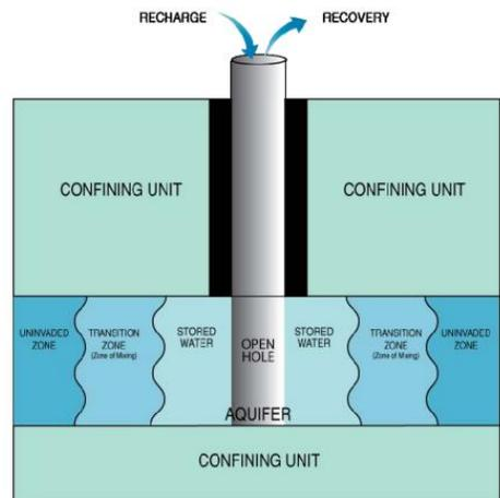
Figure 10. Graphic showing Aquifer Storage and Recharge (ASR) methodology.
