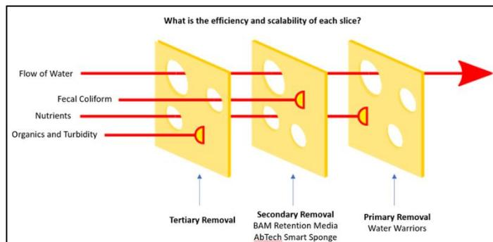
manage nutrient loads and eutrophication, the proposed multi layered approach takes the form of multiple locations and technologies of nutrient removal with the goal of eventually scaling appropriate solutions until contaminants are contained within the ideal limits. Future iterations may look at the reductive effects of incorporating NBS.
