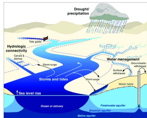
Figure 8. Diagram depicting elements of the coastal hydrologic cycle.
