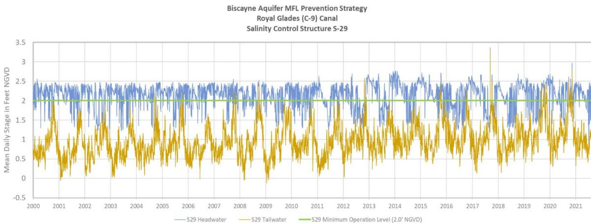
Figure 26. Headwater and Tailwater stages at S-29 structure.
