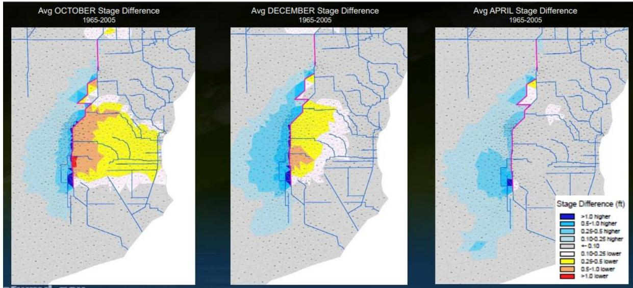
Figure 17. H&H modeling results illustrating the average water stage difference with and without the full extent curtain wall scenario.
