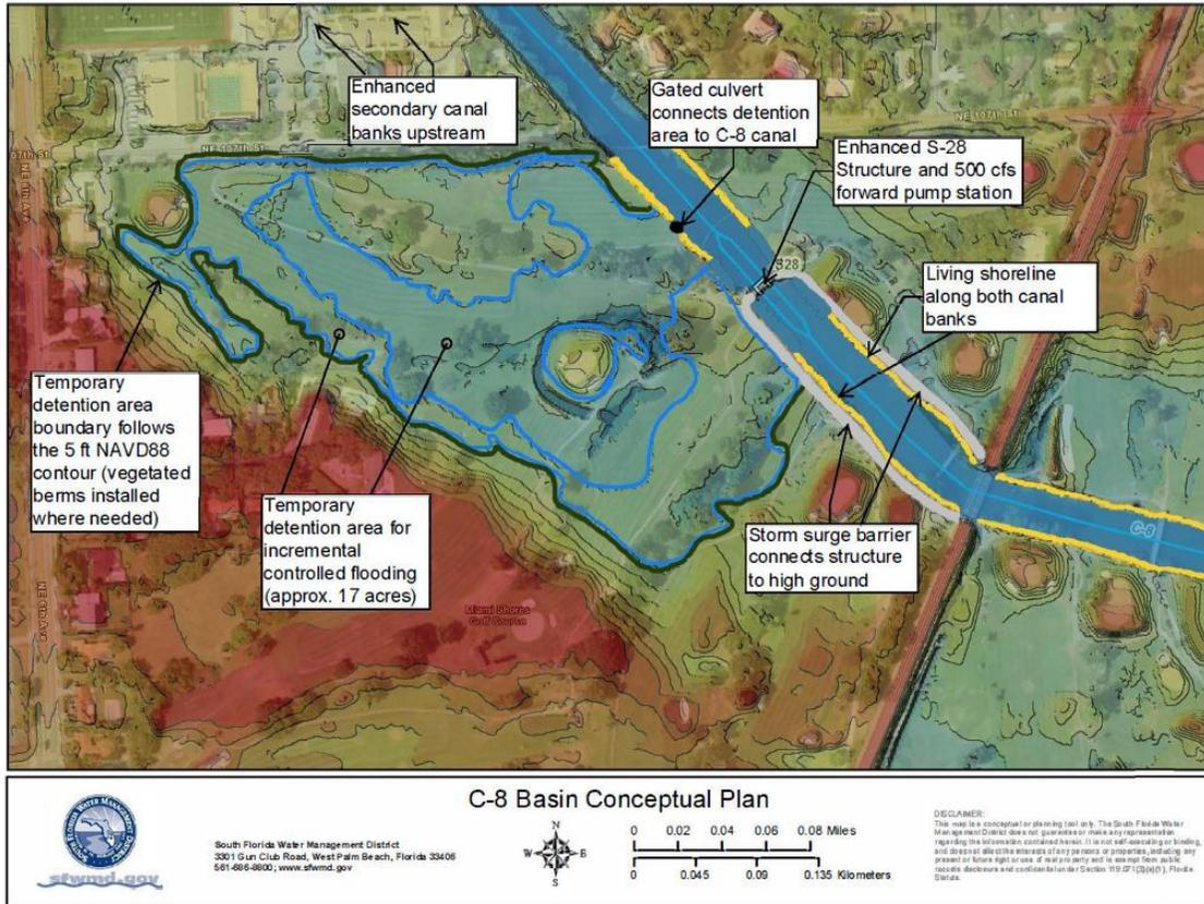
Figure 6. Conceptual plan for the C-8 Basin.
