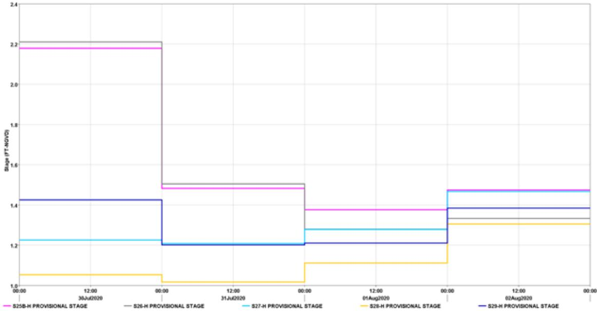
Figure 12. Observed Headwater Stages during Hurricane Isaias, in July/August 2020, at Coastal Structures with forward pump (S-25B and S-26) vs. Coastal Structures with gravity discharge only (S-27, S-28, S-29)
