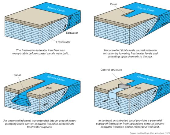
Figure 7. Diagram depicting the impact of canals and structures on saltwater intrusion.
