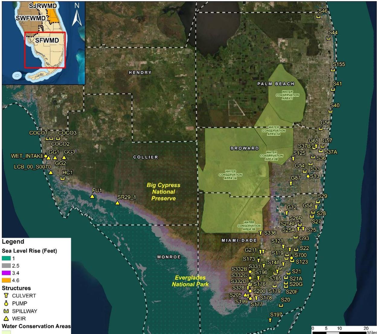
Figure 35. Potential impacts of rising sea levels in South Florida to water control structures.
