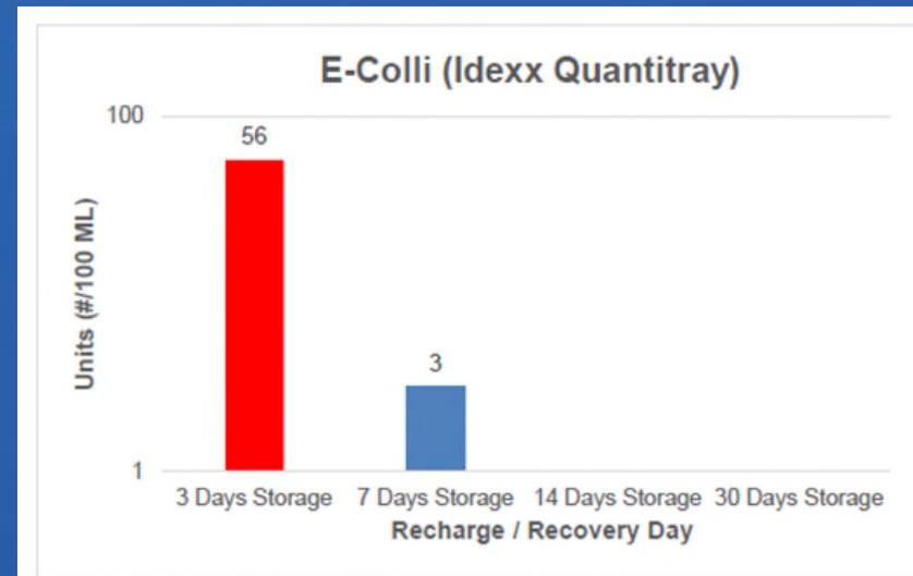
Figure 3. Cycle Test 6C ASR-1 Well E-Coli Results.
