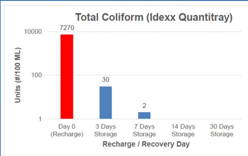
Figure 1. Cycle Test 6C ASR-1 Well Total Coliform Results.
