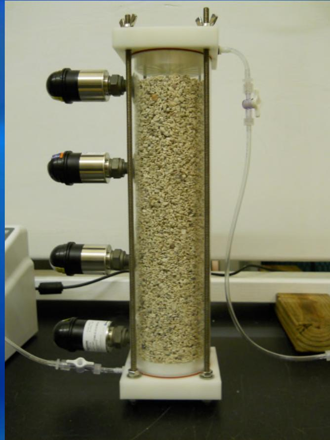
Crushed core (no biofilm at  $T_0$ )
