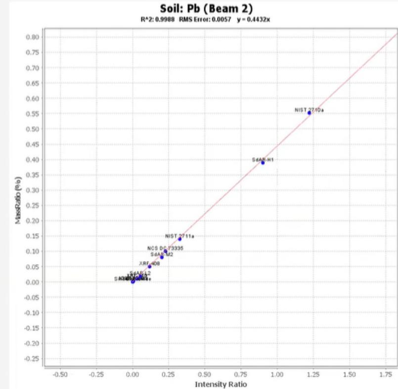
These are example of calibration curves for Mo, Hg, and Pb. Working with SciAps we modified the calibrations to fit our needs.
