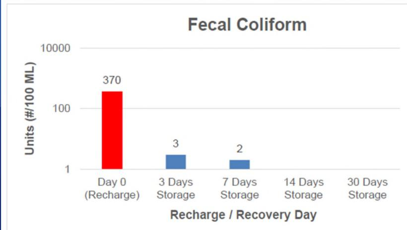
Figure 2. Cycle Test 6C ASR-1 Well Fecal Coliform Results.
