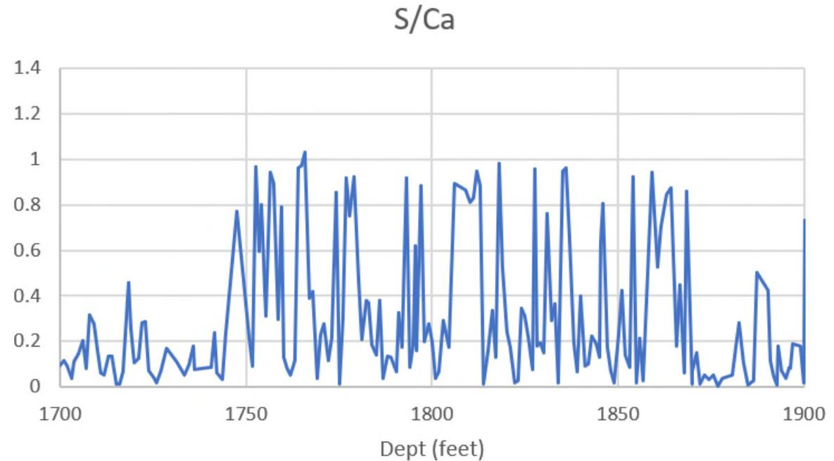
Figure S/Ca: S vs. Ca ratios for core intervals where massive and nodular gypsum occurs. S/Ca ratio for pure gypsum = 1. Change et al. (1998) report a S/Ca ratio of gypsum from limestone of approximately 0.8.
