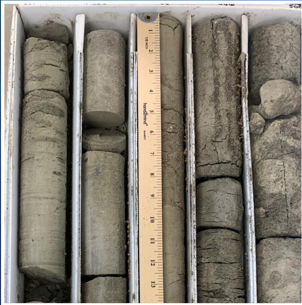
**Goal: to chemically analyze the core from ASR L63N to find areas of potentially high metal concentrations using a hand held X-Ray fluorescence (XRF).**
