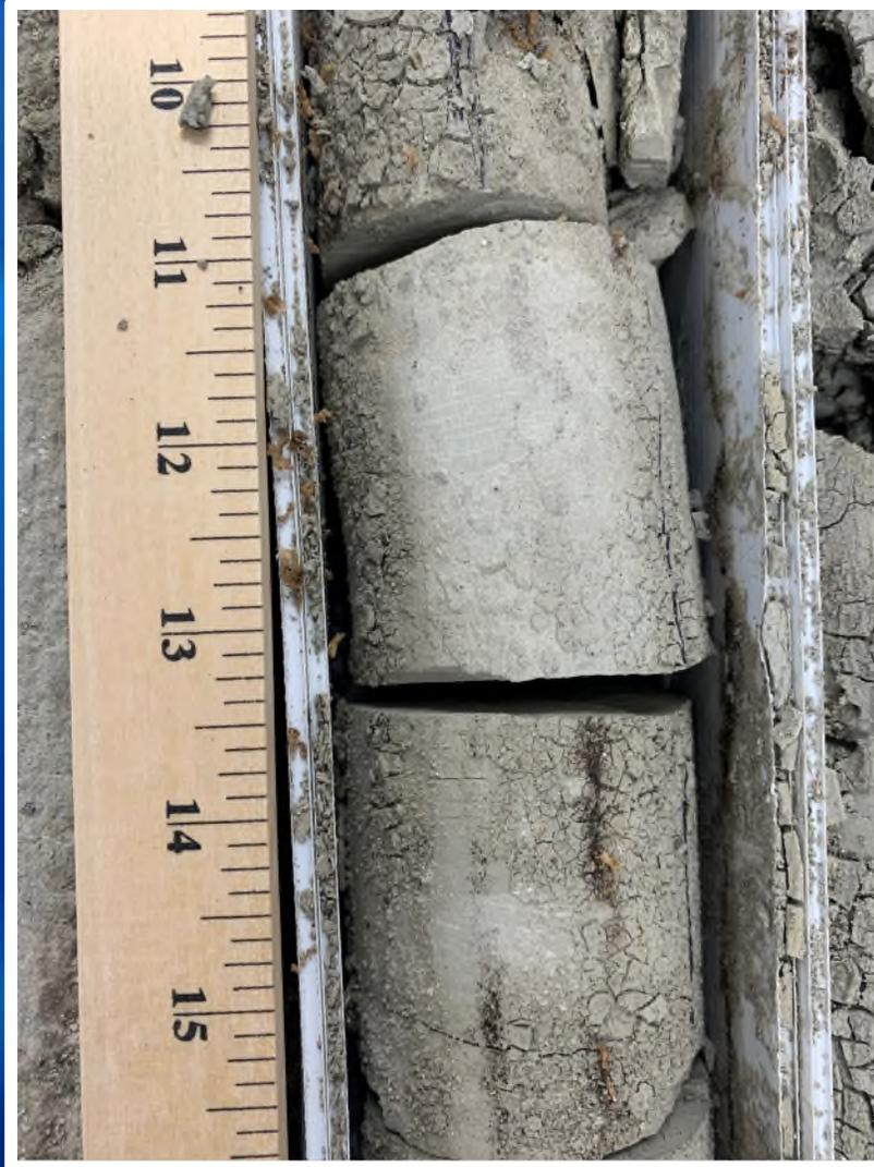
Debris and rust were cleaned off of the core surface using a wire brush before every analysis.
