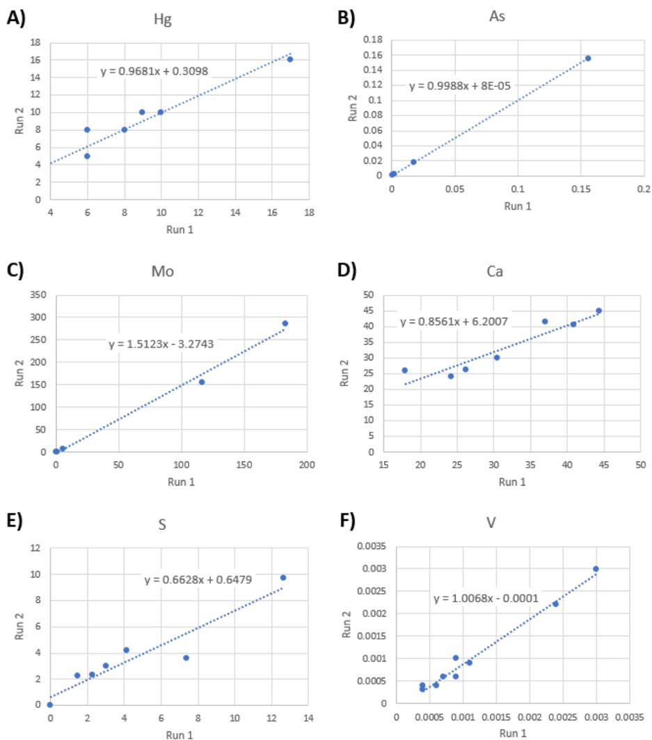
9 samples from core L63N were each analyzed twice – i.e., run 1 and run 2.
