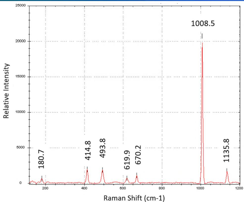
Figure Raman: Raman analysis of gypsum from core L63N. This sample, along with another sample, are a  $\geq 97\%$  match to gypsum's Raman wave number positions.
