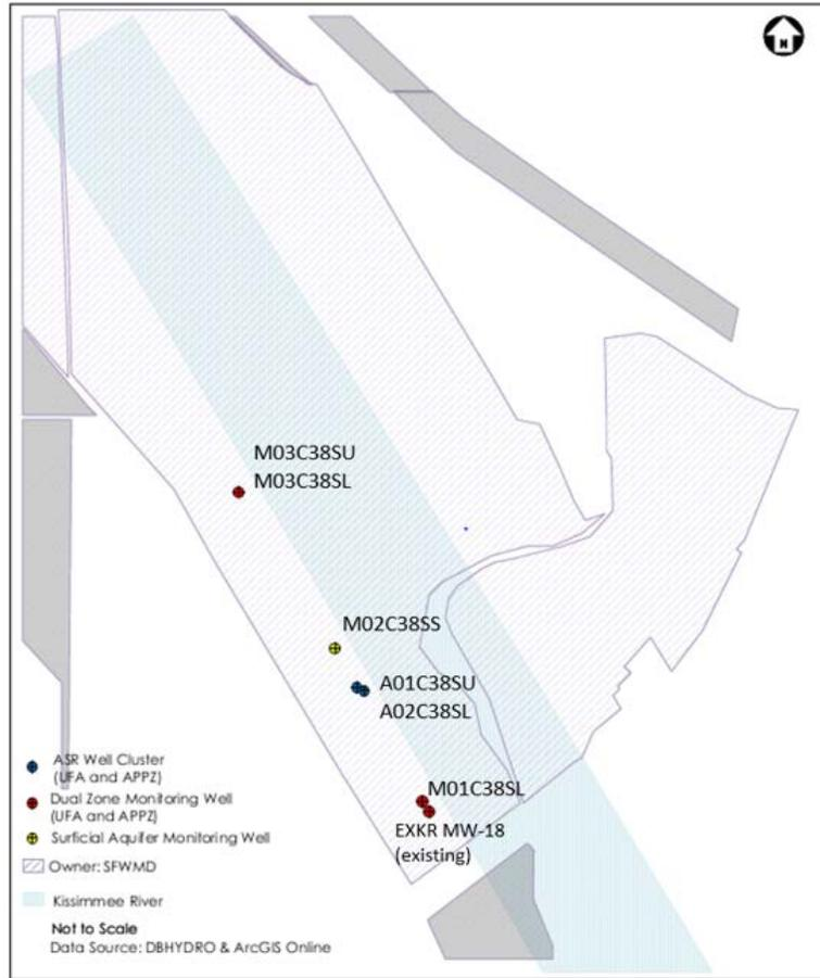
Figure 3-1. C-38S ASR test well and monitoring well layout.
