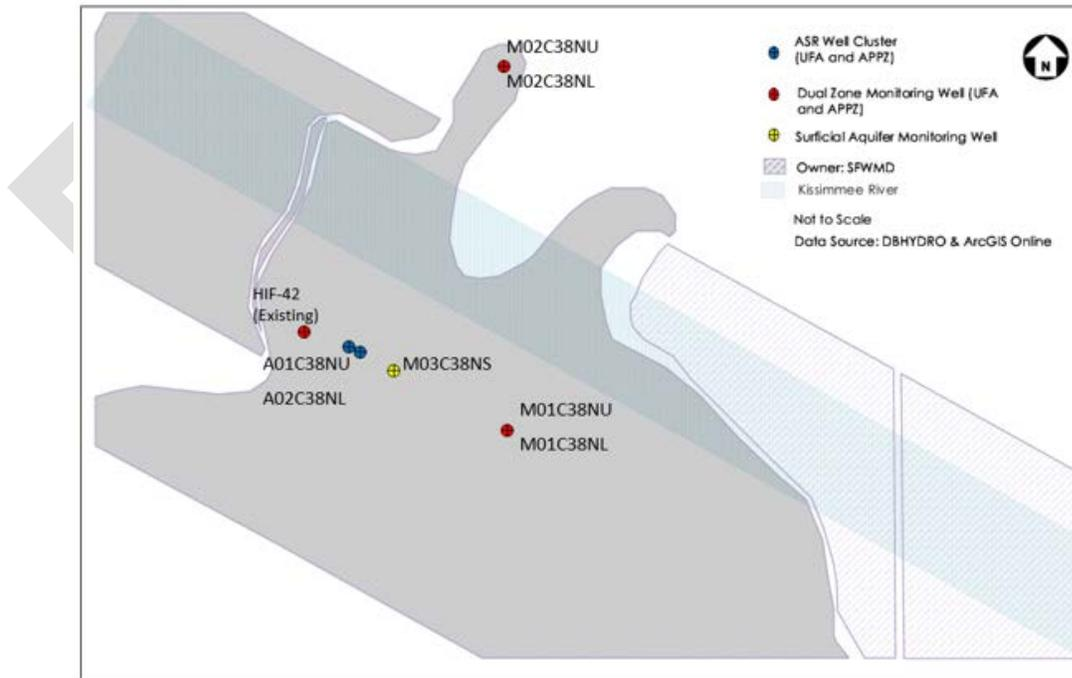
Figure 3-2. C-38N ASR test well and monitoring well layout.
