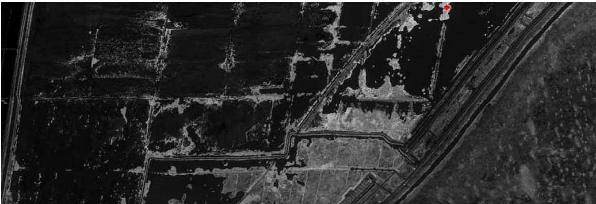
Figure 6-5: Example fraction images and endmember spectra (endmember locations are marked with a red dot), based on Abacus® Level 1 analysis of Probe-1 hyperspectral imagery. Two distinct classes of green (photosynthetic) vegetation were identified. The top image shows the distribution of a vegetation type whose spectrum is shown in the left-hand plot, and is believed to represent SAV. The bottom image shows the distribution of the material whose spectrum is plotted on the right, and is believed to represent non-SAV. Each pixel in these images is associated with a quantitative value indicating the % abundance of the given vegetation type (areas that are bright indicate a high abundance). The Level 2 (more detailed) Abacus® analysis breaks these two vegetation classes into a total of 11 different sub-categories (see Appendix B).
