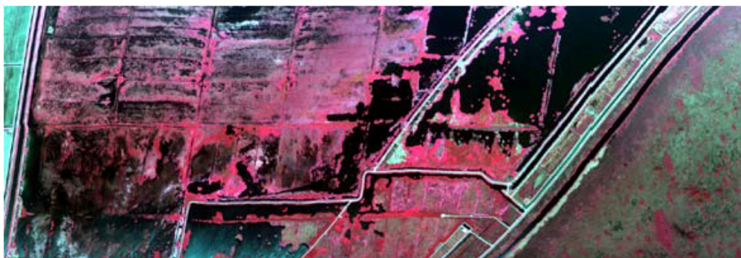
Figure 5-2: False color composite created from Probe-1 hyperspectral image, with 0.65 \mu\text{m} in red, 0.56 \mu\text{m} in green, and 0.45 \mu\text{m} in blue. The HSI data were not georectified for this study, but would be for future collections, particularly where precise identification of ground truth locations in the HSI scene is necessary.
