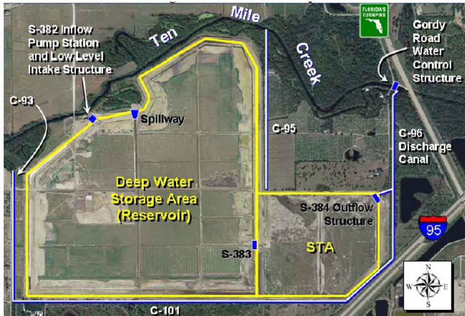
Figure 8. Ten Mile Creek WPA Project components.
