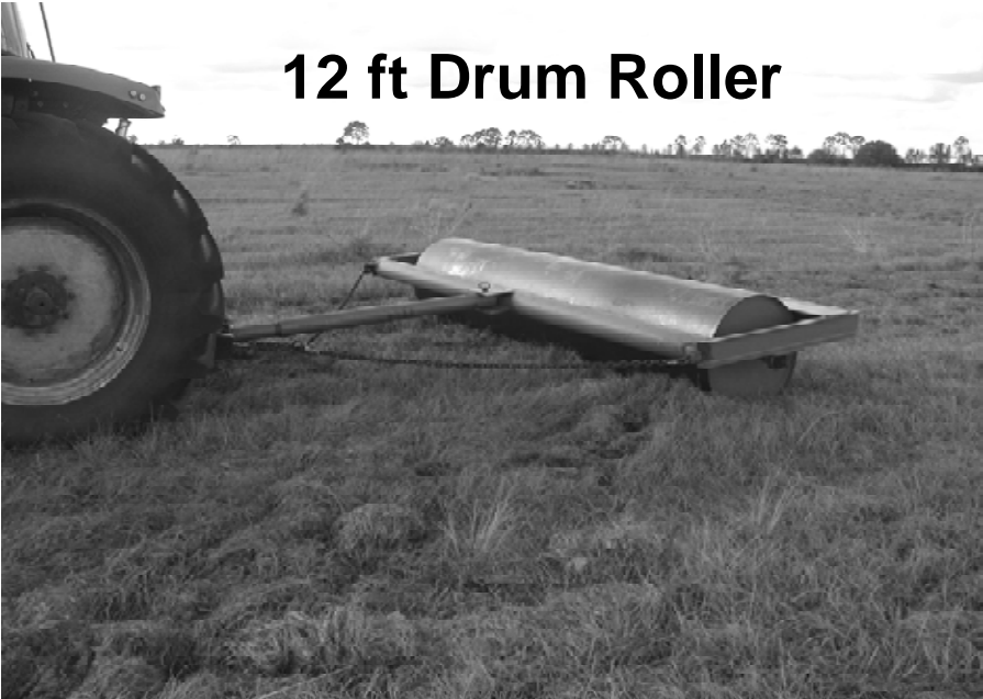
Figure 4. Twelve ft drum roller that was used to compact the soil after disking.
