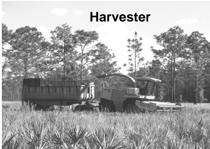
Figure 6. Green silage cutter used to harvest seed from Avon Park Bombing Range. The harvester projected seed directly into a tractor trailer.
