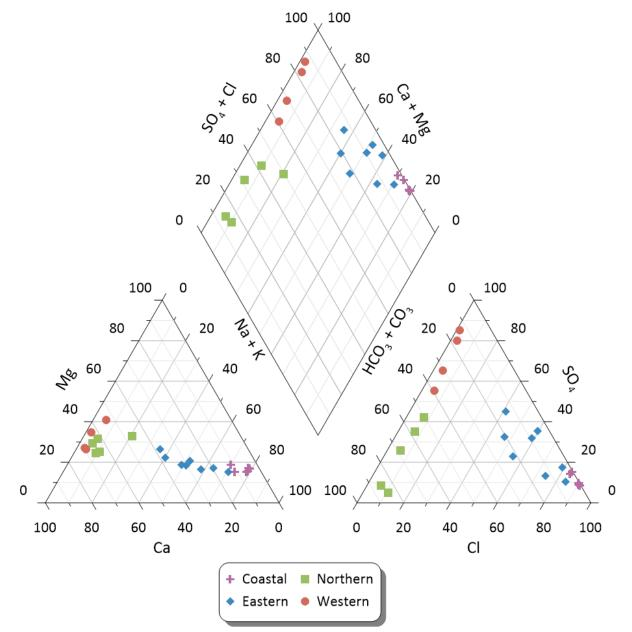
Figure 25. Piper diagram of water types from Lower Floridan aquifer-upper permeable zone water quality results.
