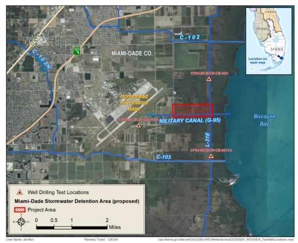
Figure 5. Locations of core borings as part of the surficial aquifer system investigation in the Biscayne Bay area.
