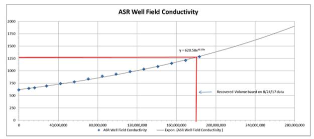
Figure 13. Specific conductivity of the water recovered from the Hillsboro ASR well during Cycle 4.
