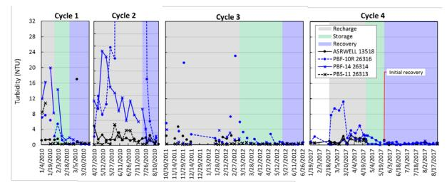
Figure 22. Water turbidity from the Hillsboro ASR well and monitoring wells during the four test cycles.
