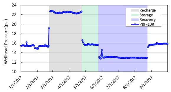
Figure 14. Wellhead pressure (in psi) in storage zone monitoring well PBF-10R in response to recharge, storage, and recovery at the Hillsboro ASR site during Cycle 4.
