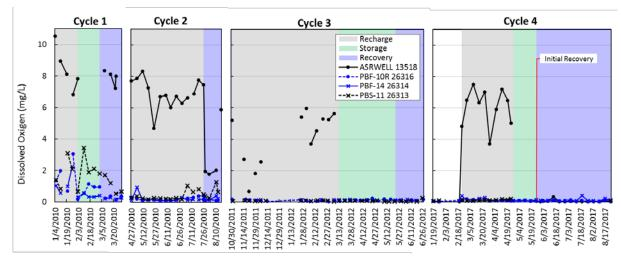
Figure 23. Dissolved oxygen concentrations from the Hillsboro ASR well and monitoring wells during the four test cycles.
