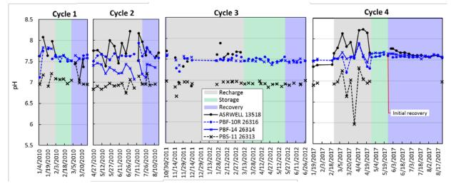
Figure 21. Water pH levels from the Hillsboro ASR well and monitoring wells during the four test cycles.
