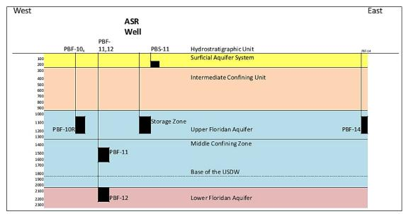
Figure 5. Aquifer cross-section showing the vertical relationship of the monitoring wells and ASR well at the Hillsboro ASR site.
