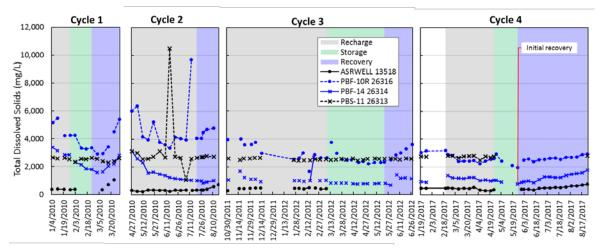
Figure 27. Total dissolved solids concentrations in water from the Hillsboro ASR well and monitoring wells during the four test cycles.
