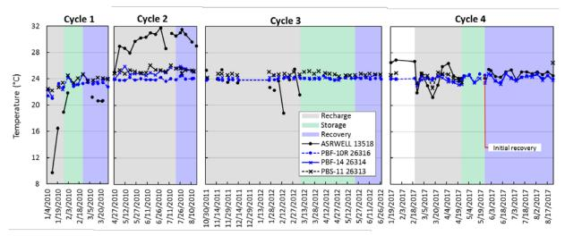
Figure 20. Water temperature from the Hillsboro ASR well and monitoring wells during the four test cycles.
