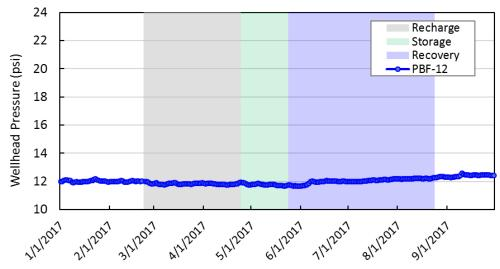
Figure 17. Wellhead pressure (in psi) in monitoring well PBF-12 during operation of the Hillsboro ASR well.
