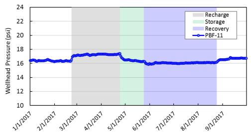
Figure 16. Wellhead pressure (in psi) in monitoring well PBF-11 during operation of the Hillsboro ASR well.
