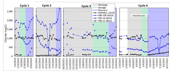
Figure 26. Chloride concentrations in water from the Hillsboro ASR well and monitoring wells during the four test cycles.
