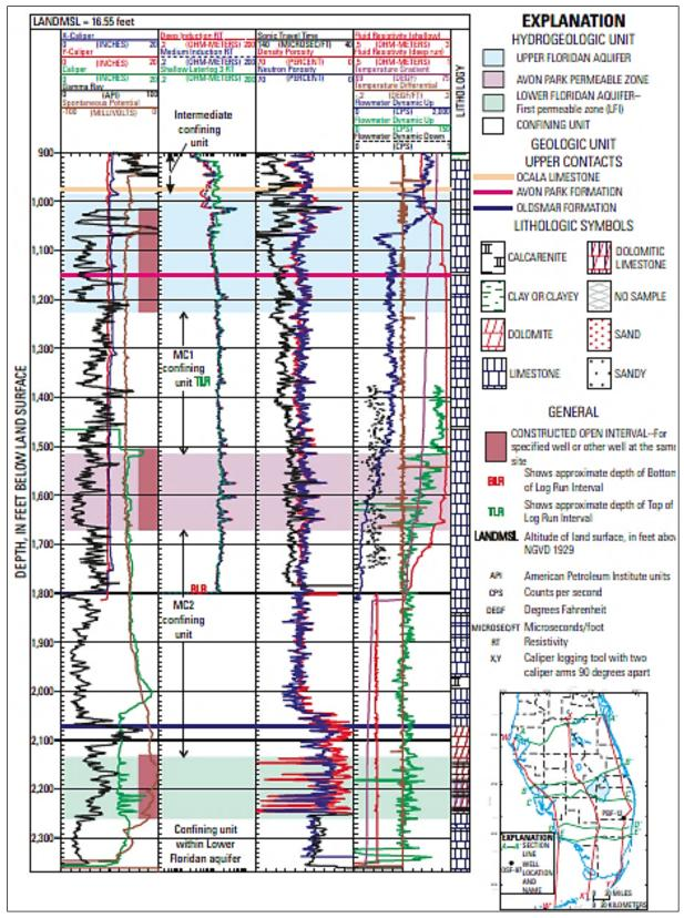
Figure 8. Compilation of geophysical logs from the Hillsboro ASR system (From: United States Geological Survey 2008).
