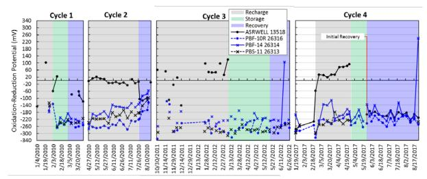
Figure 24. Oxidation reduction potential of water from the Hillsboro ASR well and monitoring wells during the four test cycles.
