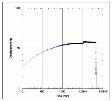
Figure 10. Drawdown response of water levels in monitoring well PBF-14, located 1,010 feet away from the ASR well.
