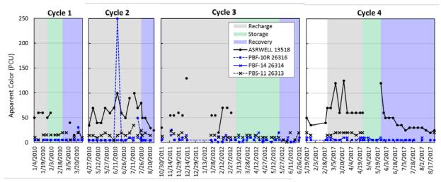
Figure 18. Water color from the Hillsboro ASR well and monitoring wells during the four test cycles.
