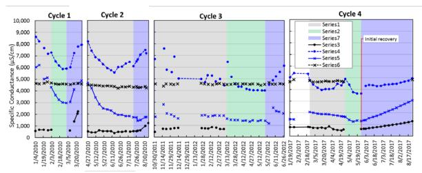
Figure 25. Specific conductivity of water from the Hillsboro ASR well and monitoring wells during the four test cycles.
