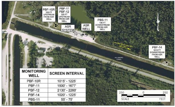
Figure 6. Locations of the monitoring wells and ASR well at the Hillsboro ASR site.
