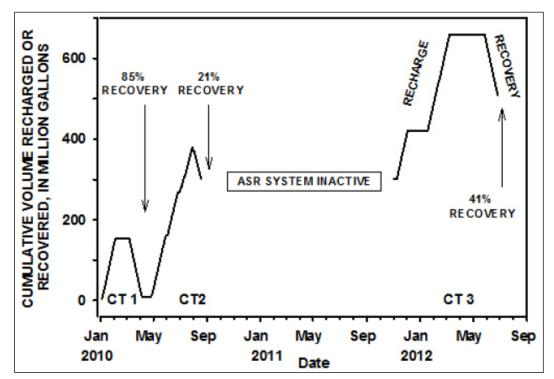
Figure 12. Hillsboro ASR facility cumulative recharge, storage, and recovery volumes (gallons) during the first three test cycles.
