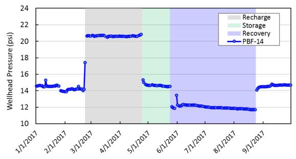
Figure 15. Wellhead pressure (in psi) at storage zone monitoring well PBF-14 in response to recharge, storage, and recovery at the Hillsboro ASR site during Cycle 4.
