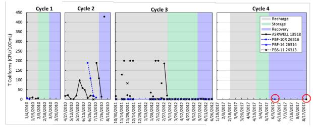
Figure 28. Total coliform bacteria concentrations in water from the Hillsboro ASR well and monitoring wells during the four test cycles.
