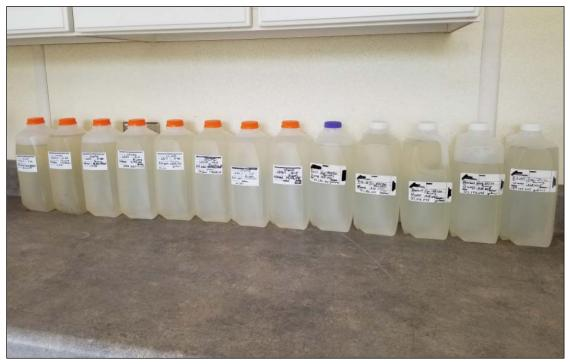
Figure 19. Weekly water samples collected from the Hillsboro ASR wellhead during the recovery phase of Cycle 4.
