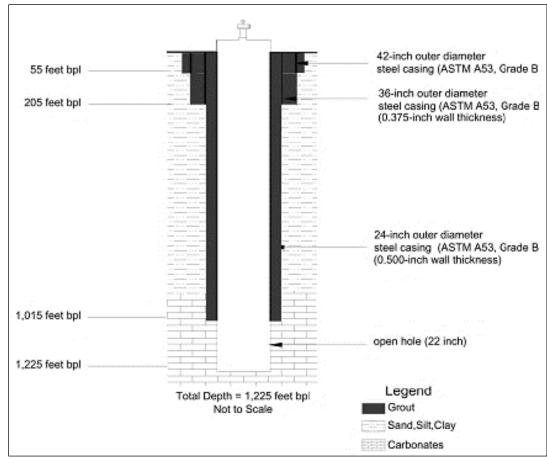
Figure 3. Hillsboro ASR well construction schematic (Note: bpl – below pad level).
