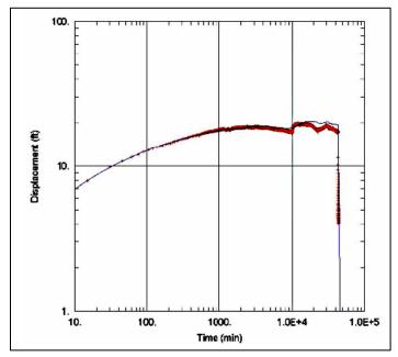
Figure 9. Drawdown response of water levels in monitoring well PBF-10R, located 330 feet away from the ASR well.
