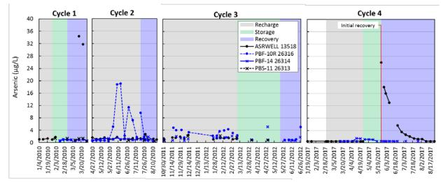
Figure 29. Arsenic concentrations in water from the Hillsboro ASR well and monitoring wells during the four test cycles.
