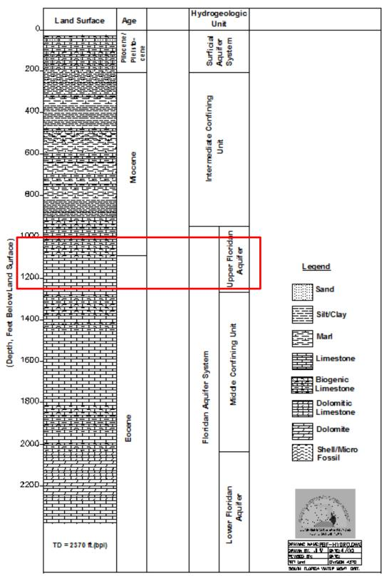
Figure 7. Generalized hydrogeology of the Hillsboro ASR site. (The red box designates the open-hole storage zone portion of the ASR well.)
