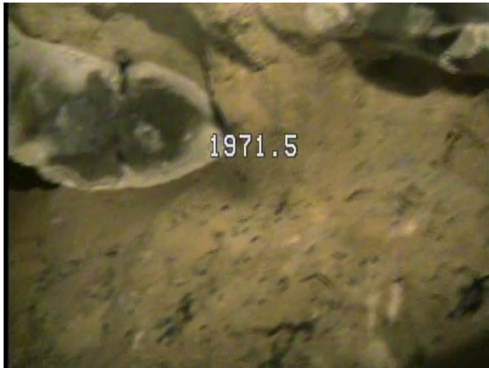
Figure 3-2. BHV view of chert nodules near the top of the Oldsmar Formation at approximately 1,971 ft bls.
