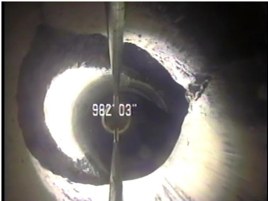
Figure 4-5. BHV view of fractures bounding a cavity in OSF-105 (982 ft bls).
