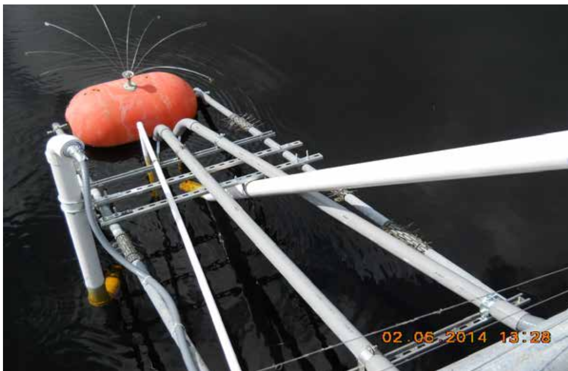
Figure 3. Sampling equipment at G310 mounted on a floating armature.
