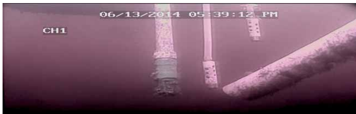
Figure 4. The sampling equipment at G310 including, from left to right, intakes for the RPA, ACF, and ADT. The diagonal, slotted pipe houses in situ probes, including temperature, conductance, and turbidity.
