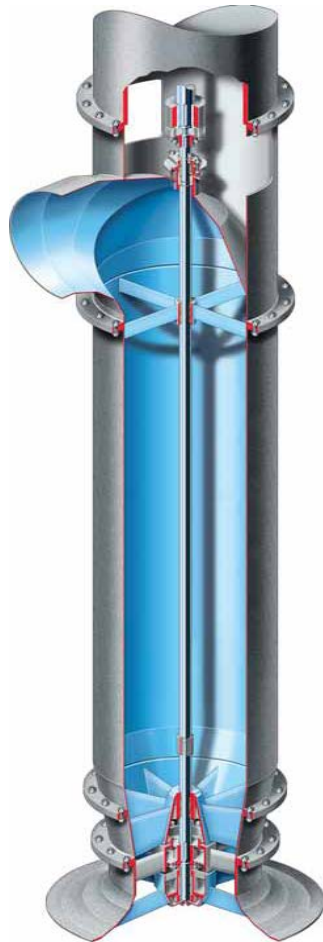
Figure 1b. Conceptual design of a vertical axial-flow pump (courtesy of the FlowServe Corporation)
