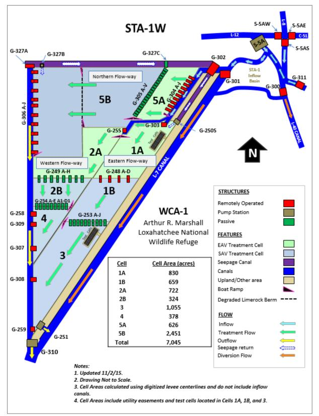
Figure B-2. Stormwater Treatment Area 1 West (STA-1W) schematic showing configurations of the treatment cells, flow direction, dominant vegetation type, and locations of flow structures.
