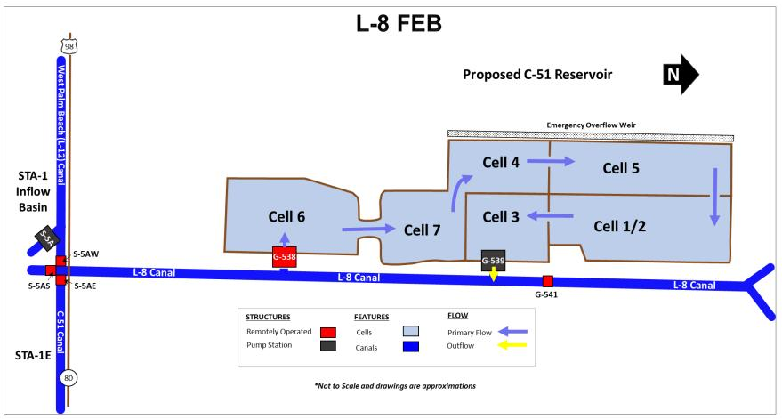
Figure B-6. L-8 Flow Equalization Basin (FEB) schematic showing configurations of cells, flow direction, and locations of flow structures.
