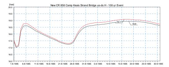
Figure 4.21 Simulated Stage Results for Scenario 1 Upstream (red) and Downstream (black) of the Proposed Bridge on CR-858 at Camp Keais Strand (Location 1) for the 100vear Design Event.
