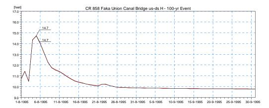
Figure 4.59 Simulated Stage Results for Scenario 3 Upstream (red) and Downstream (black) of the Proposed Modified Bridge on CR-858 at Faka Union Canal (Location 3) for the 100-year Design Event.
