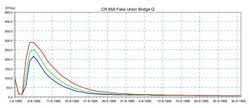
Figure 4.45 Simulated Discharge Results for Scenario 2 at the Proposed Modified Bridge on CR-858 at Faka Union Canal (Location 3) for the 5-year (blue), 25-year (green), and 100-year (red) Design Event.
