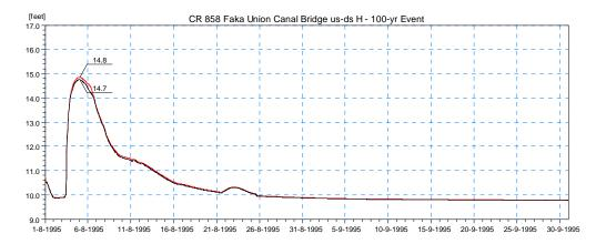
Figure 4.12 Simulated Stage Results for Existing Conditions (Scenario 0) Upstream (red) and Downstream (black) of the Existing Bridge on CR-858 at Faka Union Canal (Location 3) for the 100-year Design Event.
