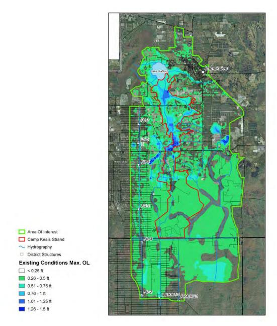
Figure 3.22 Simulated Maximum Overland Water Depths for the Calibrated Model with the 5-day 100-year Design Event.
