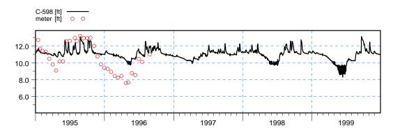
Figure 3.18 Simulated and Observed Results at the Groundwater Observation Well C-598.
