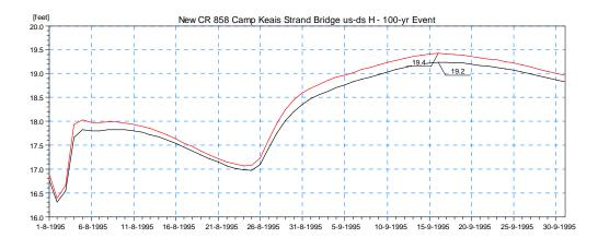
Figure 4.53 Simulated Stage Results for Scenario 3 Upstream (red) and Downstream (black) of the Proposed Bridge on CR-858 at Camp Keais Strand (Location 1) for the 100vear Design Event.
