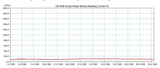
Figure 4.8 Simulated Discharge Results for Existing Conditions (Scenario 0) at the Existing Culvert on CR-858 at Camp Keais Strand (Location 1) for the 5-year (blue), 25year (green), and 100-year (red) Design Event.
