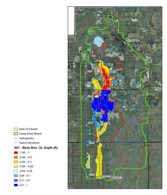
Figure 4.36 Simulated Differences Between Existing Conditions (Scenario 0) and Scenario 1 Maximum Overland Water Depths During the 100-year Design Event.
