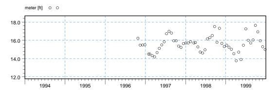
Figure 2.12 Observed Groundwater Levels at C-503 (ft NAVD 1988).
