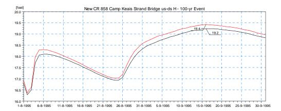
Figure 4.37 Simulated Stage Results for Scenario 2 Upstream (red) and Downstream (black) of the Proposed Bridge on CR-858 at Camp Keais Strand (Location 1) for the 100vear Design Event.
