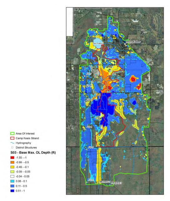
Figure 4.68 Simulated Differences between Existing Conditions (Scenario 0) and Scenario 3 Maximum Overland Water Depths During the 100-year Design Event.
