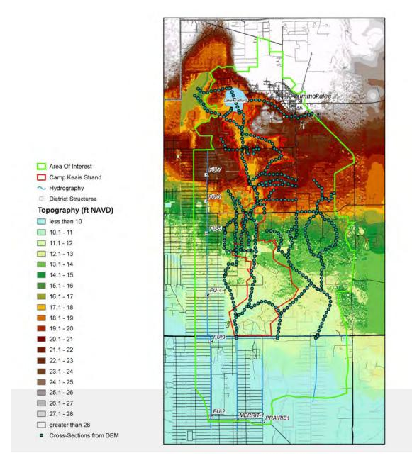
Figure 2.20 Digital elevation model for the Camp Keais Strand Area developed from the best available topographic area for the data (ft NAVD). The locations for cross-sections extracted from the digital elevation model are also shown. The digital elevation model has a maximum horizontal resolution of 100 ft.
