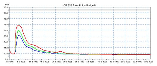
Figure 4.13 Simulated Stage Results for Existing Conditions (Scenario 0) Upstream of the Existing Bridge on CR-858 at Faka Union Canal (Location 3) for the 5-year (blue), 25-year (green), and 100-year (red) Design Event.
