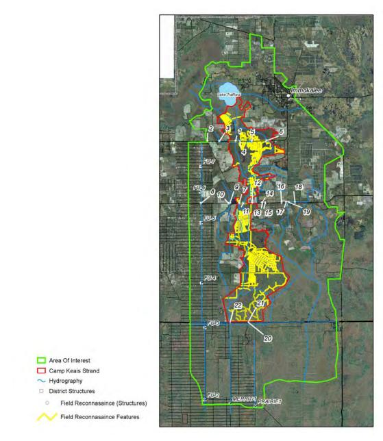
Figure 2.1 Locations of Structures and Flowway Obstructions Observed During Windshield Survey and Aerial Photograph Analysis.
