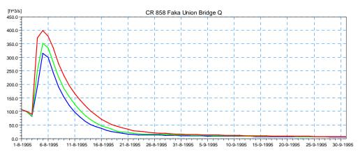
Figure 4.61 Simulated Discharge Results for Scenario 3 at the Proposed Modified Bridge on CR-858 at Faka Union Canal (Location 3) for the 5-year (blue), 25-year (green), and 100-year (red) Design Event.
