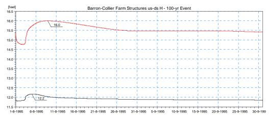
Figure 4.18 Simulated Stage Results for Existing Conditions (Scenario 0) Upstream (red) and Downstream (black) of the Existing Barron-Collier Structures in Camp Keais Strand (Locations 5 and 6) for the 100-year Design Event.
