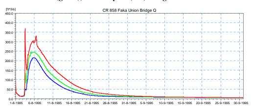
Figure 4.14 Simulated discharge results for existing conditions (Scenario 0) at the existing bridge on CR-858 at Faka Union Canal (location 3) for the 5-year (blue), 25-year (green), and 100-year (red) design event.
