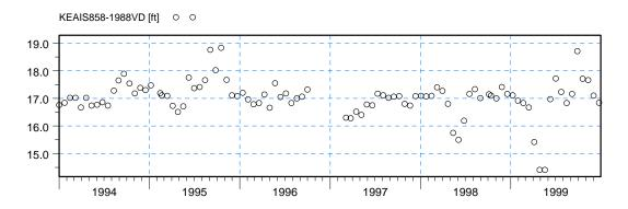
Figure 2.7 Observed Stages at the Headwater Side (North) of the Bridge on Camp Keais Strand at CR 858 (ft NAVD 1988).
