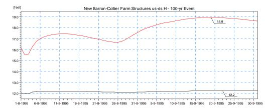
Figure 4.65 Simulated Stage Results for Scenario 3 Upstream (red) and Downstream (black) of the Proposed Modified Barron-Collier Structures in Camp Keais Strand (Locations 5 and 6) for the 100-year Design Event.
