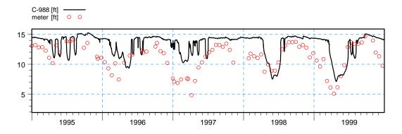
Figure 3.20 Simulated and Observed Results at the Groundwater Observation Well C-988.
