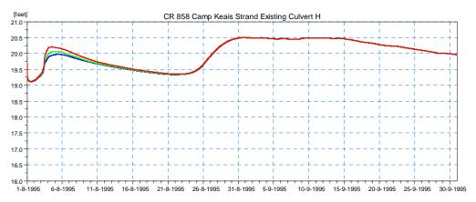
Figure 4.7 Simulated Stage Results for Existing Conditions (Scenario 0) Upstream of the Existing Culvert on CR-858 at Camp Keais Strand (Location 1) for the 5-year (blue), 25-year (green), and 100-year (red) Design Event.
