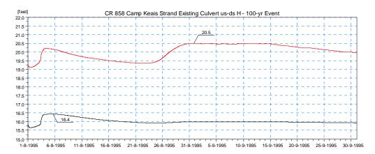
Figure 4.6 Simulated Stage Results for Existing Conditions (Scenario 0) Upstream (red) and Downstream (black) of the Existing Culvert on CR-858 at Camp Keais Strand (Location 1) for the 100-year Design Event.
