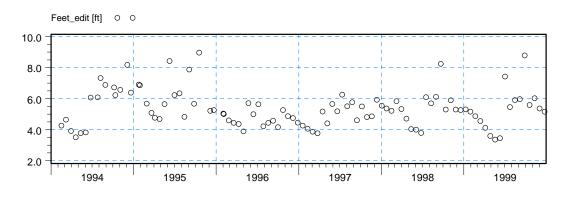
Figure 2.15 Observed Groundwater Levels at C-690 (ft NAVD 1988).
