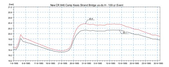
Figure 4.46 Simulated Stage Results for Scenario 2 Upstream (red) and Downstream (black) of the Proposed Modified Bridge on CR-846 at Camp Keais Strand (Location 4) for the 100-year Design Event.
