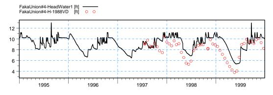
Figure 3.10 Simulated and Observed Results at the Faka Union Canal Number 4 Headwater Gage.
