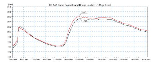
Figure 4.15 Simulated Stage Results for Existing Conditions (Scenario 0) Upstream (red) and Downstream (black) of the Existing Bridge on CR-846 at Camp Keais Strand (Location 4) for the 100-year Design Event.
