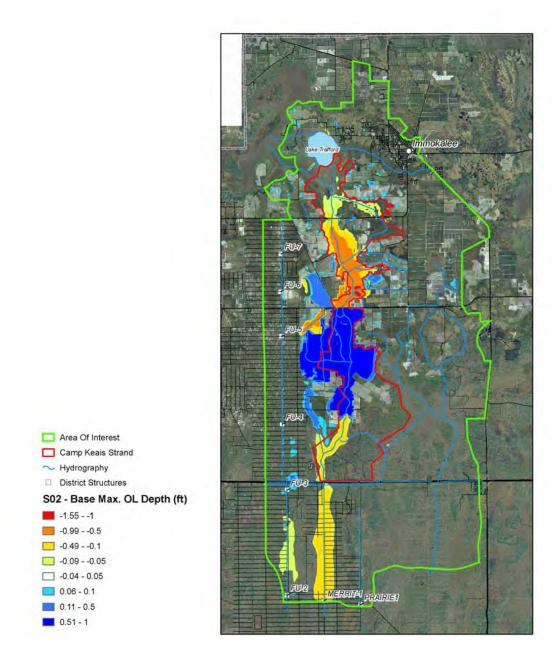
Figure 4.52 Simulated Differences Between Existing Conditions (Scenario 0) and Scenario 2 Maximum Overland Water Depths During the 100-year Design Event.
