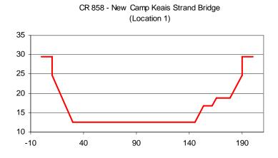
Figure 4.2 Geometry of the New Bridge on CR-858 at Camp Keais Strand (Location 1). View Looking North.
