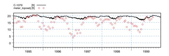
Figure 3.21 Simulated and Observed Results at the Groundwater Observation Well C-1079.
