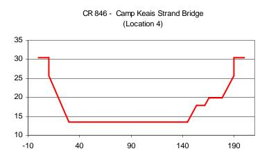
Figure 4.4 Geometry of the New Bridge on CR-846 at Camp Keais Strand (Location 4). View Looking North.
