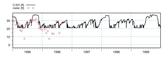
Figure 3.17 Simulated and Observed Results at the Groundwater Observation Well C-531.
