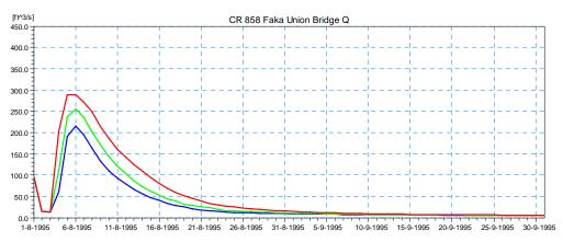
Figure 4.29 Simulated Discharge Results for Scenario 1 at the Proposed Modified Bridge on CR-858 at Faka Union Canal (Location 3) for the 5-year (blue), 25-year (green), and 100-year (red) Design Event.
