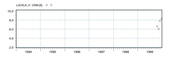
Figure 2.10 Observed Stages at the Headwater Side (North) of Lucky Lake Weir on Merritt Canal (ft NAVD 1988).
