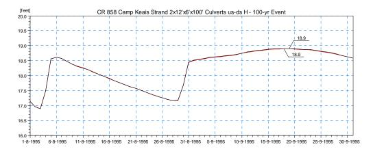
Figure 4.24 Simulated Stage Results for Scenario 1 Upstream (red) and Downstream (black) of the Proposed Culvert on CR-858 at Camp Keais Strand (Location 2) for the 100year Design Event.
