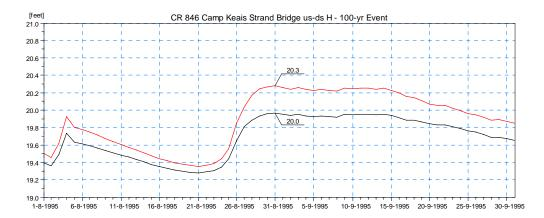
Figure 4.30 Simulated Stage Results for Scenario 1 Upstream (red) and Downstream (black) of the Existing Bridge on CR-846 at Camp Keais Strand (Location 4) for the 100year Design Event.
