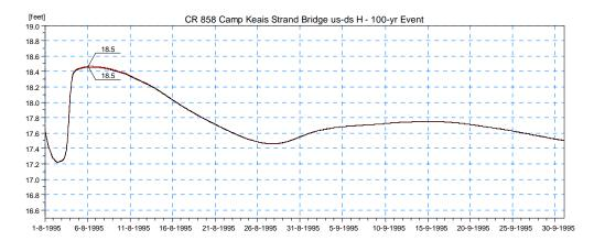
Figure 4.9 Simulated Stage Results for Existing Conditions (Scenario 0) Upstream (red) and Downstream (black) of the Existing Bridge on CR-858 at Camp Keais Strand (Location 2) for the 100-year Design Event.
