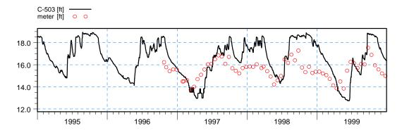
Figure 3.16 Simulated and Observed Results at the Groundwater Observation Well C-503.
