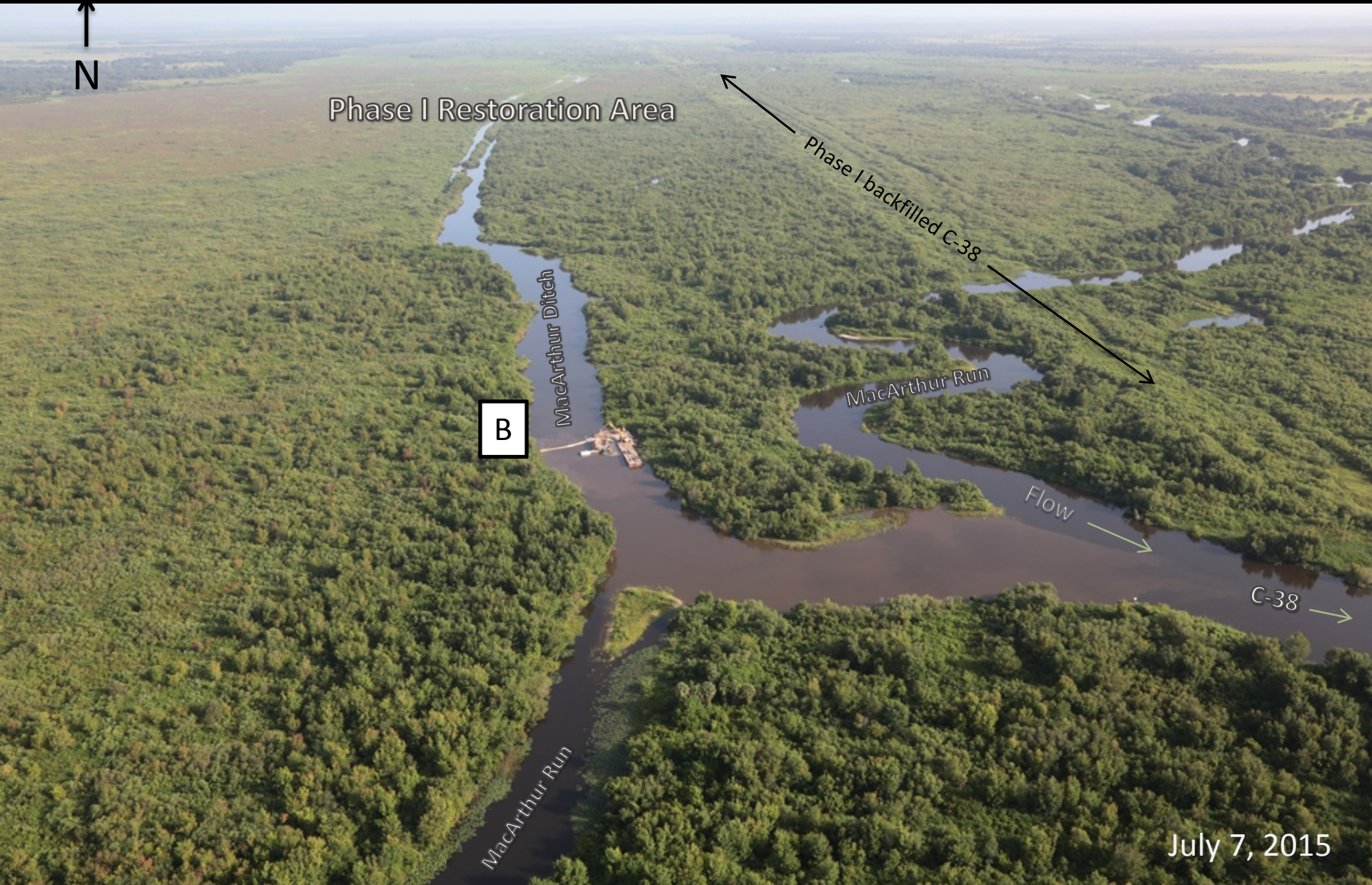
Looking north up the MacArthur Ditch, contractors are in the process of completing a plug across the ditch at location B. Once the plug is complete, they will continue to backfill to the north the entire length of the ditch.
