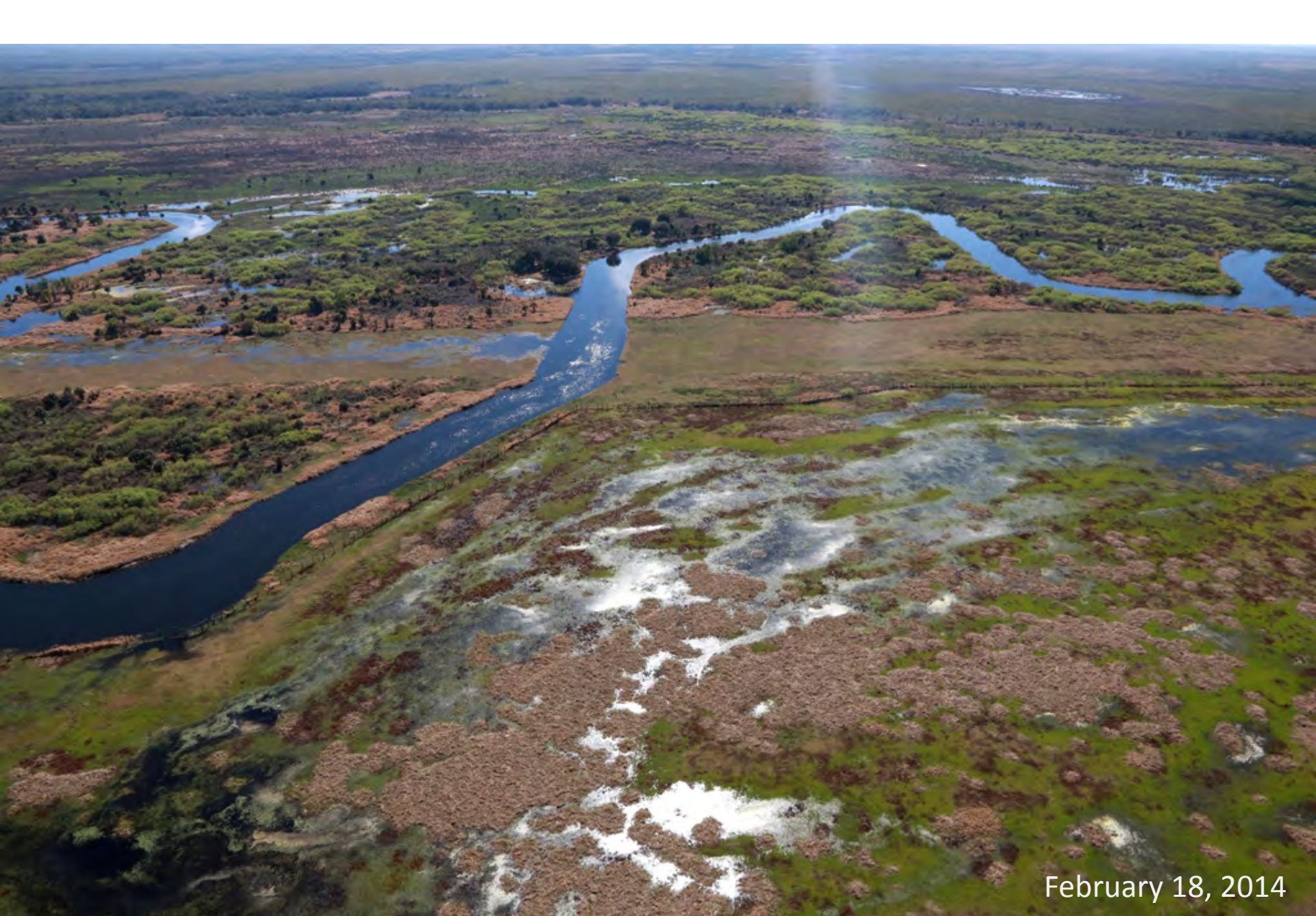
North end of Kissimmee River Phase IVB restoration area in Avon Park. The backfilled C-38 canal can be seen extending across the center of the photo.
