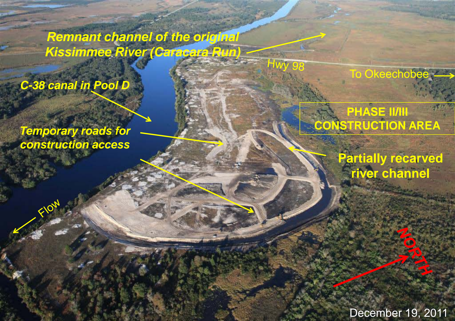
Contract 10A (Reach 3 north) river channel re carve construction. Image from December 2011
