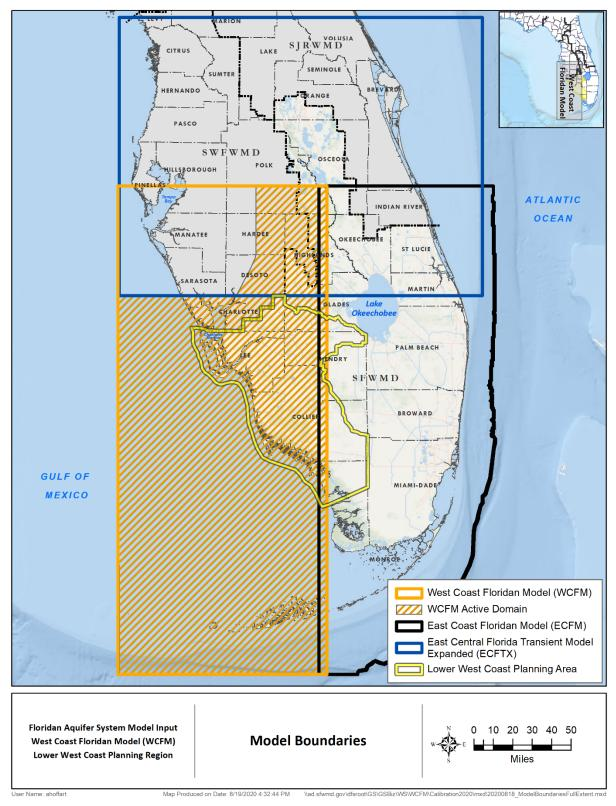
Figure 2. Model boundaries of three regional groundwater models in Central and South Florida.
