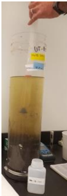
Figure 7. Sampling technique using a Coliwasa tube sampler to collect water samples from core tubes.
