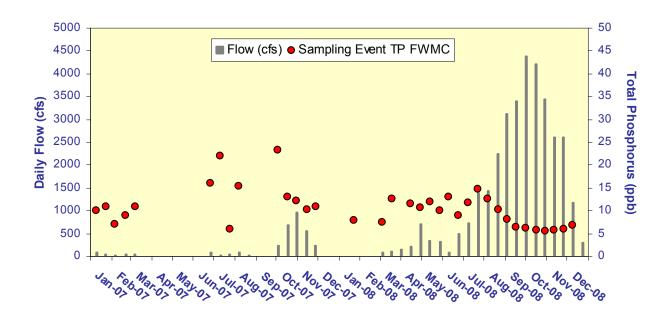
**Figure 8.** The relationship between daily flow at Shark River Slough structures and the corresponding flow-weighted mean TP concentrations for individual sampling events.
