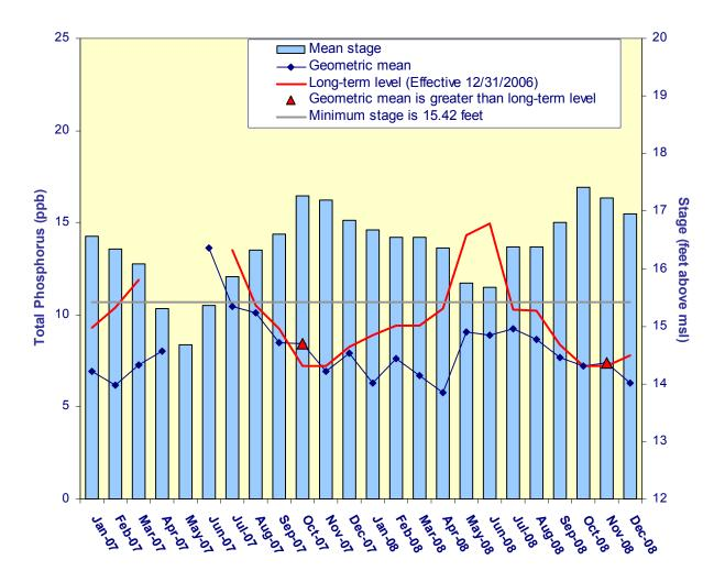
Figure 2. Monthly TP geometric mean concentrations for the Arthur R. Marshall Loxahatchee National Wildlife Refuge compared to the long-term levels. The calculated long-term levels are adjusted for fluctuations in stage. The long-term levels were not applicable for April 2007 through June 2007 because the average stage was less than 15.42 feet. The geometric mean was greater than the long-term level in October 2007 and in November 2008.
