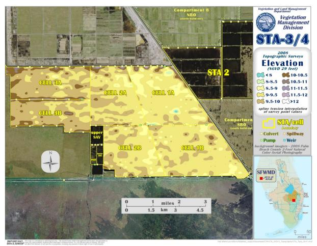
Figure 9. STA-3/4 DEM based on 2008 Topographic Survey Data
