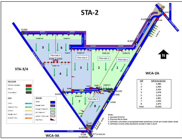
Figure 3. STA-2 Schematic
