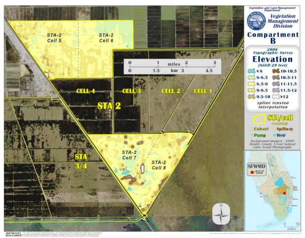
Figure 12. Compartment B\* DEM based on 2006 Topographic Survey Data (\*The Compartment B treatment cells are now referred to as STA-2 Cells 5, 6, 7 and 8).
