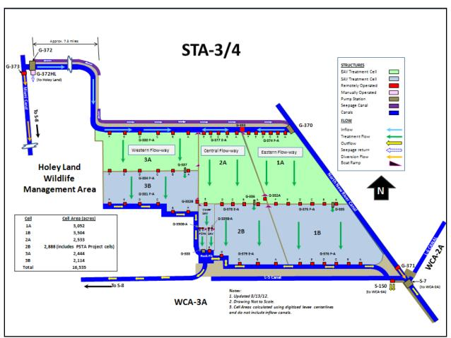
Figure 4. STA-3/4 Schematic
