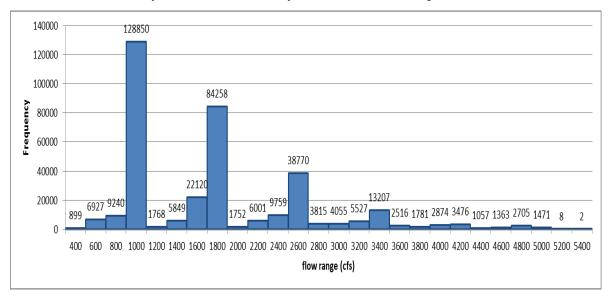
Figure 5-1. S-5A breakpoint flow data for the STA-1 Inflow Basin Canal study.
