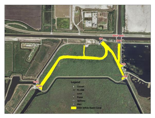
Figure 3-1. STA-1 Inflow Basin Canal and the associated structures
