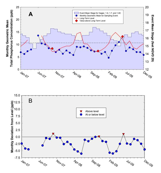
**Figure 3. (A)** Monthly total phosphorus geometric mean concentrations for the Arthur R. Marshall Loxahatchee National Wildlife Refuge compared to calculated long-term levels. These calculated long-term total phosphorus levels are adjusted for fluctuations in stage. The long-term levels were not applicable for April 2007 through June 2007 because the average stage was less than 15.42 feet. The geometric mean was greater than the long-term level in October 2007, November 2008, and June 2009.
