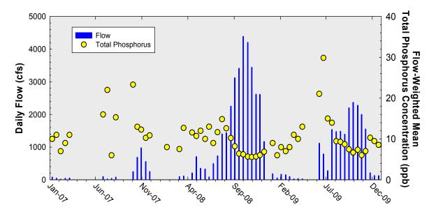
**Figure 10.** Total daily flow at Shark River Slough structures and the corresponding flow-weighted mean total phosphorus concentrations for individual sampling events.
