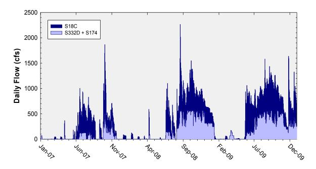
**Figure 13.** Daily flows into Everglades National Park as a stacked sum of Taylor Slough (structures S332D + S174) and Coastal Basins (structure S18C). Structure S174 was plugged in September 2007 and is no longer used.
