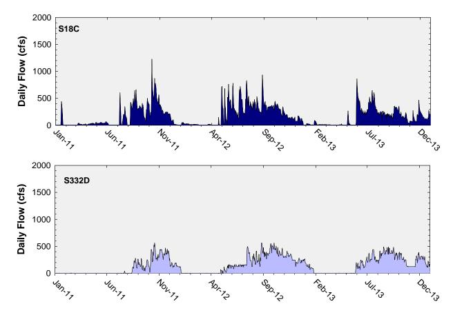
**Figure 8.** Daily flows at individual Coastal Basins (S18C) and Taylor Slough (S332D) structures into the ENP.
