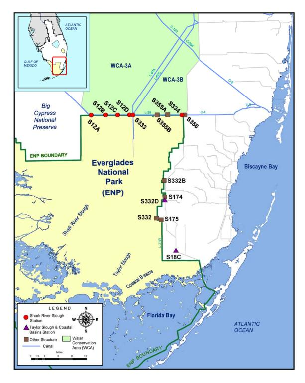
**Figure 4.** ENP flow structures.
