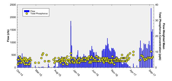
**Figure 10.** Flow from Taylor Slough and Coastal Basins structures (S332D and S18C) on the days of sampling, and the corresponding flow-weighted mean TP concentrations for individual sampling events (Method 1).
