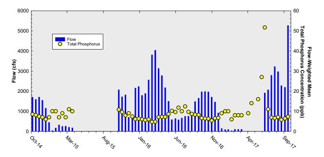
**Figure 11.** Flow at Shark River Slough structures on the day of sampling and the corresponding TP FWMCs for individual sampling events using Method 1. There were no sampling event values from April to September 2015 because there was no flow during sampling events in this period.
