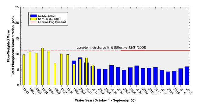
**Figure 5.** The 12-month TP FWMCs in inflows to ENP through Taylor Slough and Coastal Basins at the end of each water year compared to the 11 ppb long-term TP limit. Blue bars show S332D, S174, and S18C for WY 1999 through WY 2007, and S332D and S18C (Method 1) from WY 2008 to WY 2017.
