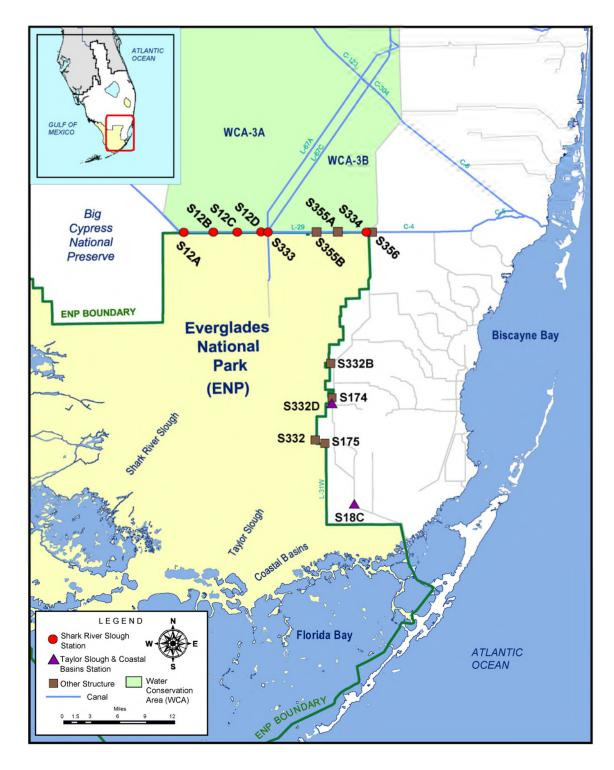
Figure 4. ENP flow structures.
