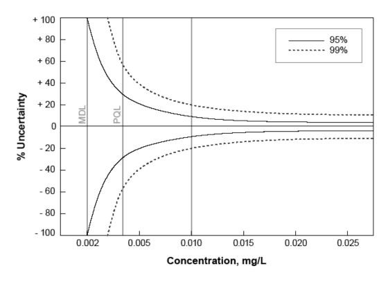
Figure 8. Uncertainty of TP measurement close to the detection limit.
