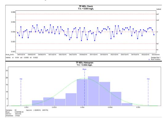
**Figure 4.** TP QC (Method Detection Limit Check, 0.004 mg/L) sample recoveries and histogram.
