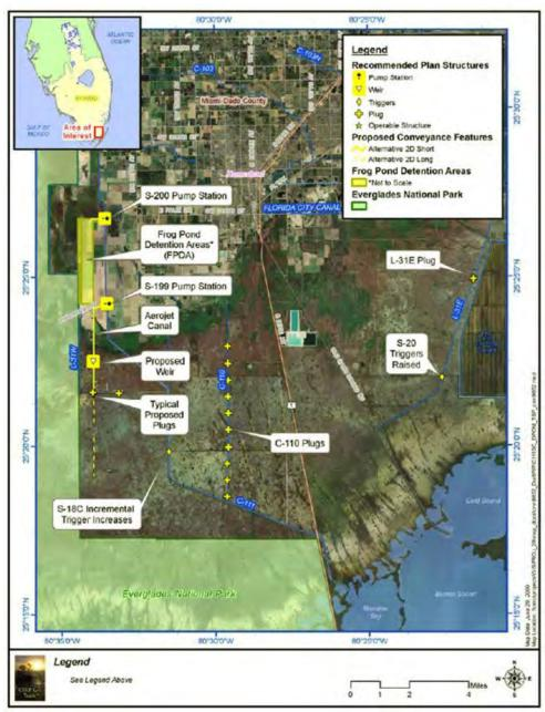
Figure A-5A: C-111 Spreader Canal Western Project Features
