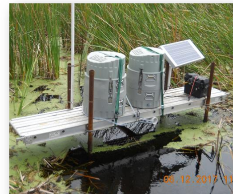
Monitoring platform at interior location in STA-2
