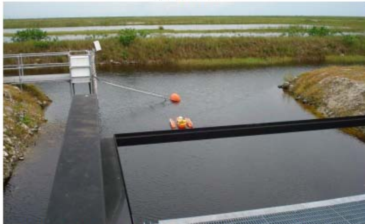
Figure 4. Showing channel cross-section where flow was measured.
