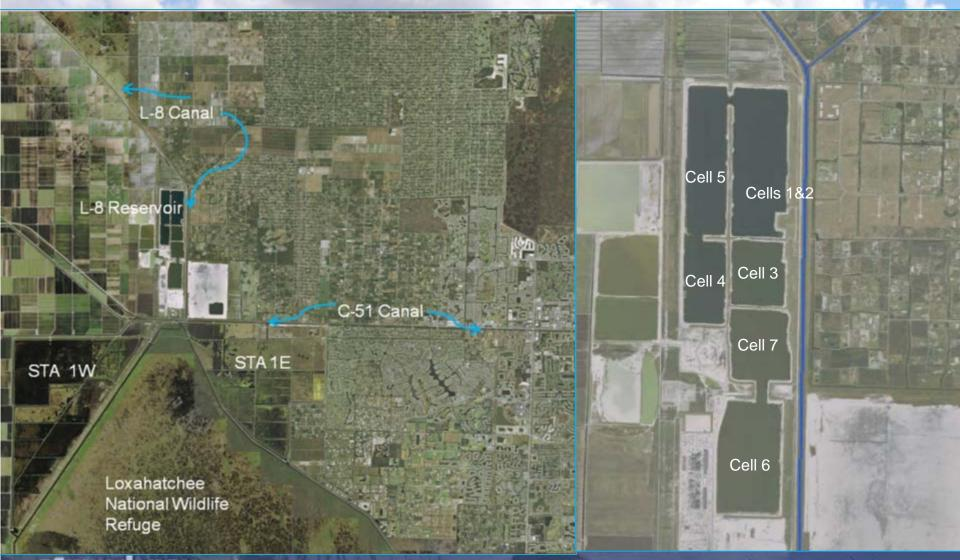
Cells 1/2,4,5: -26.9' NAVD Cell 3: -37.0' NAVD Cell 6,7: -28.3' NAVD L-8 Canal: +12.0' NAVD
