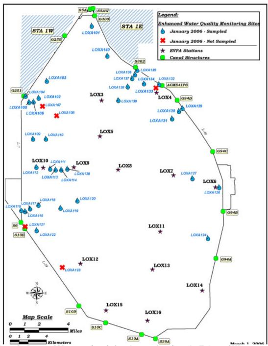
Figure 2. January 2006 map of total phosphorus values from the Enhanced Water Quality Monitoring and the EVPA stations in the A.R.M. Loxahatchee National Wildlife Refuge. A primary reason that a station is not sampled is that it has less than 10 cm of clear water column representative of that area.
