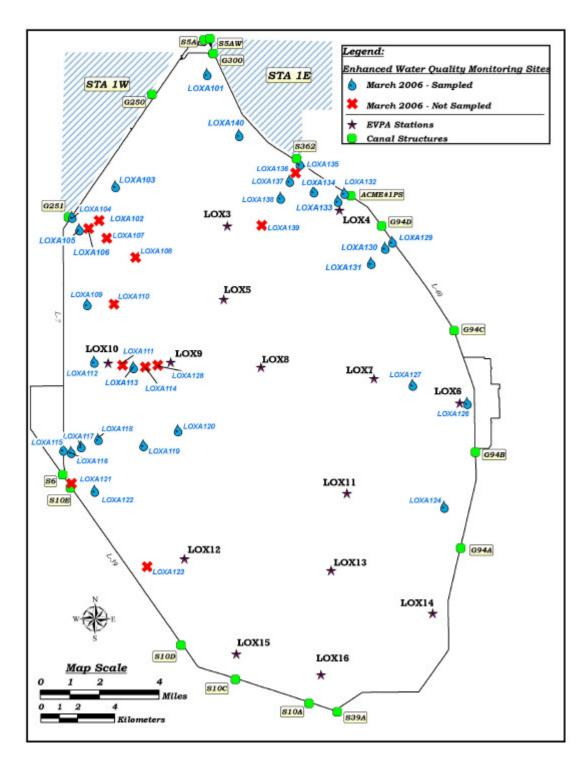
Figure 4. March 2006 map of total phosphorus values from the Enhanced Water Quality Monitoring and the EVPA stations in the A.R.M. Loxahatchee National Wildlife Refuge. A primary reason that a station is not sampled is that it has less than 10 cm of clear water column representative of that area.
