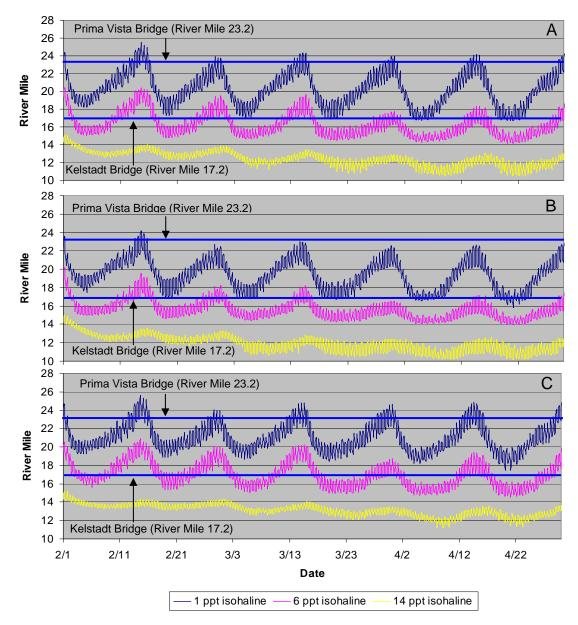
**Figure 7.3.** Locations of 1 psu, 6 psu, and 14 psu isohalines during the 30-day simulation for (A) 130 cfs mean monthly, V=4,000 acre-feet, Qp=400 cfs, Tp=3 day; (B) 170 cfs mean monthly, V=5,000 acre-feet, Qp=400 cfs, Tp=3 day; (C) 100 cfs mean monthly V=3,000 acre-feet, Qp=250 cfs, Tp=3 day.
