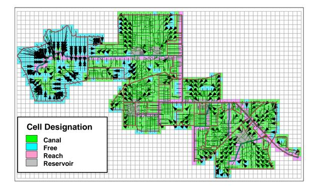
**Figure C2-2.** The C-24 Model Grid showing cell designation. The green lines represent the hydrography coverage. The red lines represent the sub-basin delineation.
