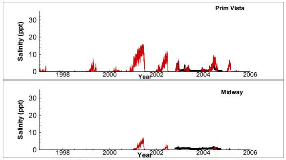
**Figure 12.** Modeled salinity (red) at Prim Vista Bridge and Midway Bridge compared with observation (black) from 1997 to 2005
