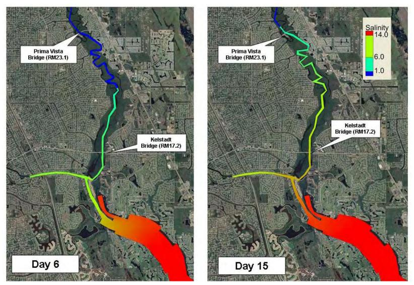
Figure 7.4c. Simulated salinity results for Day 6 and Day 15 using pulse A release flows to the North Fork of the St. Lucie River.
