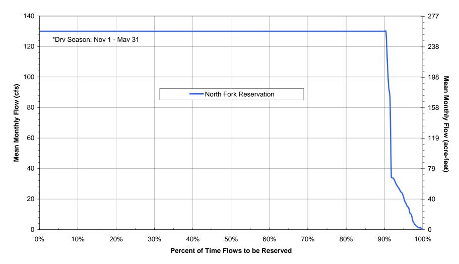
Figure 9.1. Volume probability curve of surface water deliveries into the North Fork at the Gordy Road Structure to be reserved for the dry season.
