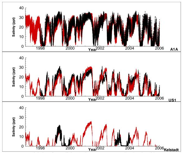
**Figure 10.** Modeled surface salinity (red) at A1A, US1 and Kelstadt Bridge compared with observation (black) from 1997 to 2005
