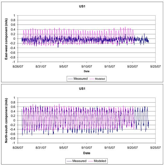
Figure 8. Modeled velocity (red) compared with measured at US1 Bridge in August-September, 1997
