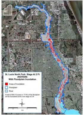
Along with the DEM analysis, the stage data of the river was analyzed to determine the stages of the river and duration for the period of record. The river stages have been monitored at three locations. Traveling upstream, the sites are Veteran's Park just north of the Kelstadt Bridge, Prima Vista Bridge, and Midway Bridge.
