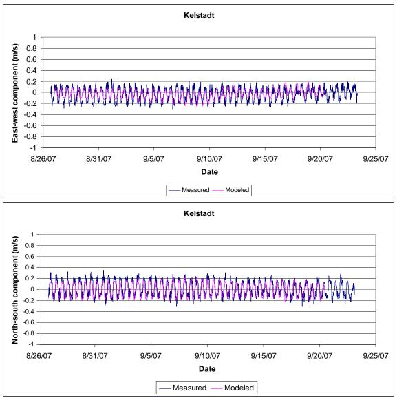
Figure 9. Modeled velocity (red) compared with measured at Kelstadt Bridge in August-September, 1997
