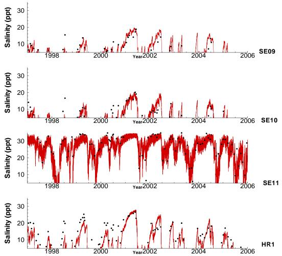
Figure 15. Modeled salinity (red) at SE09 through SE11 and HR1 compared with observation (black dot) from 1997 to 2005
