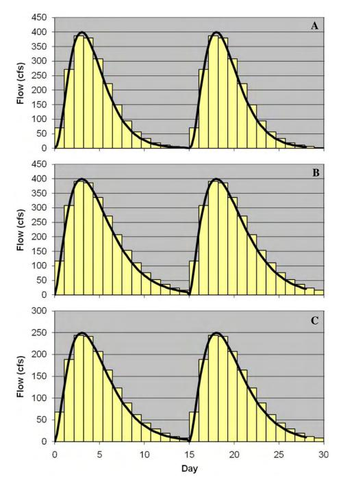
**Figure 7.2.** Hydrograph for the pulse release at the Gordy Road Structure simulated with CH3D: (A) 130 cfs mean monthly assuming two releases made over a 30-day period, V=4,000 acre-feet, Qp=400 cfs, Tp=3 day; (B) 170 cfs mean monthly assuming two releases made over a 30-day period, V=5,000 acre-feet, Qp=400 cfs, Tp=3 day; (C) 100 cfs mean monthly assuming two releases made over a 30-day period, V=250 cfs, Tp=3 day.
