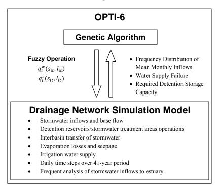
**Figure 5.2.** Interaction of the genetic algorithm in OPTI6 for optimizing fuzzy operating rules with drainage network simulation model (Wan et al. 2006).
