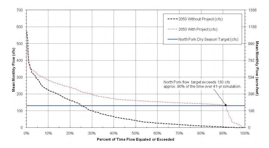
**Figure 8.2.** Volume probability curve for surface water deliveries into the North Fork at Gordy Road for 2050 Future with Project Condition, Future without Project Condition, and North Fork flow target for the 41-year period of record (1965–2005).
