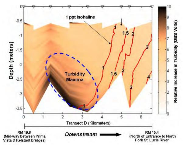
**Figure 6.4.** Example of the relationship between the estuarine turbidity maximum and the location of the 1 psu isohaline within the North Fork of the St. Lucie River on April 3, 2008 (Fugate and Andreson 2008).
