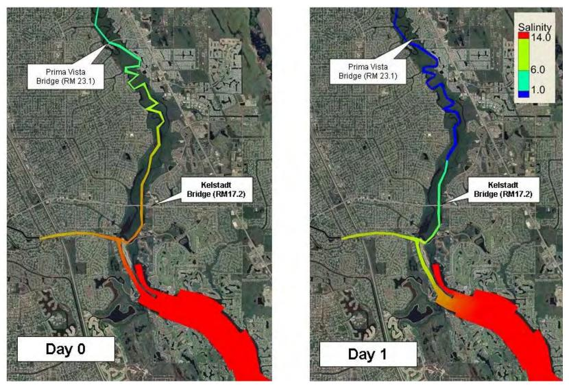
Figure 7.4a. Simulated salinity results for Day 0 and Day 1 using pulse A release flows to the North Fork of the St. Lucie River.
