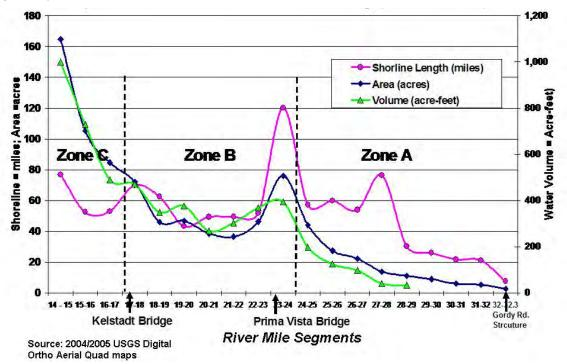
**Figure 6.2.** Calculations of shoreline length, area, and volume for the North Fork of the St. Lucie River based on GIS analysis of 2004/2005 USGS Digital Ortho Quad Maps and bathymetric data.
