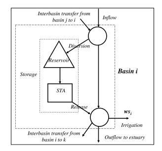
Figure C3-2. Schematic of typical off-stream reservoir with connected storm-water treatment area (Wan et al., 2006).
