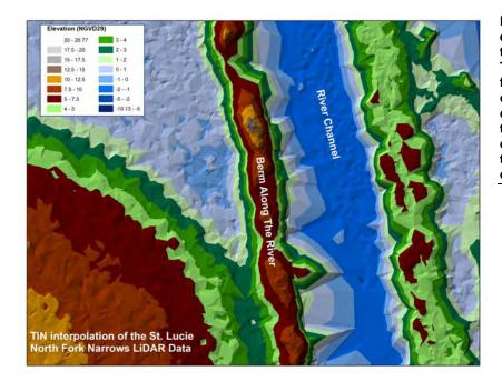
Figure 2. This is an example of a TIN. Note the irregular triangles. This TIN was created from the LiDAR data only. The bathymetry data was not included in the interpolation. One can clearly see the berm to the left of the river channel.
