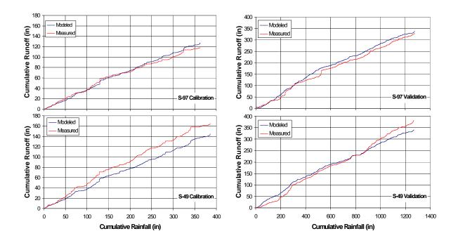
Figure C2-4. Double mass curve during the calibration period (1994–2000) and validation period (1965-1993) at S-97 and S-49 Stations.
