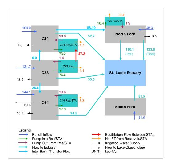
Figure C-3. Annual water budget of OPTI6 simulation results for the period from 1965 to 2005.
