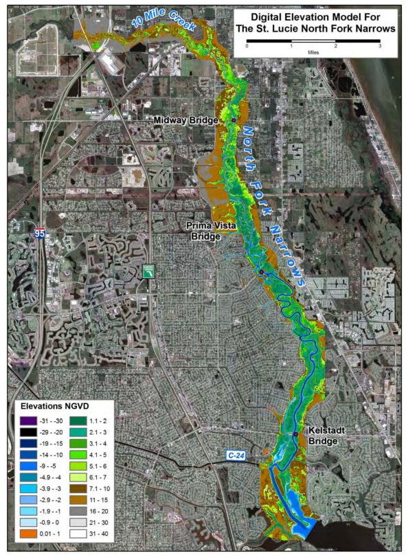
Figure 7. The final digital elevation model for the North Fork Narrows
