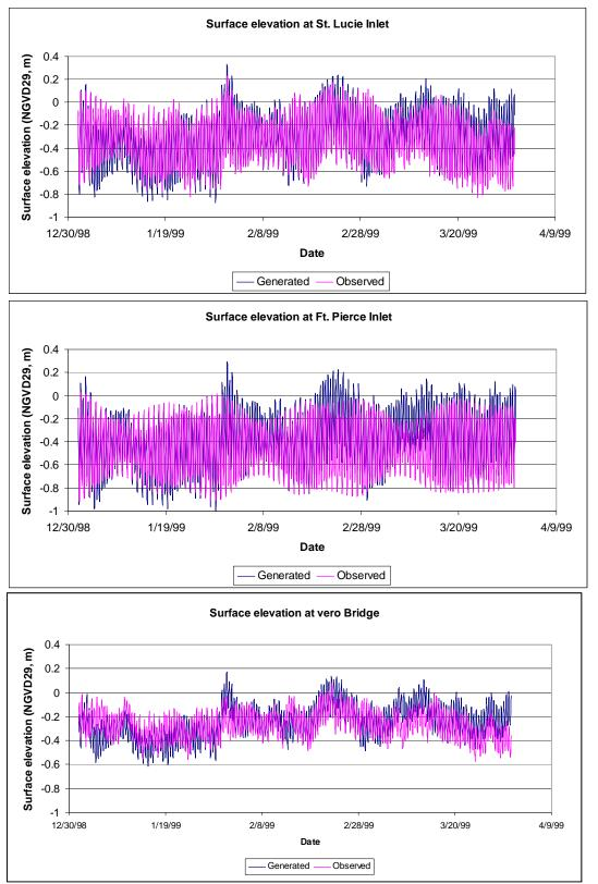
**Figure 3.** Surface elevation generated by the combination of harmonic tide and low frequency motion compared with observation at three ocean boundary locations: St. Lucie Inlet, Ft. Pierce Inlet and Vero Bridge.
