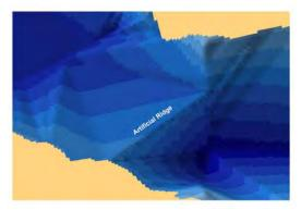
Figure 3. The initial TIN of the bathymetry created this artificial ridge in the river's bed where there was a lack of bathymetry data
