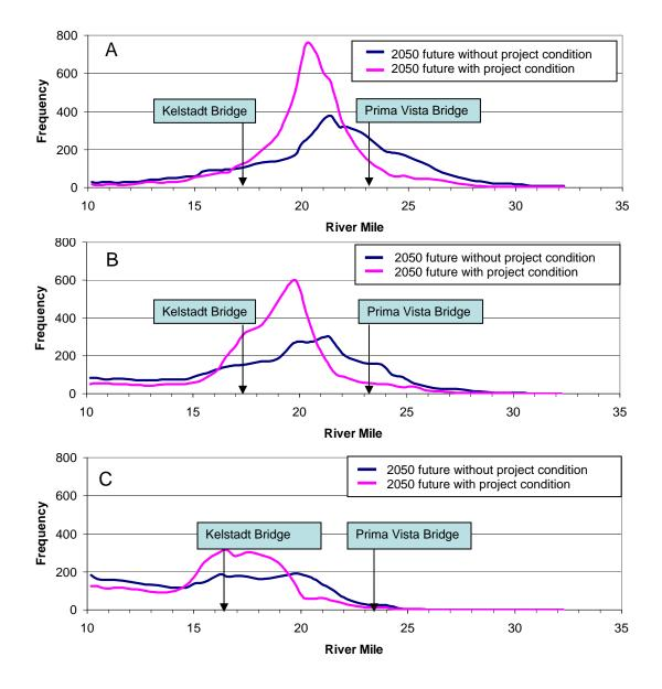
**Figure 7.8.** Frequency of occurrence of (A) 1 psu, (B) 6 psu, and (C) 14 psu isohalines in the North Fork under the 2050 Future with and without Project Conditions as determined using the CH3D hydrodynamic model.
