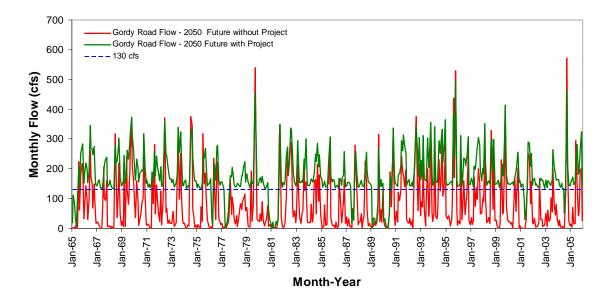
**Figure 7.7.** Ten Mile Creek flow comparison between 2050 Future with and without Project Conditions as simulated with WaSh and OPTI-6. Note these were modeled with a constant mean monthly 130 cfs flow and not as a pulsed flow.
