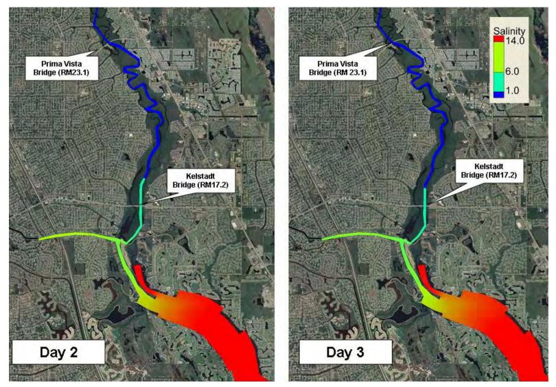
Figure 7.4b. Simulated salinity results for Day 2 and Day 3 using pulse A release flows to the North Fork of the St. Lucie River.
