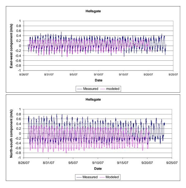
Figure 7. Modeled velocity (red) compared with measured at Hellsgate in August-September, 1997
