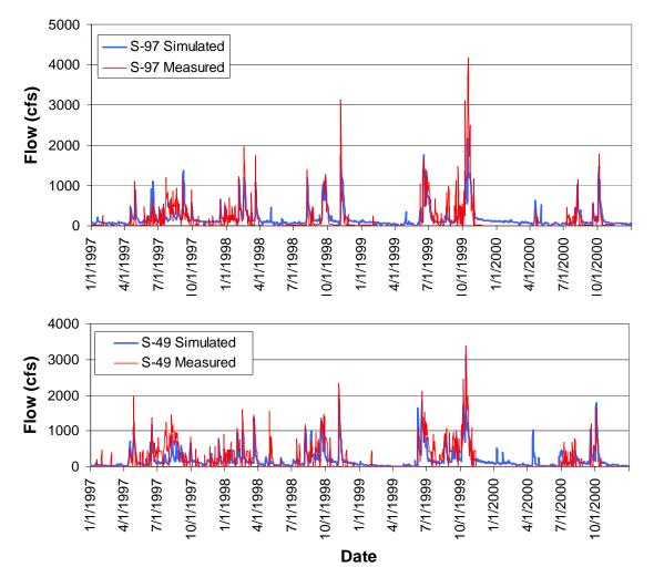
Figure C2-6. Comparisons between simulated and measured daily flow time series for the period from 1997 through 2000 at S-97 and S-49 Stations.
