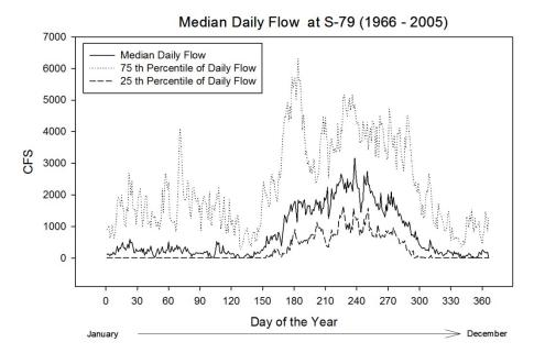
**Figure 3-3.** Median daily discharge (cfs) at the S-79 Structure for 1966 through 2005. Also shown are the 25th and 75th percentiles.
