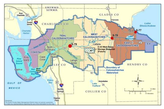
Figure 3-1. Caloosahatchee River, C-43 Canal, and watershed showing major basins, water management structures, and location of the C-43 Reservoir.
