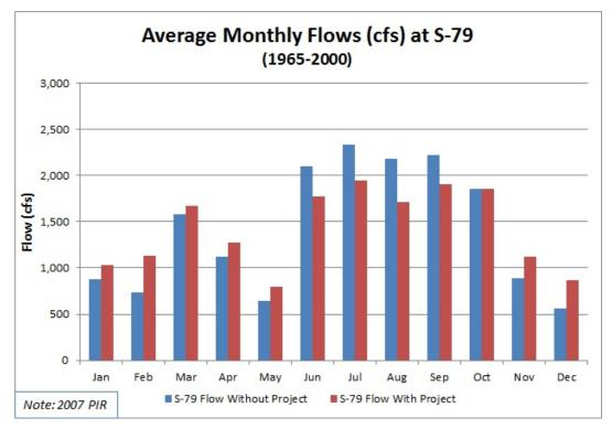
**Figure 3-11.** Average monthly flows (cfs) at the S-79 Structure with and without the C-43 Reservoir based on the WSE and a 36-year period of record (1965 through 2000).
