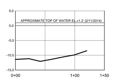
SURVEY BASELINE 'D' PROFILE (Intended Horizontal Display Scale: 1"=50') (Intended Vertical Display Scale: 1"=5")
